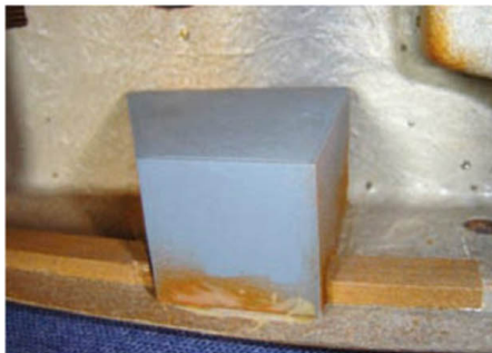
One of the internal companionway boxes glued in place. Note other strip wood pieces, which were fitted earlier to remove distortion of the moulding edge
