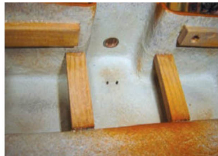
Looking inside the main superstructure. These are some of the braces which had to be fitted and glued to remove the distortion in the moulding
