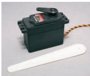
The Hitec 765HB arm winch
