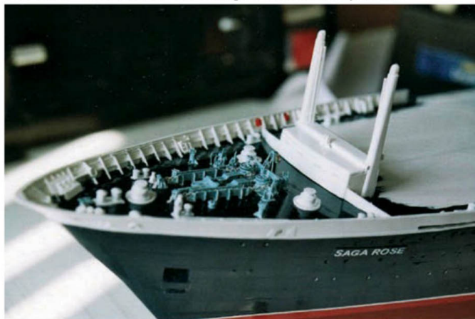
The fully fitted forequarter with its bollards, cable capstans, anchor winches and anchor chains
