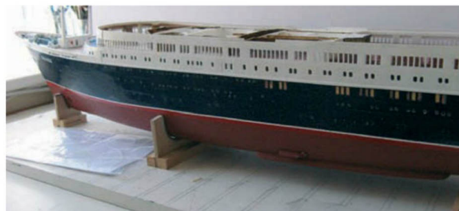
View of the port side, showing the installed superstructure side panels from the weather deck to the promenade deck
