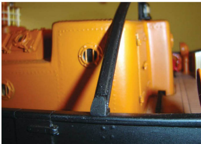
This shows how accurately you must place the large tow beam brackets to align exactly with the rear edge of the superstructure
