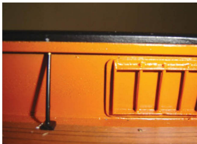
Here is a view of the brass square section tubing running under handrail, which was used to remove the bulwark distortion
