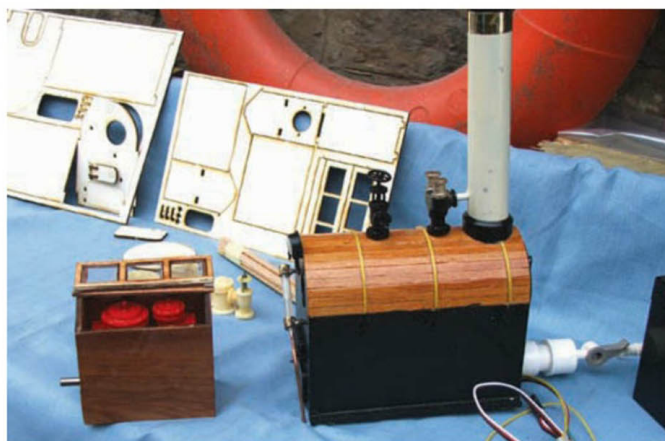
Completed painted dummy engine and boiler with pressure valve and funnel
