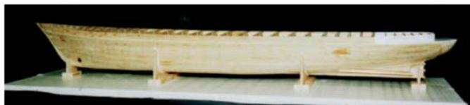
All the planking with 6 mm x 1.5 mm tulipwood strips has been completed
