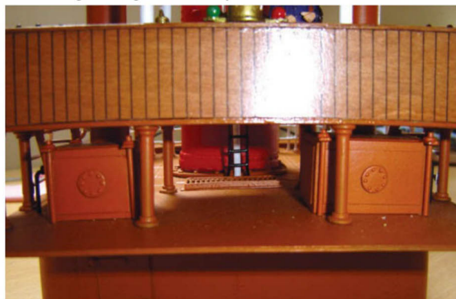
Bridge mounted on its deck with water tanks fixed. Note camber. The front stanchions should just touch the boat deck when fitted correctly
