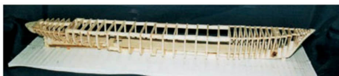
The completed wooden framework for the hull before planking
