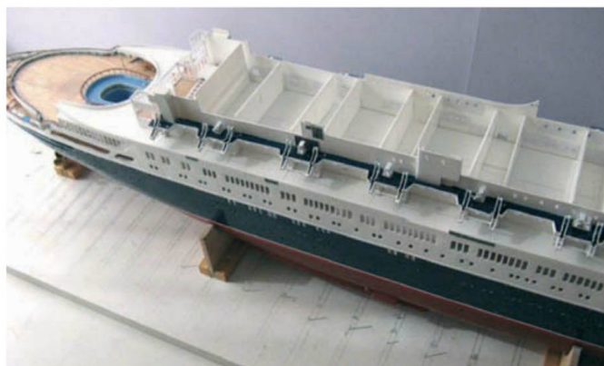
View from the starboard side, of the newly installed davits and boatdecks on the promenade deck
