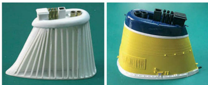
Stages in the construction of the funnel
