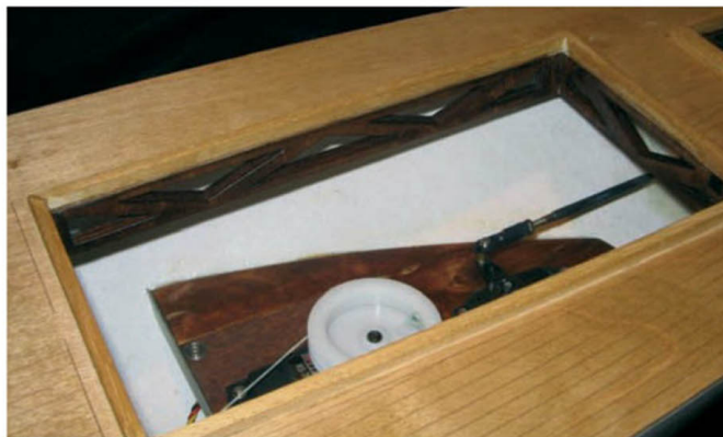
The deck around the hatch covers is supported by CNC cut timber beams as you can see here, supplied as part of the timber pack, alongside such obvious things as the stand!
