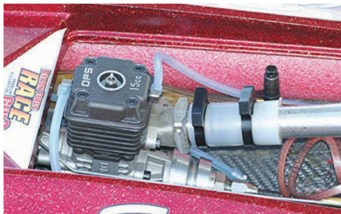
This boat's power plant features a rearward-facing exhaust port, so mounting its tuned pipe didn't require a curved header pipe and the two components were coupled with a thick-wall, high-temperature silicone hose
