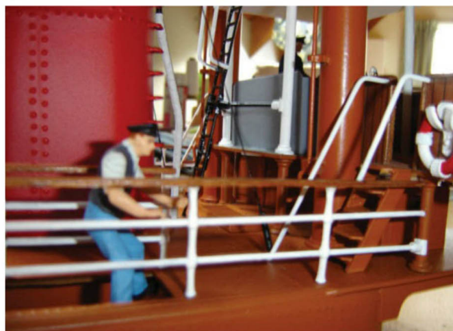
This shows starboard side bridge steps and rails. Note lagged whistle pipe and searchlight ladder braces. Note deck handrails terminating at bridge stanchion per text
