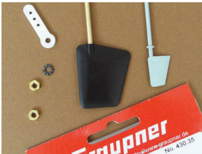
This Graupner rudder is suitable and weighs just 10 g
