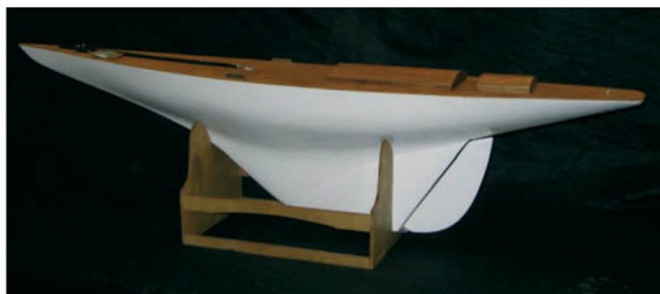
The full keel and rudder is key to the boat's ability to glide through weed – the rudder heel is held by a small metal fitting and a carefully built up tube and O-ring to ensure water tightness inside the hull
