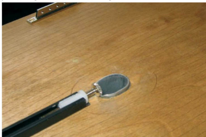
The mast steps in a tube to the hull centreline, and a simple ram gives some rake adjustment
