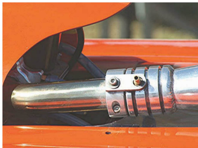
As a backup to the pipe's clamp set-up, this hull's coupler's been drilled/tapped to accept a screw that will in turn hold a small tab and this stay's other opening fits over the coupler's water nipple to create a safety tab should the coupler loosen unexpectedly
