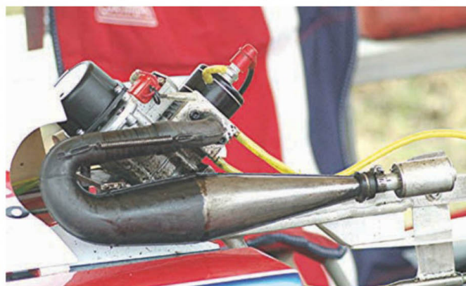
Not unlike an older motocross exhaust, this unique petrol boat's 'outboard' engine arrangement has a steel tuned pipe that features an adjustable header section held in place by two heavy-duty retaining springs
