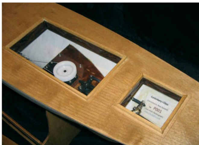
Another view of the winch in place, a single Hitec 785BB, both inexpensive and readily available
