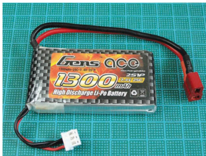
The 1300 mAh 2-cell LiPo battery pack with Deans style connector and 3-pin charge lead
