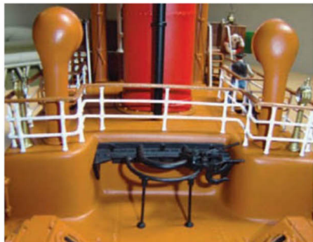
Finished tow hook bolted in its recess. Also, note deck stanchion placements at corners
