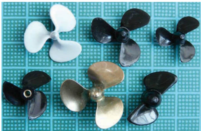
The supplied grey plastic propellers are too weak to use for model propulsion
