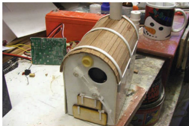
Unpainted boiler showing fire door and water gauge
