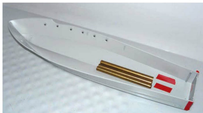
Test tank measurements indicated the all up weight should be in the range of 0.85 to 1 kg
