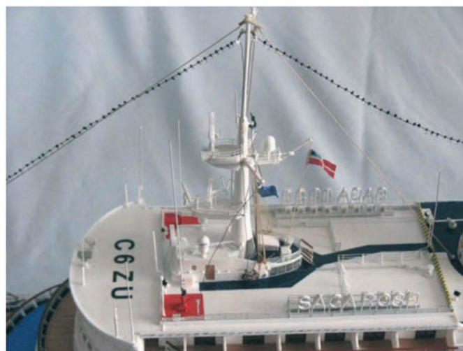
View of the topmost deck showing the mainmast and deckhouse, the illuminated SAGA signs, radio aerials radar scanners and the ship's identification number
