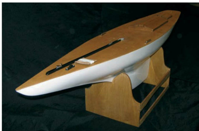
The timber stand is supplied as part of the CNC cut timber items, and is clearly intended to provide good support during building and sailing
