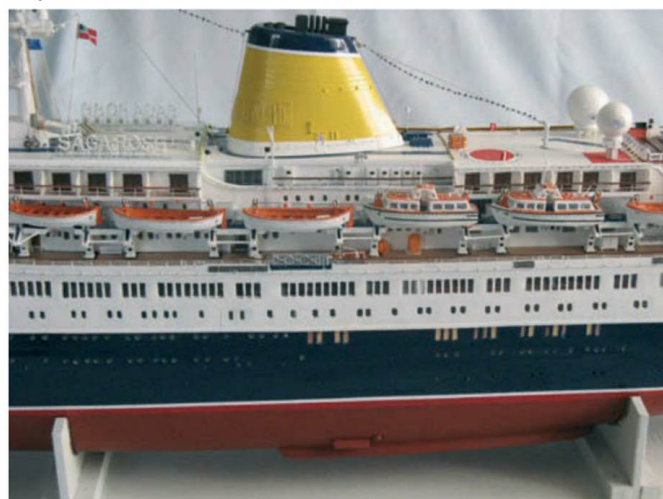
Close-up of the port side showing the funnel, tenders and lifeboats installed
