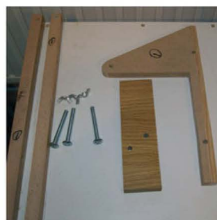
The component parts for one side of the bench – the parallel battens fixed to the bench on the left, the short horizontal support in the middle, and the 30 degree/perpendicular support on the right
