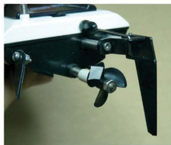
Reflective tape applied to measure the speed of the 20 mm propeller on a Joysway Magic Vee
