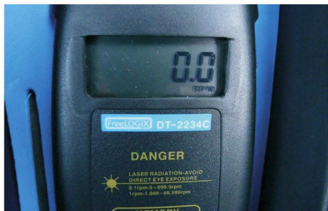
The tachometer displays the rpm on a 5 digit LCD display
