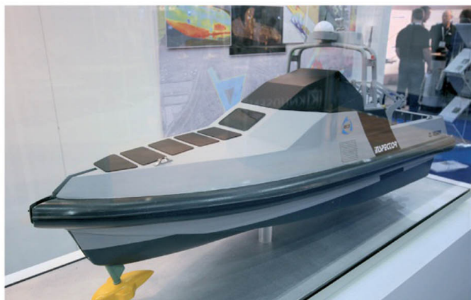
A model of the USV Inspector designed for remote controlled shallow and very shallow water operations
