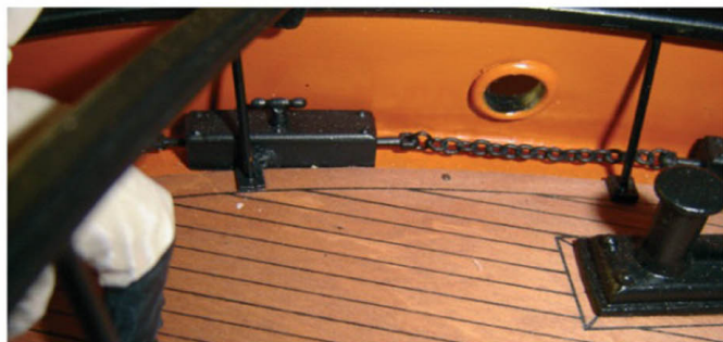
Stern deck portside again showing steering chain spring boxes. Two each, port and starboard
