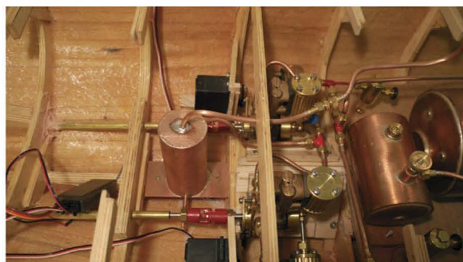
First soldering of outlet pipe using soft solder – what a mess!
