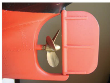
This shows the finished curve at the bottom of the skeg after filling and shaping
