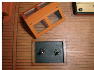
Control mini toggle switches housed under aft skylight. Left-hand is sound generator, right-hand is Rx
