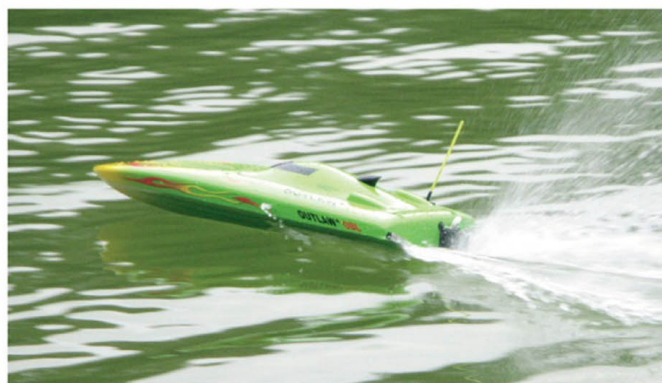
A little tweak with the trim tabs and the boat is running a little looser. If you look at the stern you can see how much water is running off the trim tab – this has quite an effect on the attitude of the hull. Note also the water-cooling out flow
