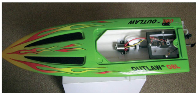
Internal layout. Note the shaft support and the tiny motor!
