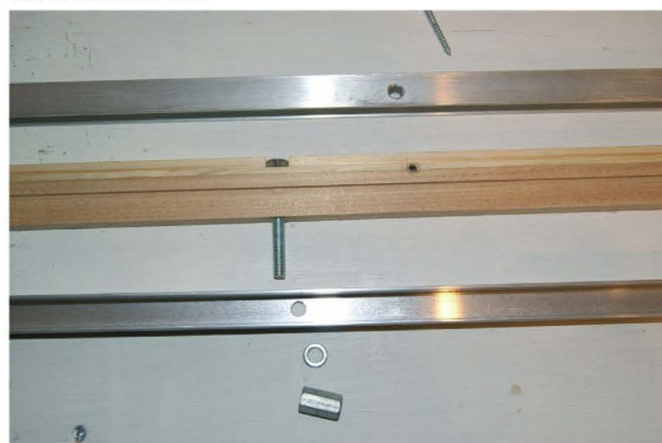
The component parts, with the bolted head fixed in a cut-out in the insert
