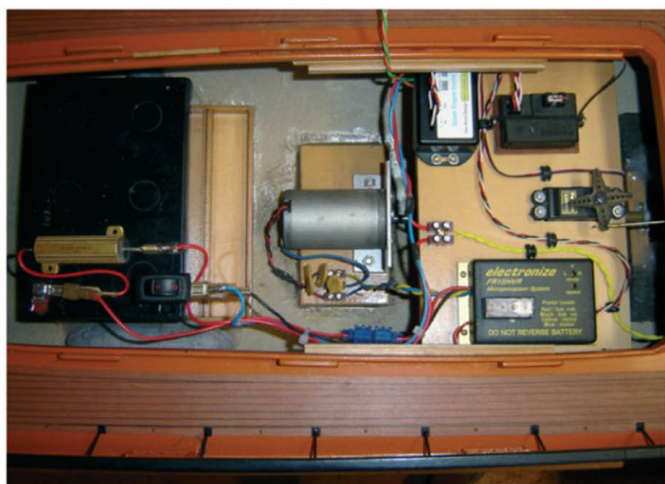
The radio control layout. The Technobots sound generator is at the top next to the Rx. Note aerial running through tubing along inside of coaming
