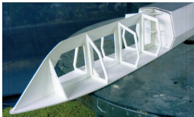
The Plasticard frames in place
