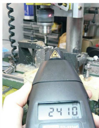
Measuring the speed of a drill press chuck
