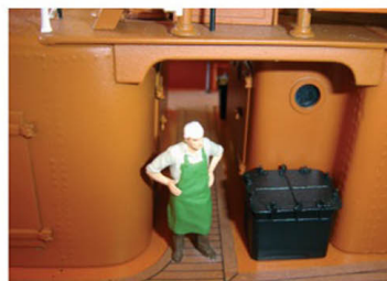
Showing the perfect fit of the bridge deck into the recess of the front superstructure. This is the main superstructure break point for removal
