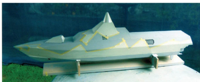
Masked using Tamiya tape for the camouflage
