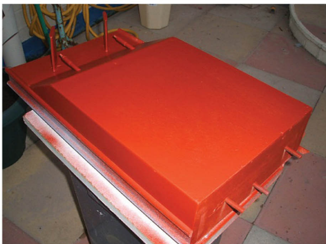
Lower hull painted with red oxide
