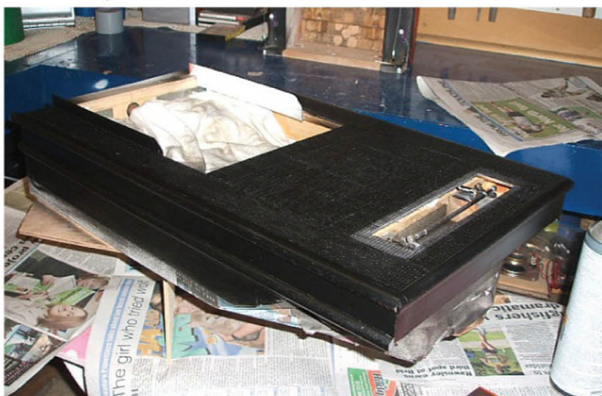
Lower hull masked off and tops sprayed satin black
