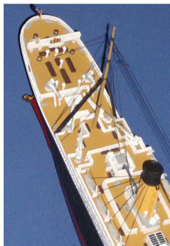
Deck superstructure parts were built and painted as sub-assemblies
