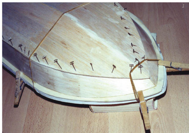
Fig 5a – Extra support to hold the bow shape with elastic band clamps and pins
