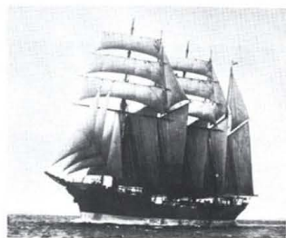
A real oddity, the Carl Vinnen, one of the five Vinnen sisters, built to try and keep sail alive as an economic proposition in the 1920s. Described as "a three masted topsail schooner, chasing a two masted topsail schooner!"
