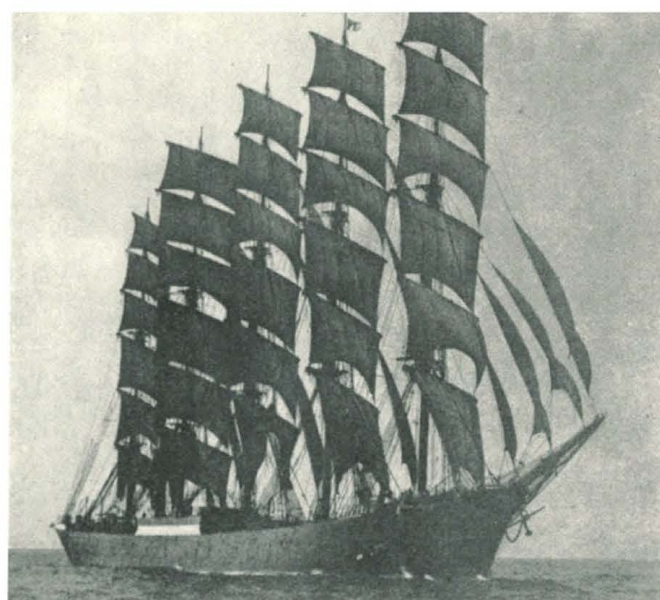
Preussen at sea, under all sail. The original, German caption of this picture calls her "majestic", and I cannot but agree. Her port anchor is hanging from the 'cathead', showing that she is close to land, either arriving or departing
