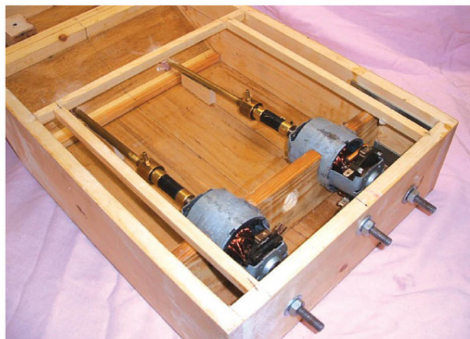
New motors dry fitted to shafts
