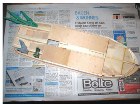
You are so cheap: the hull has been constructed using balsa and plywood
