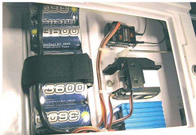
The Impulse 26's moulded plastic hull uses a separate/glued-in inner structure to provide the battery, ESC, rudder servo and receiver-mounting points and a dual Velcro strip/strap set-up retains the NiMH pack to the boat
