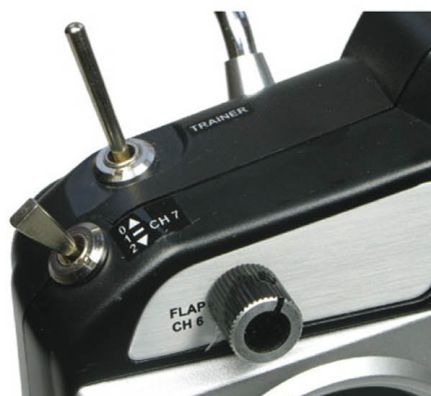
Channel 6 is a rotary proportional control, Channel 7 is a three-position switch
