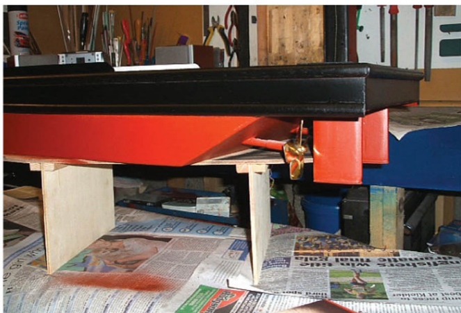
Ready to apply waterline in white tape
