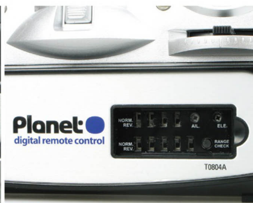
Channel reversing switches are behind a removable panel
