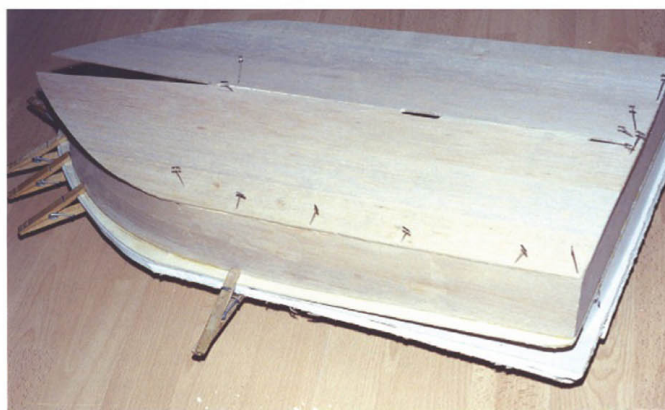
Fig 5 – Fitting the bottom hull panels
