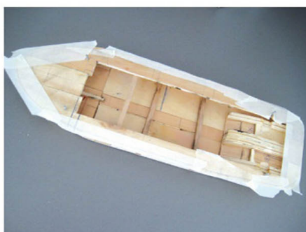
Tunnels for the propellers are visible in the aft end of the hull
