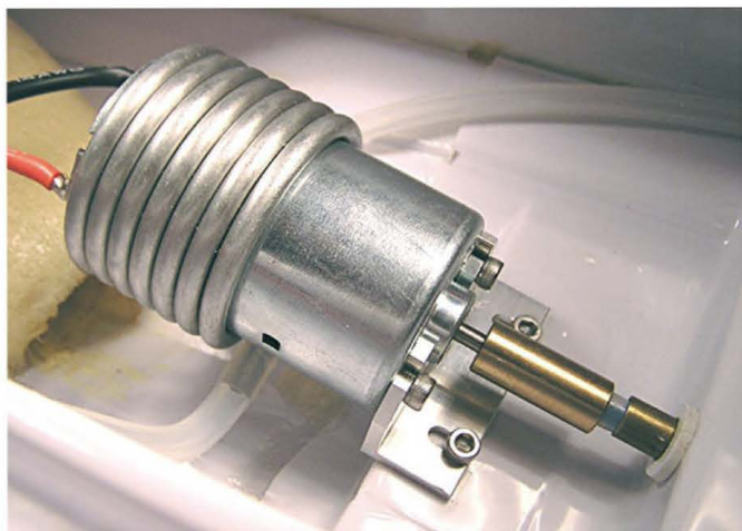
Water-cooled and bolted to the hull with an aluminium bracket the 26's brushed DC motor has a dual grub-screw coupler to join the motor to the flexible drive line
