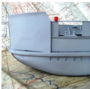
The bow's shape eased beaching, the two doors gave full access to the cargo hold
