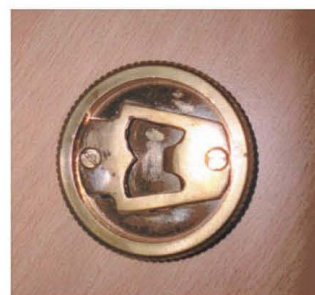
Bottom of the key screwed in place
