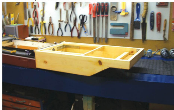
New stern section completed using pine and ply
