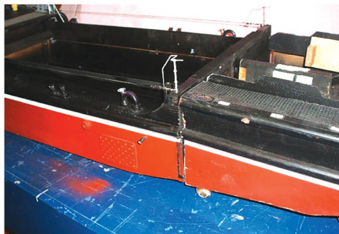
The stern section sawn off the hull
