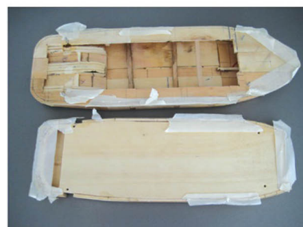
PiLaBo 39 hull and deck are separated to allow for R/C installation
