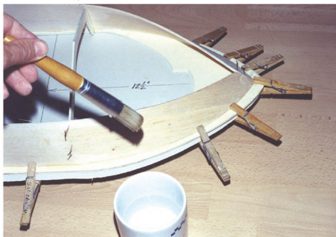
Fig 4 – Clothespins used to hold the bow side panels after a coat of water to help bending
