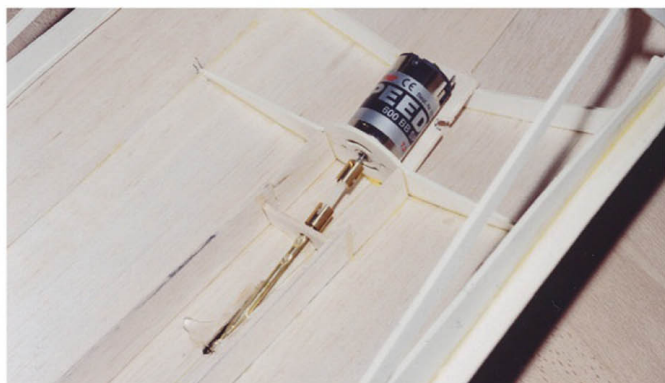
Fig 8 – Check alignment for the motor and prop shaft
