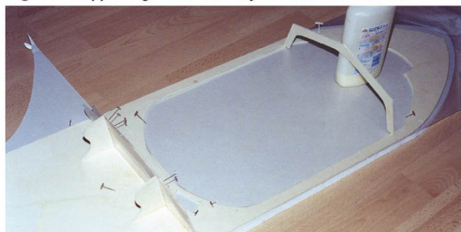
Fig 2 – Assembling the transom using the angled guide pieces
