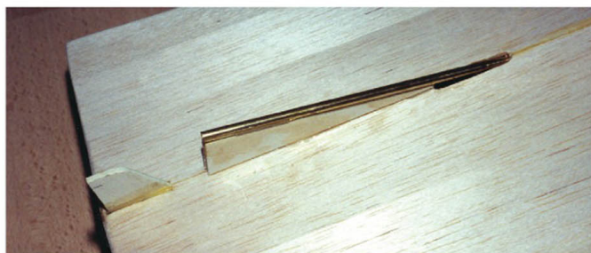
Fig 7 – Prop tube now in place
