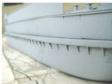
Supporting struts have been largely made from cardboard
