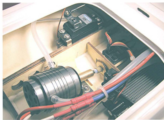
Water-cooled and bolted to the hull with an aluminium bracket the 26's brushed DC motor has a dual grub-screw coupler to join the motor to the flexible drive line
