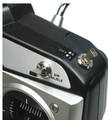
Channel 5 is a two-position slow or normal switch
