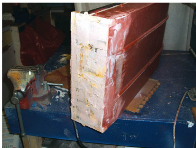
Filler applied to bulkhead to be sanded down
