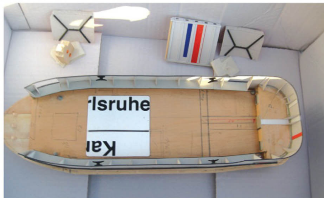
Main components of PiLaBo 39 are assembled and ready for the first layer of primer
