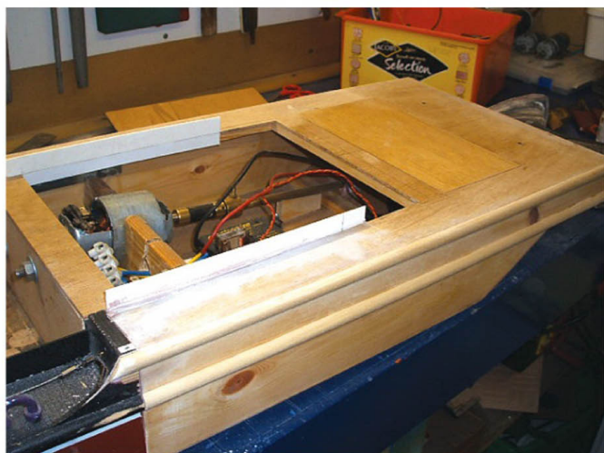
Mouldings added to hull
