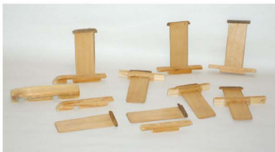
The leeboards and their support blocks were made early
