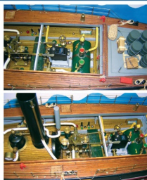
Imperial German Navy Seaplane Tender named 'Greif (Griffon)'. Built from drawings and a picture of the ship in Zeebrugge Harbour (Belgium) 1917. Again the boiler and engine have been home-made. Length 1 m, beam 26 cm. Powered by a gas burner it has a run time of 45 minutes at low speed. MIMI
