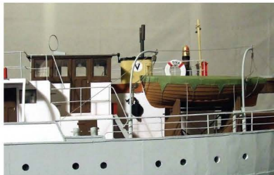
Close-up of the wheelhouse and lifeboat – the clinker hull of the boat is formed with strips of thin card
