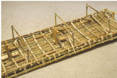
The supports for the hogging trusses, held in place initially with clothes pegs and sheering elastic
