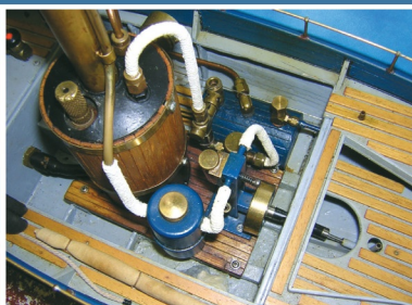
Imperial Russian Navy Torpedo Boat used in the Black Sea called 'Nakhimov'. Again built from plan with a picture to 1/25 scale. All wood construction with length 85 cm, beam 14 cm. Boiler and engine from France (Anton). Gas powered with a run time of 20 minutes (10 minutes at high speed).
