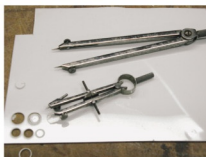
Types of compass or divider used to score/cut circles. The top ones are usable with care, but the bottom ones are the preferred type
