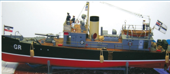
Imperial German Navy Seaplane Tender named 'Greif (Griffon)'. Built from drawings and a picture of the ship in Zeebrugge Harbour (Belgium) 1917. Again the boiler and engine have been home-made. Length 1 m, beam 26 cm. Powered by a gas burner it has a run time of 45 minutes at low speed. MIMI
