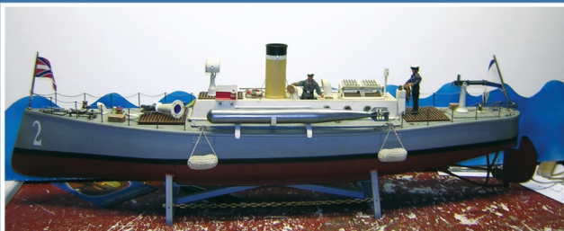
French Gun Boat 1870 Type Farcy named 'Liberte' (built to defend Paris). Scratch-built from a plan and photograph to 1/25 scale (approx) with all wood construction. Boiler and engine home-made. Length 52 cm, beam 20 cm. Fuelled by a gas burner, which gives a run time of about 18 minutes.
