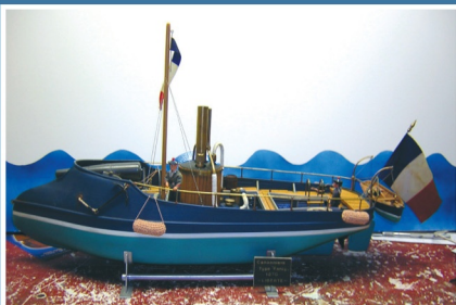
Imperial Russian Navy Torpedo Boat used in the Black Sea called 'Nakhimov'. Again built from plan with a picture to 1/25 scale. All wood construction with length 85 cm, beam 14 cm. Boiler and engine from France (Anton). Gas powered with a run time of 20 minutes (10 minutes at high speed).
