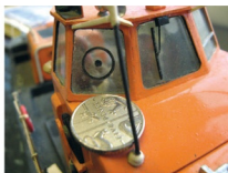
Representation of rotating clearview screen on small model lifeboat. The 5p coin gives idea of scale
