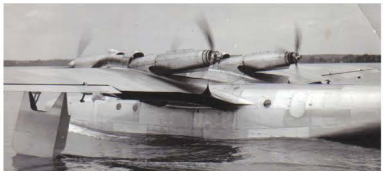
Another shot of a pre-series Dornier Do 26. To avoid the backside propellers being affected by spray, they could be uplifted during taxiing and take-off
