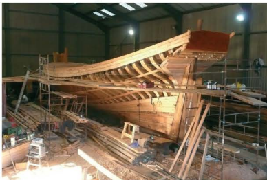
The stunning lines can clearly be seen with the hull partially planked
