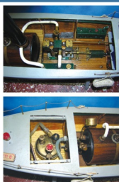
French Gun Boat 1870 Type Farcy named 'Liberte' (built to defend Paris). Scratch-built from a plan and photograph to 1/25 scale (approx) with all wood construction. Boiler and engine home-made. Length 52 cm, beam 20 cm. Fuelled by a gas burner, which gives a run time of about 18 minutes.
