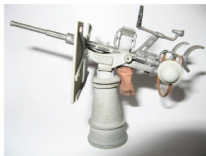
Scratch-built 1/24th scale Oerlikon Cannon. The conical stand is turned aluminium, the support strap is paper, the spent cartridge bag is linen. Everything else including the barrel is plastic
