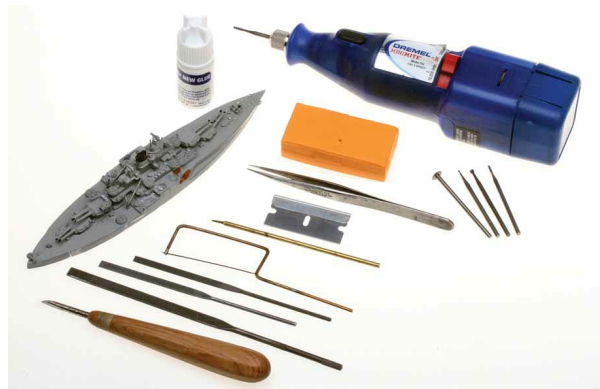
Tools and materials used in Thunderbolt project of Superior West Virginia: Dremel rotary tool, burrs, unfired polymer clay, forceps, safety razor, home-made brass punch, home-made saw, needle files, artist-made
