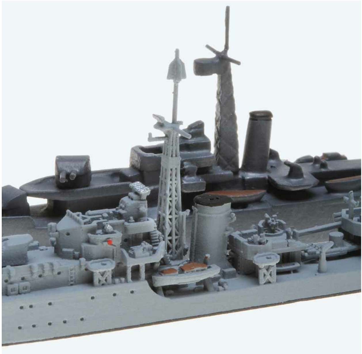
Destroyer HMS Cavendish and Fleetline HMS Amethyst , 1944. Spider Navy/NN-CAD cast lattice mast of Cavendish very good compared to 1970s technology/modelling of Amethyst lattice mast, where the lattice is simply represented by incised lines.
