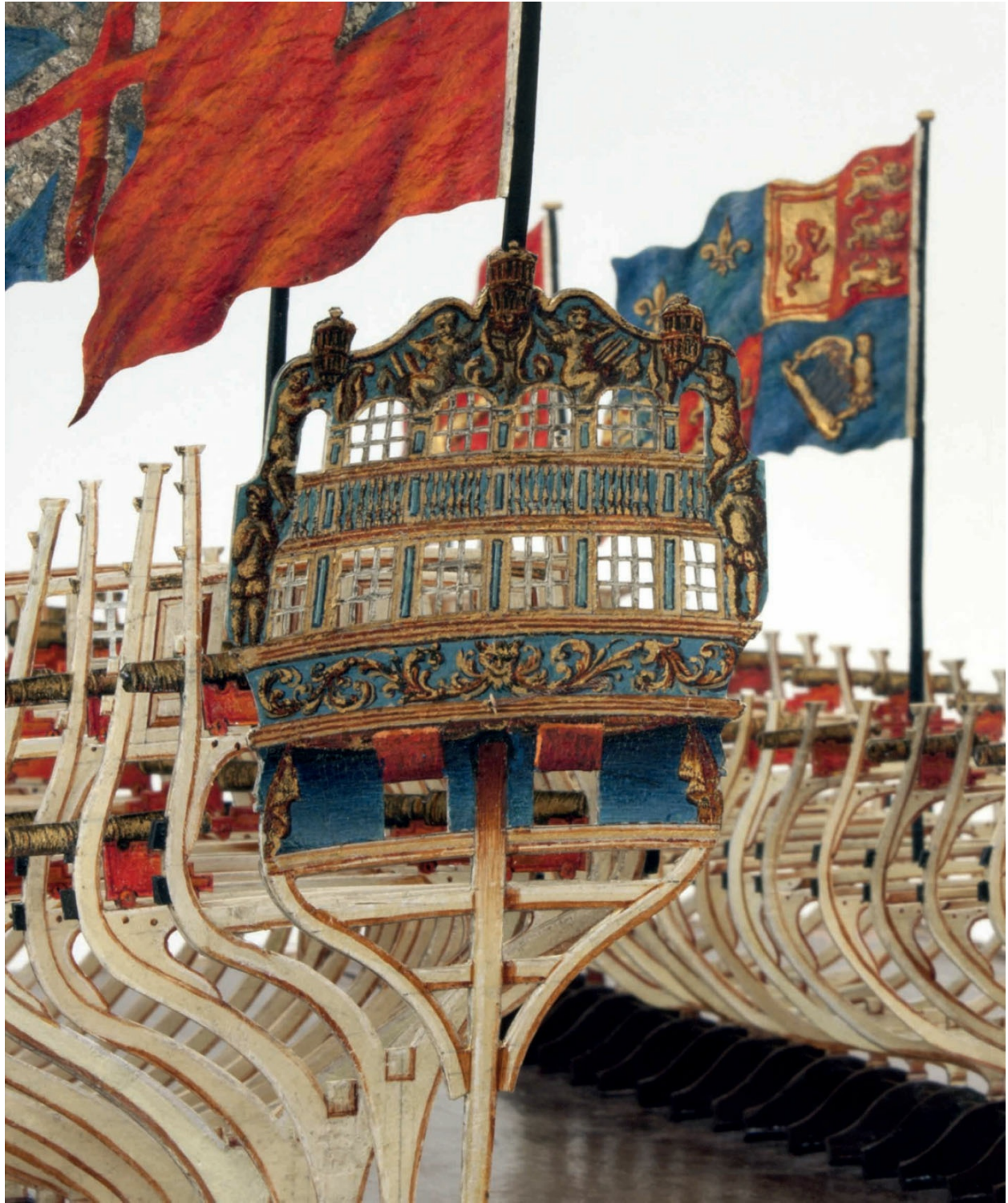
Note the trompe-l'oeil gun port lids and stern lanterns and the way the gun deck can be viewed through the open chase ports. The knotted thread with toggle stop centred just above the counter is also visible.
