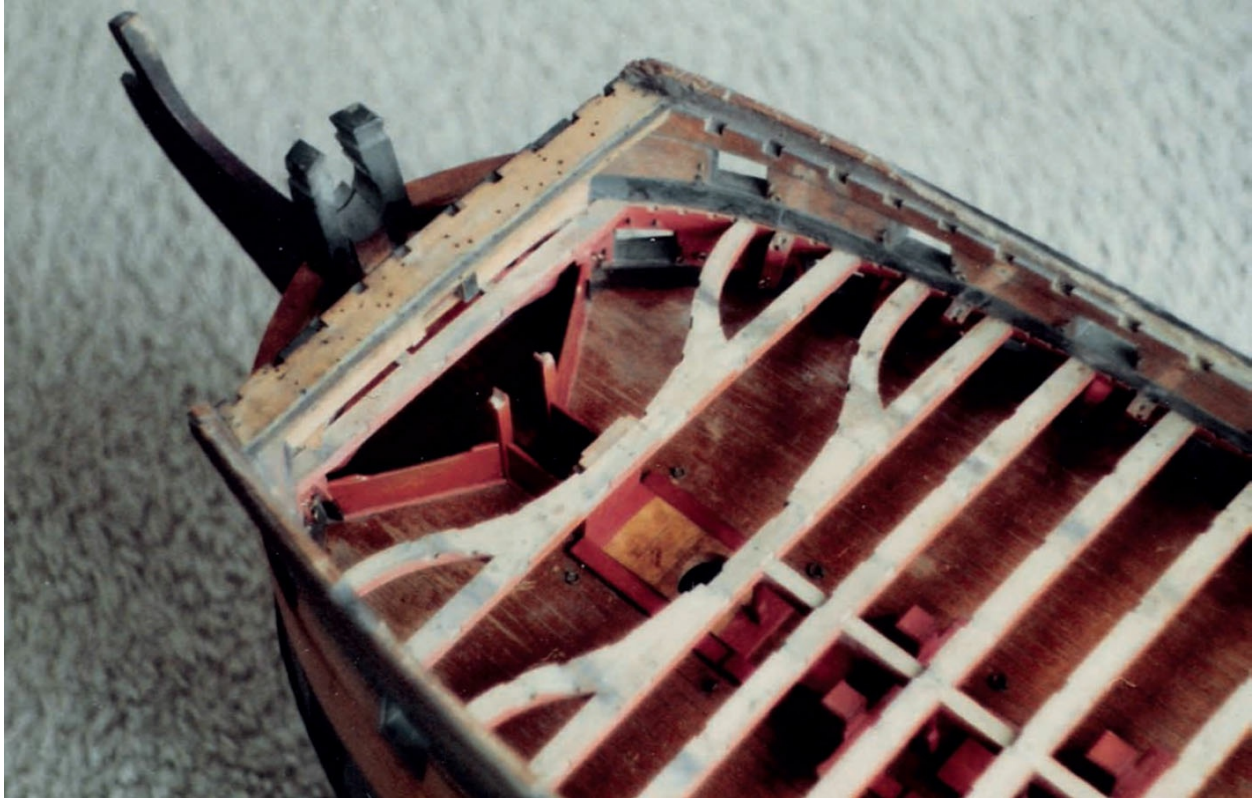
This photograph was taken while the model was taken apart for cleaning. The upper deck beams remain in place, and chamfers for carlings, ledges and forecastle deck beams can be seen.
