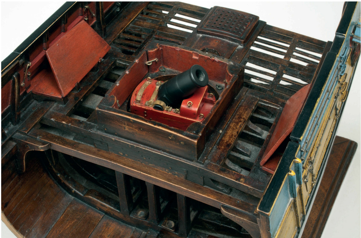
The fine detail and fittings of the mortar bed and pit can be seen, along with the
