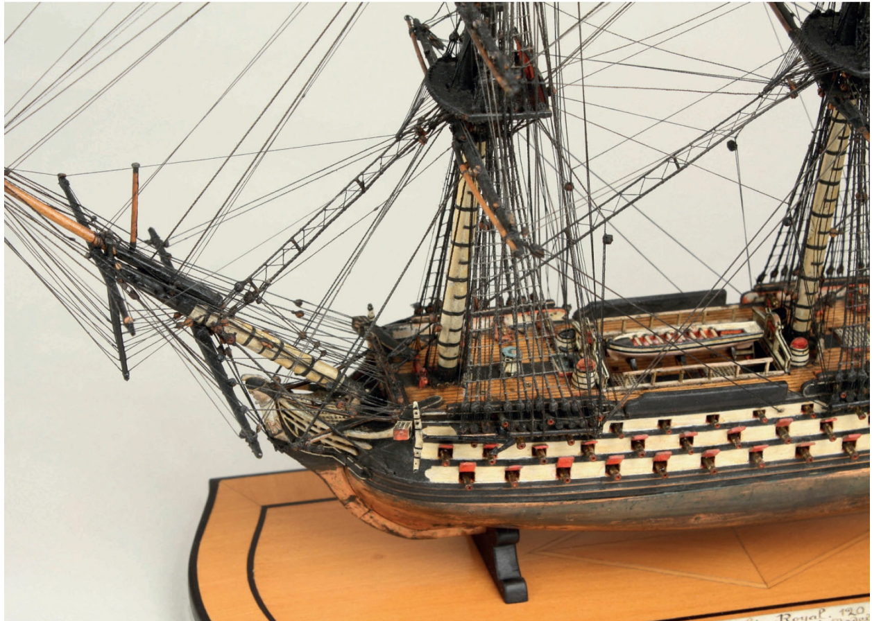
A finely detailed small boxwood PoW model with coppered hull and colourful deck details. Note that there is a watch bell at the quarterdeck breastwork in French fashion.
