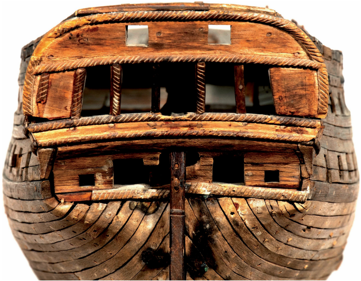
The simple stern with its single closed gallery. The only decorative carvings remaining on the model are simple rope mouldings around the stern lights and quarter galleries.
