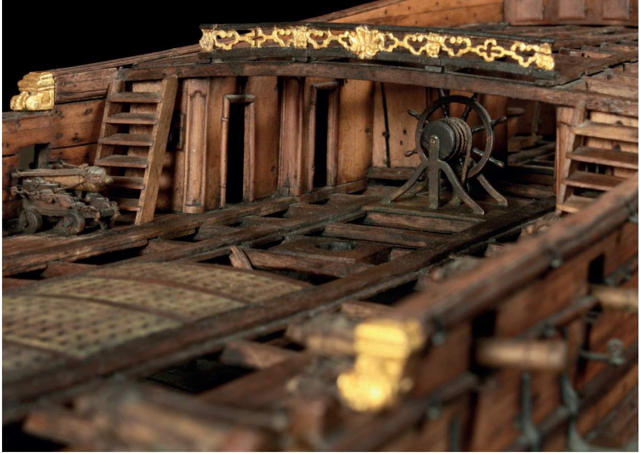
A view of the quarterdeck showing the poop breastwork carved with an openwork frieze, mirroring the forecastle breastwork carving. The single wheel is mounted on metal pillars just beneath the poop. Open doorways lead to two starboard sleeping cabins for officers. Note the moulded corner stanchions of the bulkheads. Ladders providing access to the poop deck are fitted on each side.
