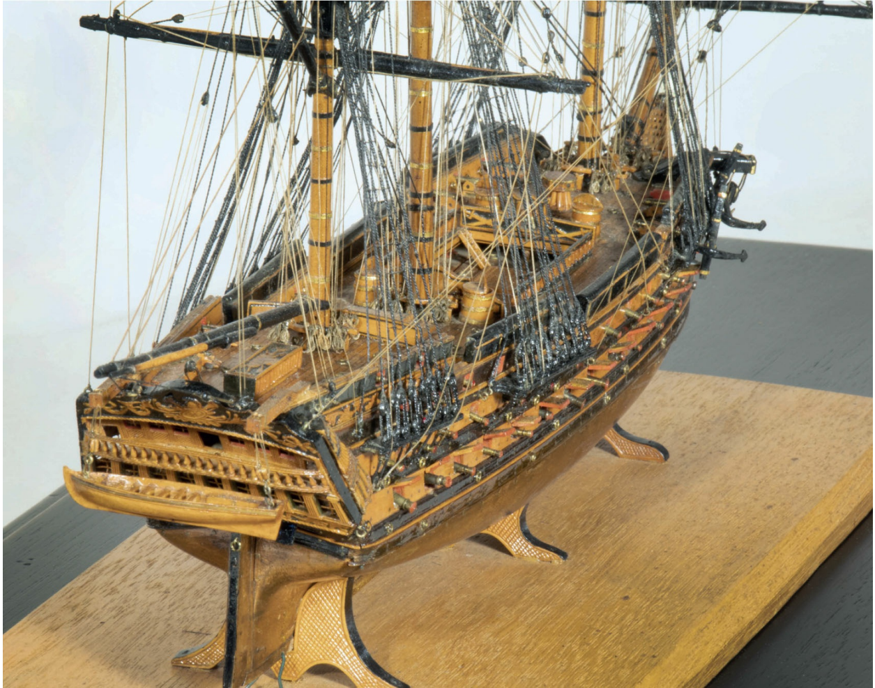
A small boxwood copper hull model with fine carved decorations on the taffrail, forecastle breastwork and along the frieze planking.
