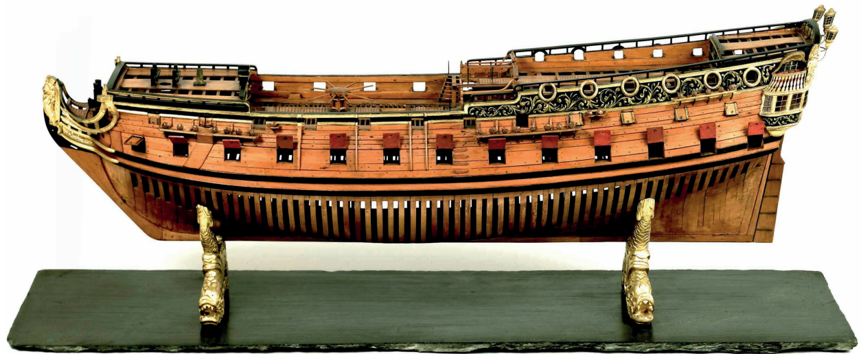
Broadside view showing the well balanced but relatively modest scale of the head and quarter galleries on this well-armed two-decker.
