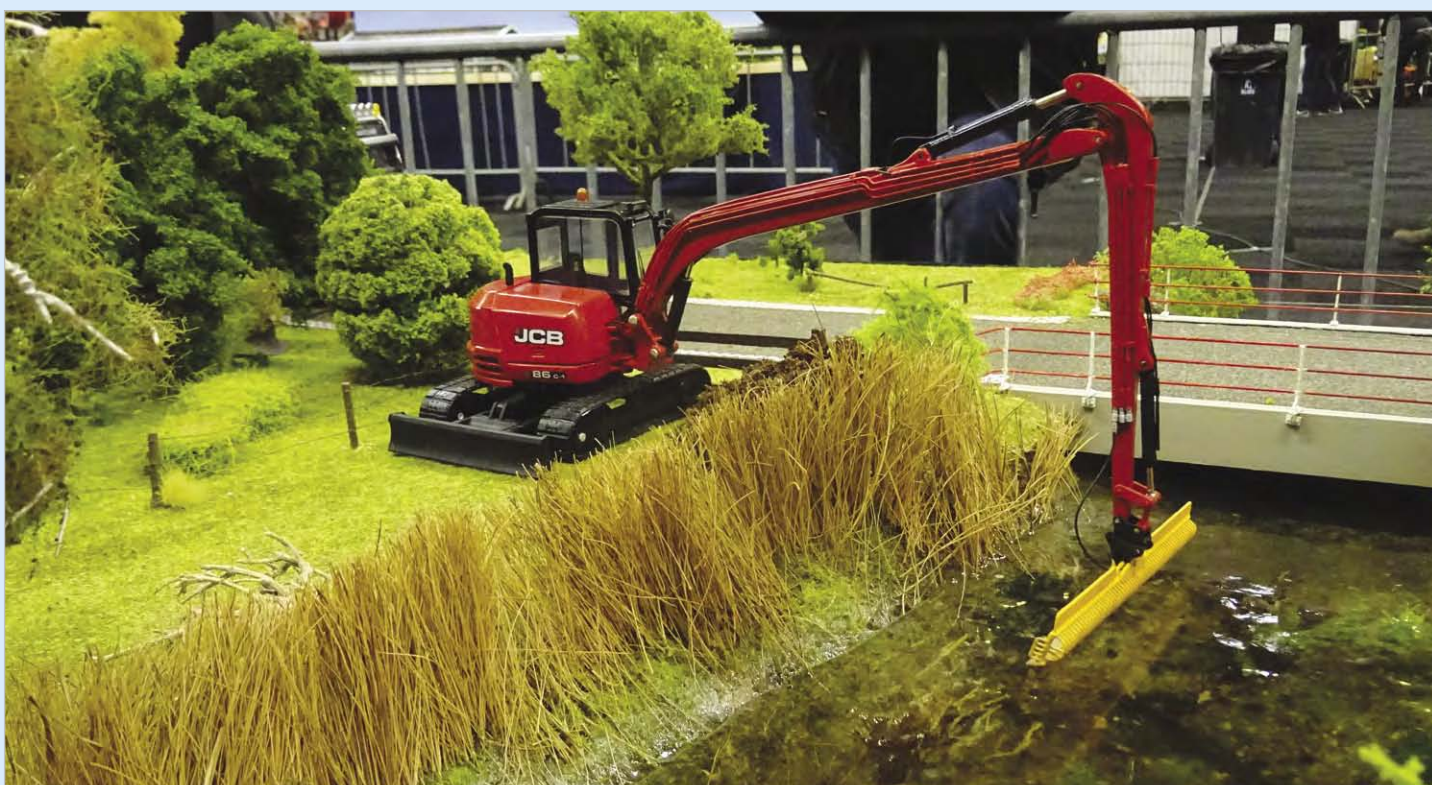
A converted JCB 86C in red with extended boom and mowing bucket for cleaning out the ditches. This model has been made by 21 years young Mathew Arntz from Wijchen, the Netherlands.
