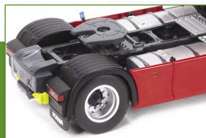
The chassis has side panels, silver fuel tanks and fifth wheel coupling plate.
