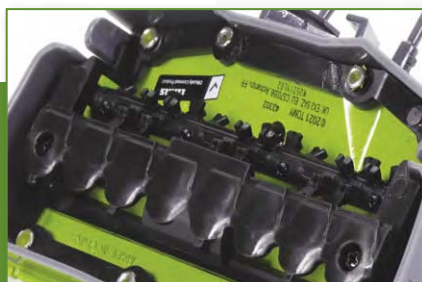
The underside detailing of the MAX CUT mower bar and rotating tine conditioning drum.
