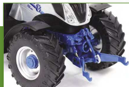
The front linkage is height adjustable with the arms foldable.
