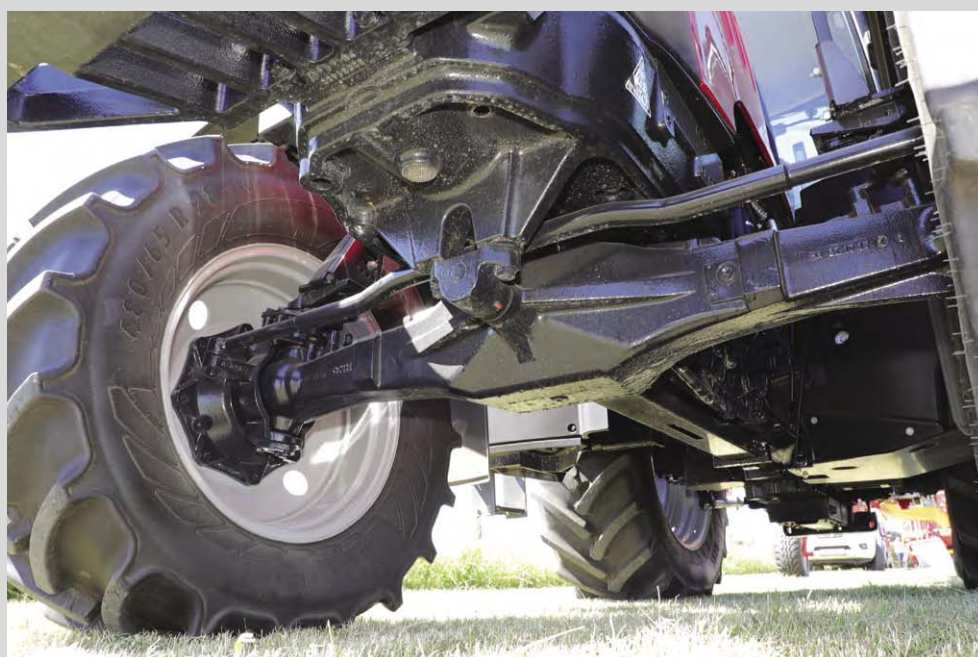
Above: Standard front axle with optional front axle suspension. Front brakes are optional too.
