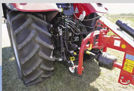
Above: The Puma X rear hitch can lift 8,257kg and the hydraulic system uses an axial piston variable displacement pump with a delivery rate of up to 110 l/min.
