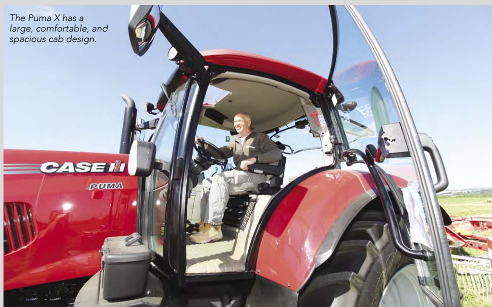
Above: Fuel and AdBlue tanks are situated next to the O/S door.
