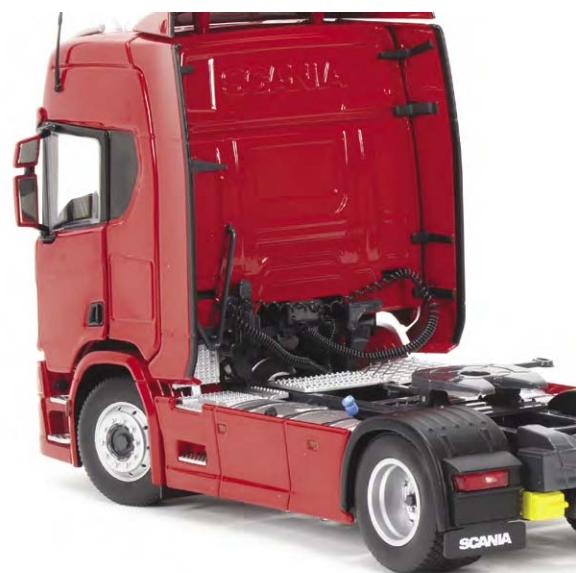
Above: Added details include the wheel chocks and air tanks fixed to the chassis.
