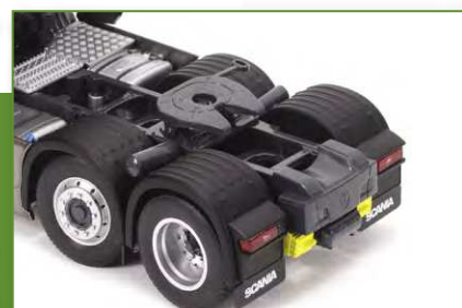
The 6x2 chassis has air tanks between the rear wheels with linked steering of the front and middle axles.
