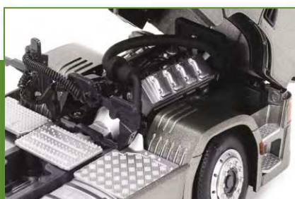
Textured walkways are fitted behind the cabin along with coiled service lines.
