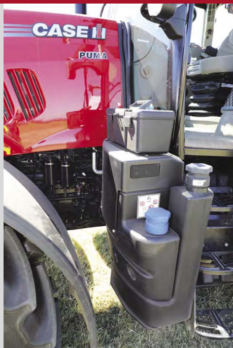
Above: Fuel and AdBlue tanks are situated next to the O/S door.
