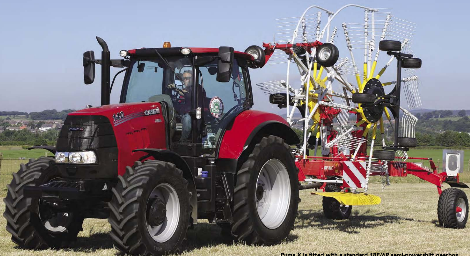
Puma X is fitted with a standard 18F/6R semi-powershift gearbox with smooth clutch less gear changes up to 40 km/h.
