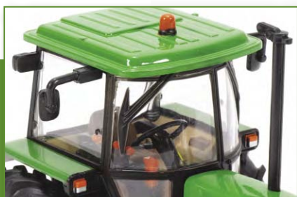
Exterior detailing of the cabins includes rear view mirrors, work lights, screen wiper and amber beacon.
