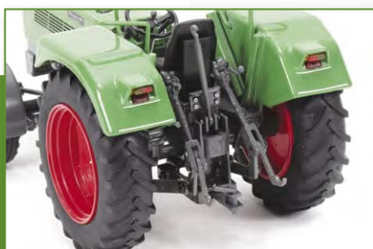
The implement linkage on all the models is height adjustable with pivoting upper link bar.
