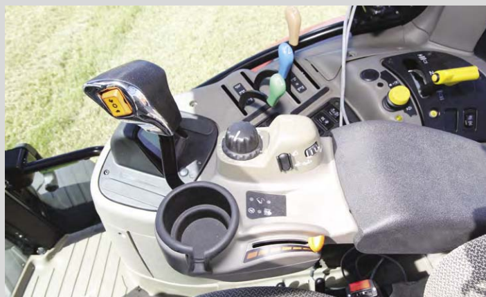
Above: Easy to reach and simple controls for gear change / selection, diff-lock, three spool valves with the option of having four fitted.
