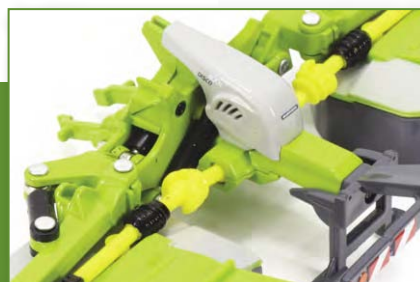
The rear mowers use a clever ball and socket connection to allow the mowers to fold up.
