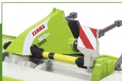
The front housing and driveshafts to power the cutting discs and conditioner are neatly implemented.
