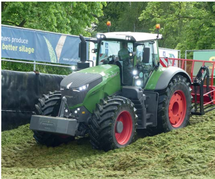
Above: Reverse drive 542hp Fendt 1050 Vario taking it's turn to be demonstrated on one of the two clamps.
