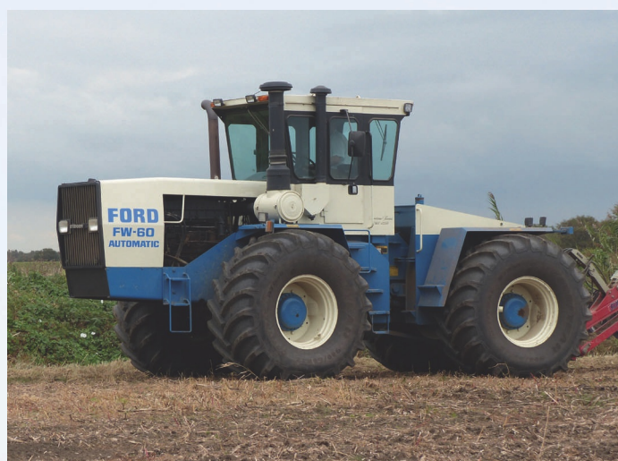
This particular FW60 was another tractor given a nut and bolt refurbishment by Amtrac at Bedale. The tractor's Cummins motor now pumping out an impressive 420hp.
