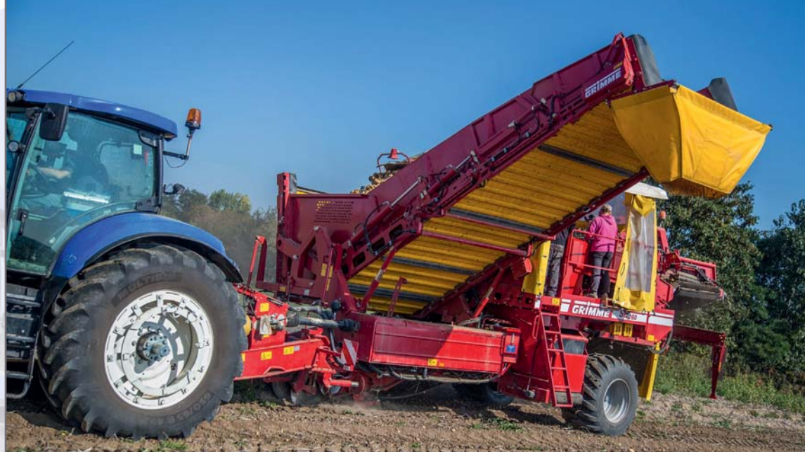
Above: Grimme's SE260 sets the standard in its category. It has a capacity of 6 tonnes, is 10.7m long and 3.3m wide. Options include a steering axle, multiple cameras, automatic levelling and a joystick control system.
