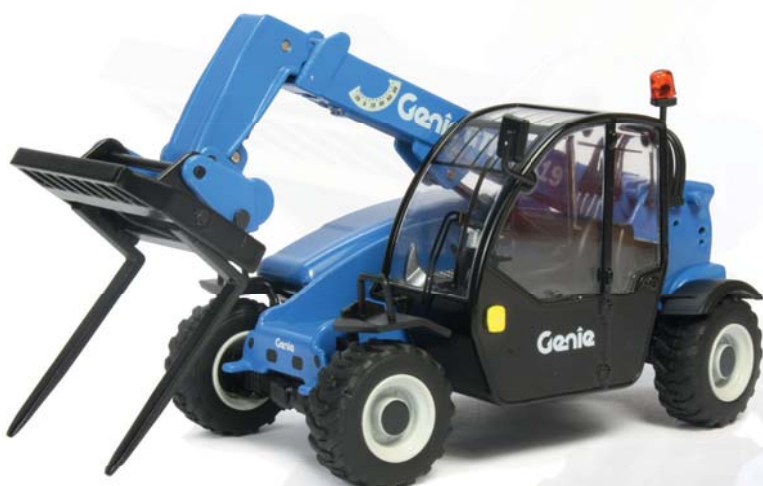
Above: Both versions have steering front and rear axles allowing crab steering to be demonstrated.
