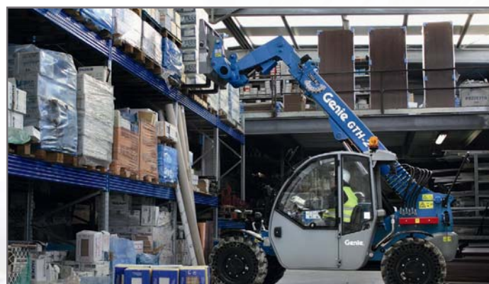
Above: Both versions have steering front and rear axles allowing crab steering to be demonstrated.
