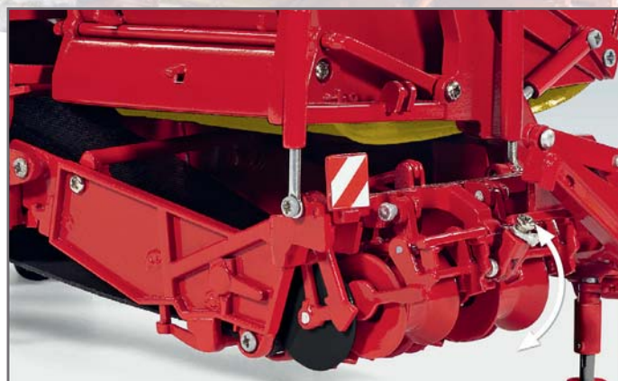
Above: The two digging share units move up and down independently and both the hulk discs diablo rollers rotate.
