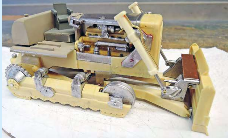
New cylinder brackets on tractor and blade.
