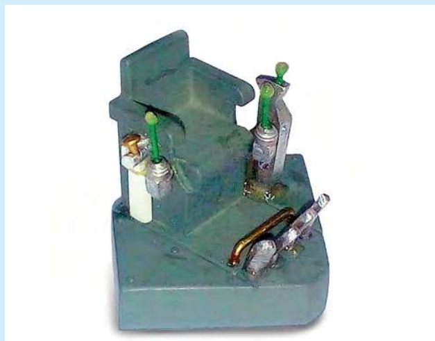
Modified operator's seat with four pedals.
