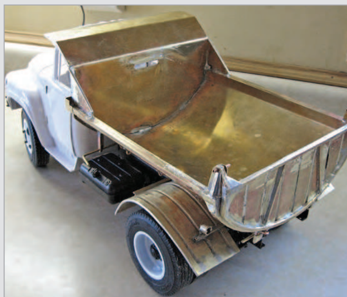
Forming the standard Zil 130 dump body using soldered sheet brass. Various solders, each with different melting points, were used to avoid later parts from overheating and releasing previously soldered assemblies.
