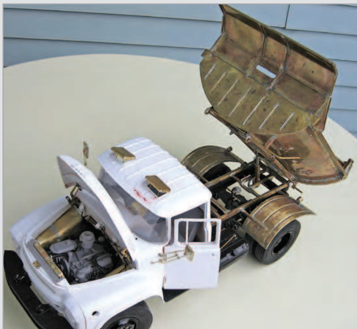
Before priming and painting, the main assemblies were lightly fastened together to check their fit and tolerances.
