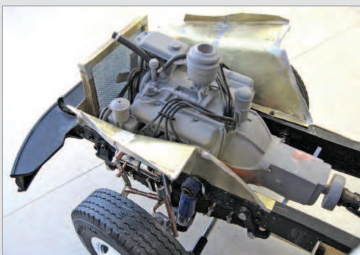
The motor was loosely positioned, to check its fit, between the beginnings of the brass wheel well inner liners as well as the unfinished radiator.
