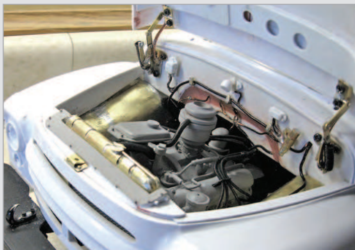
Detailing the engine bay comprised a new, accurate plastic firewall with the necessary wiring, coil, and voltage regulator from brass. Further details included a small firewall maintenance lamp, working hood hinges, a new brass radiator and bonnet hold-down latch. The underside of the bonnet also had the intake plenum chamber added.
