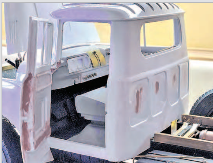
The dashboard and instrument panel were replaced with new polystyrene versions, while the opening glove-box door, as well as the various knobs and grab-bar, were all brass. The cab floor and 'rubber' mat were both fabricated in polystyrene as well as a driver's folding sun-visor from plastic and stiff wire.
