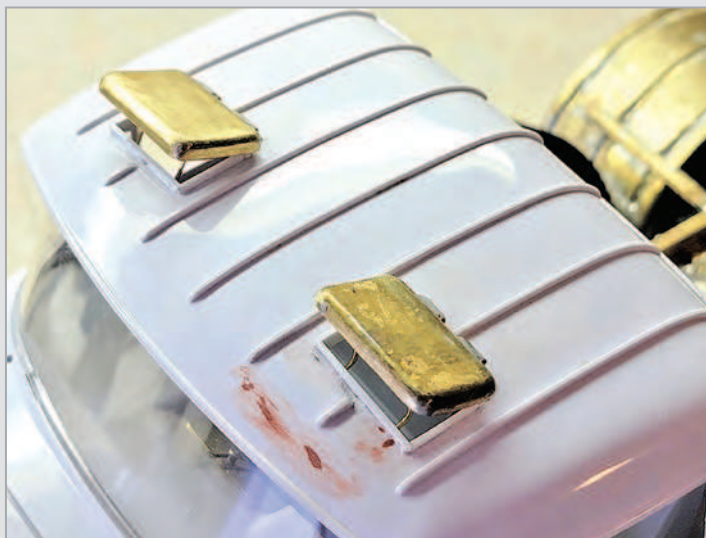
The opening roof air-vents were fabricated in brass.
