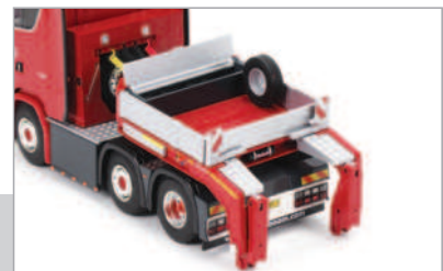
Above: The gooseneck can be detached from the load floor and has a functional storage box and spare wheel.
