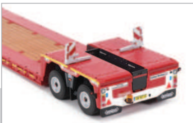
Above: The rear module has an excavator trough with detachable panels and wide-load marker boards.
