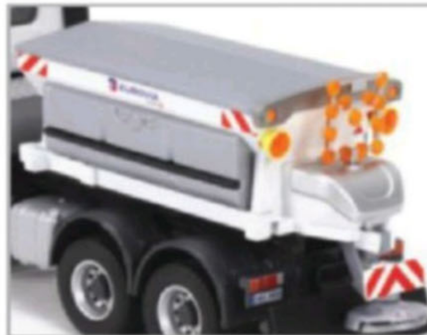
Below: The gritter unit on the Arocs uses new tooling, permanently fixed to the truck chassis.
