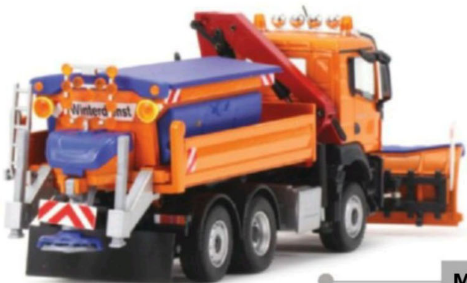
Above: The MAN TGS NN is a tipper truck at heart, with detachable gritting unit.
