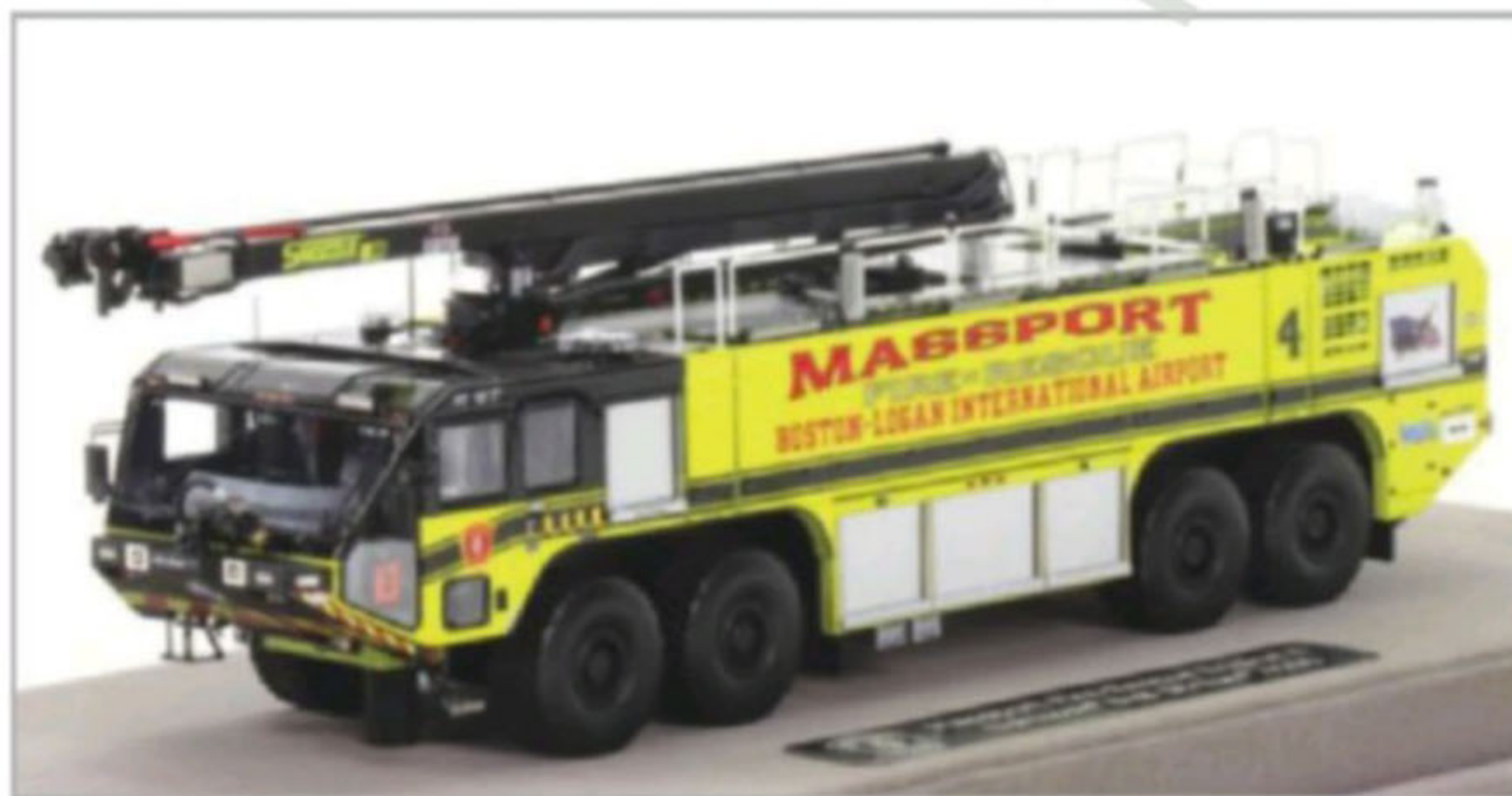
Above: Still available are the larger Striker 4500 8x8 ARFF vehicles decorated in the Massport Fire Rescue colours at the Boston-Logan International Airport, truck 3 with bumper and roof turrets and truck 4 with Snozzle.
