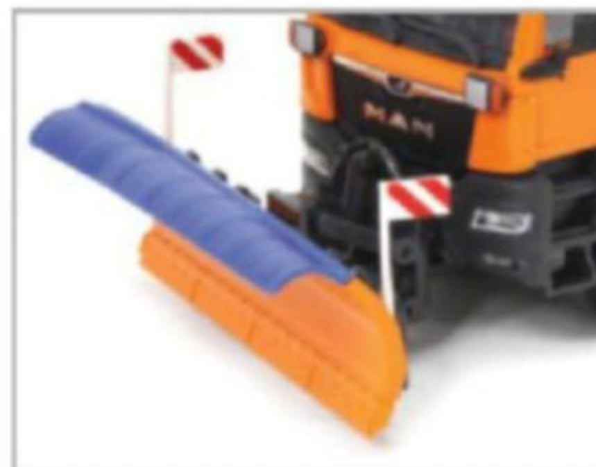
Above: The front plough has both height and angular movement, complete with small width markers.
