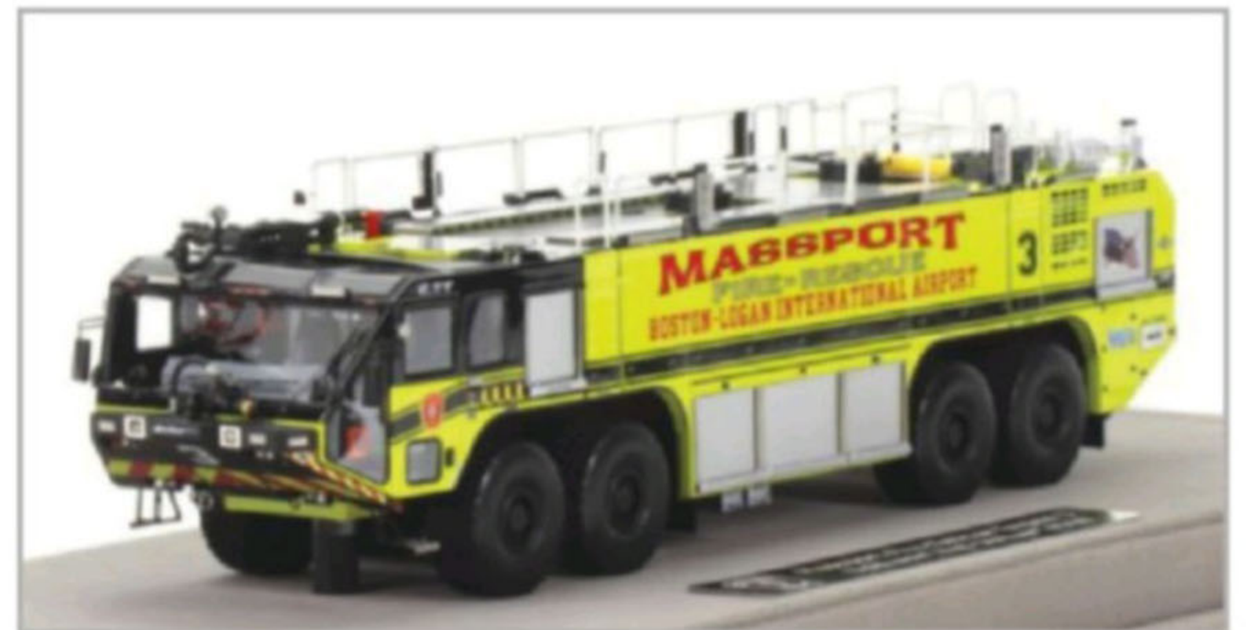
Above: Still available are the larger Striker 4500 8x8 ARFF vehicles decorated in the Massport Fire Rescue colours at the Boston-Logan International Airport, truck 3 with bumper and roof turrets and truck 4 with Snozzle.
