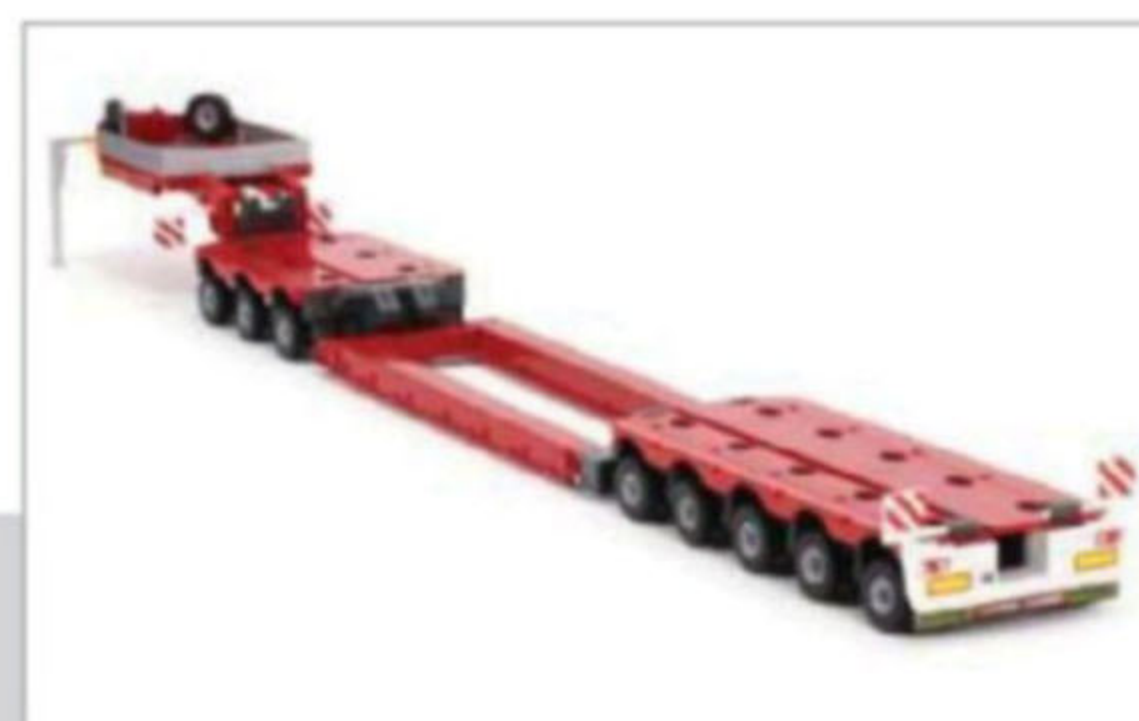
Above: Another option is a low loader with three-axle module at the front and five-axle module at the rear. It is also possible to omit the front module, connecting the floor directly to the gooseneck.
