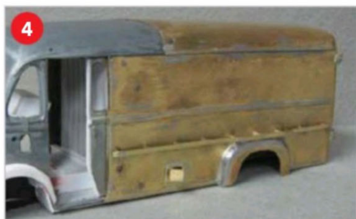
4 Addition of the soldered brass side protector rub-rails, as well as the opening fuel filler door.
