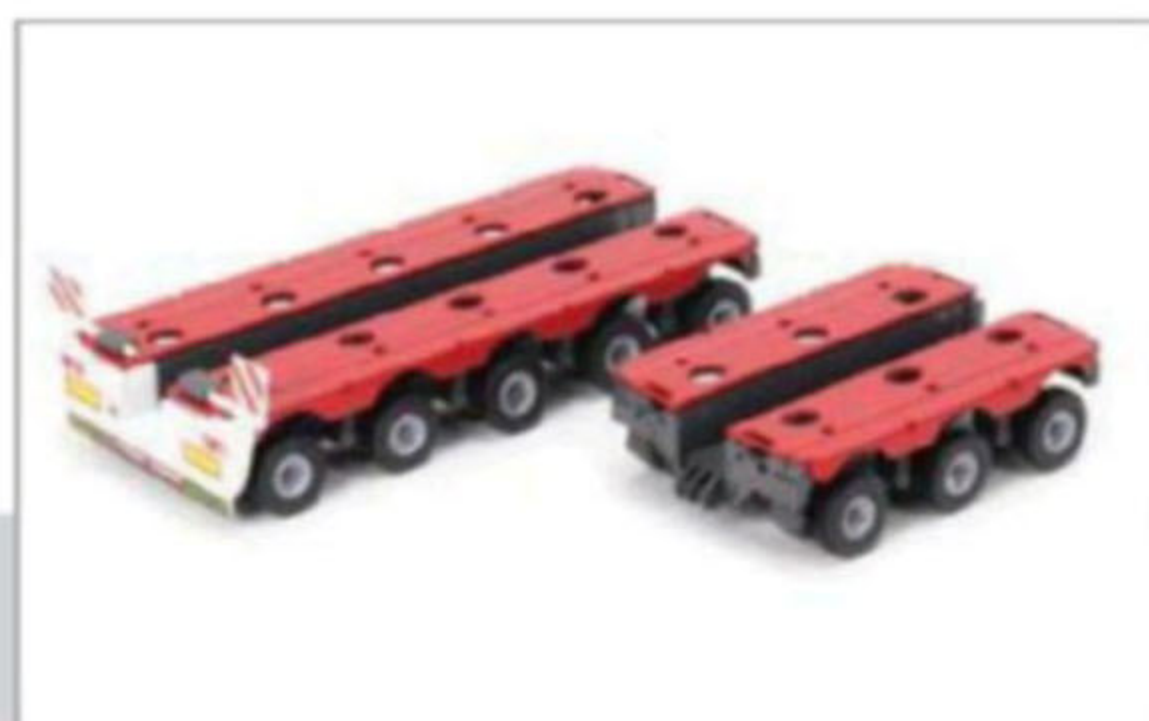
Above: There is a three-axle line and a five-axle line module with end panel displaying the lights and markings.
