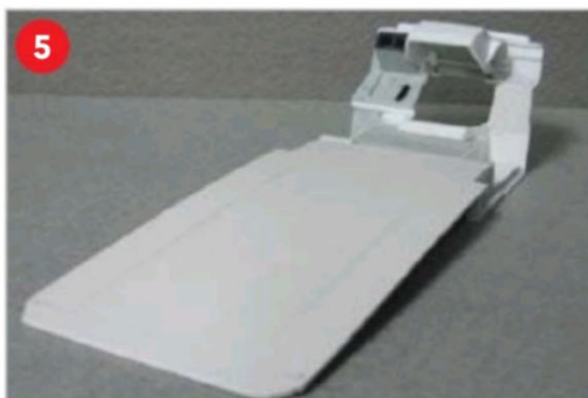
5 Forming of the interior floor detail with its opening engine access cover.
