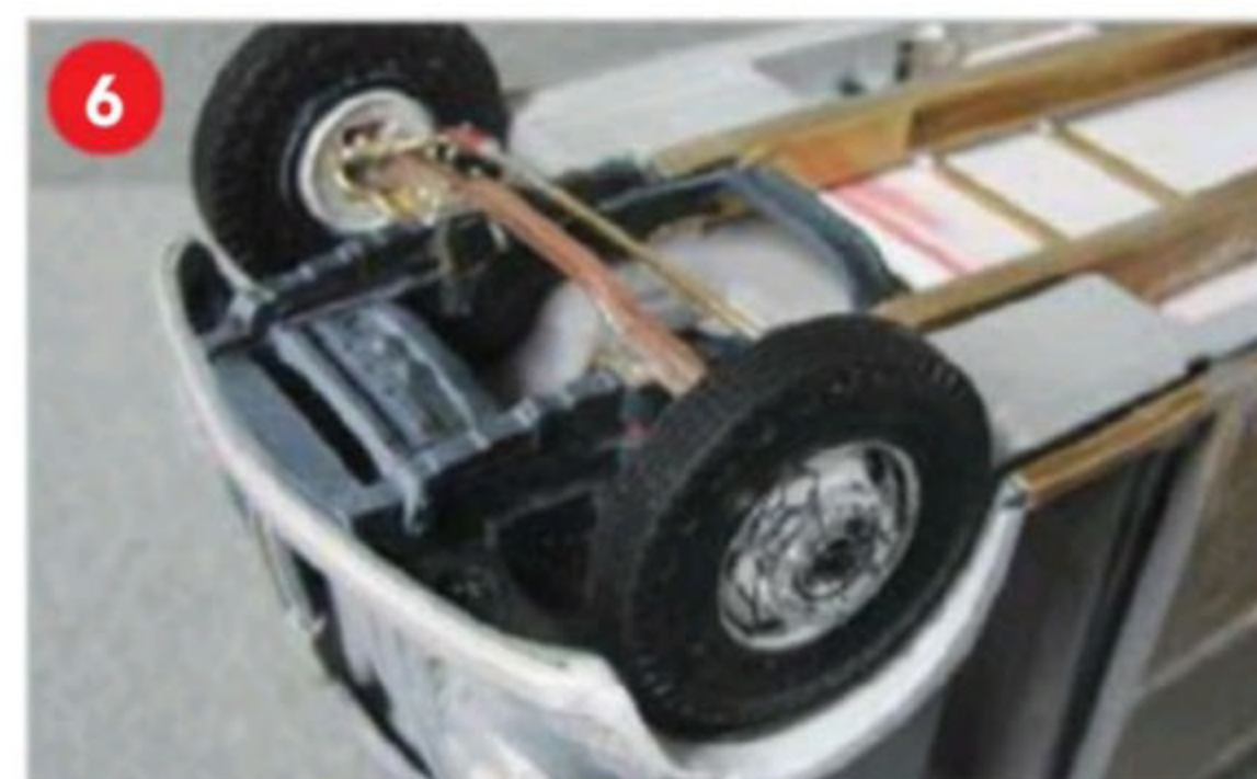
6 Early chassis development with the soldered brass steering I-beam front axle.
