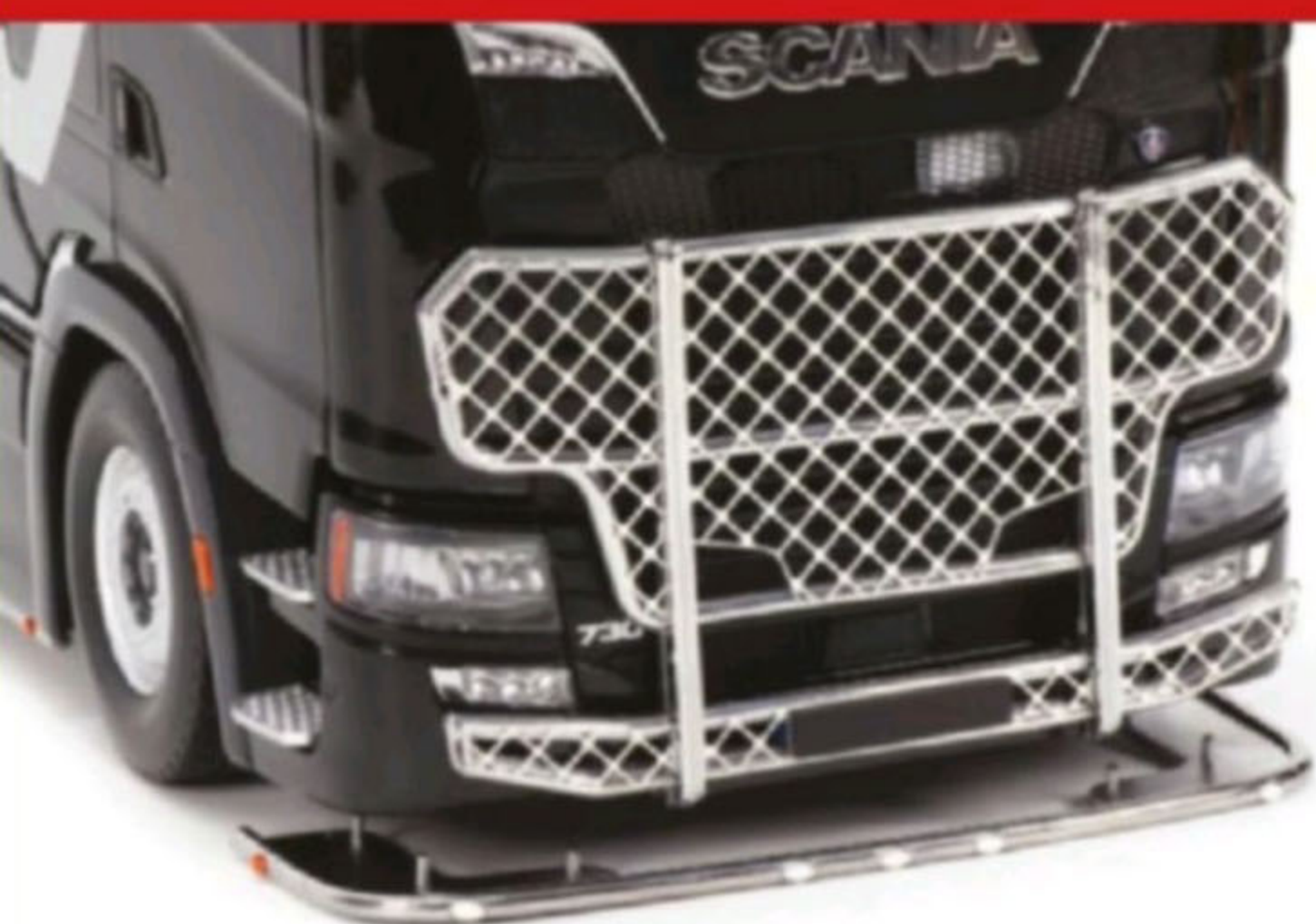
Left: The protective mesh really enhances the appearance of the truck, hinging down to allow the cabin to tilt.
