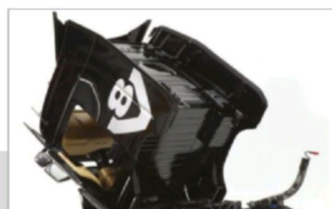
Above: The entire cabin can be tilted forward to uncover the engine area.
