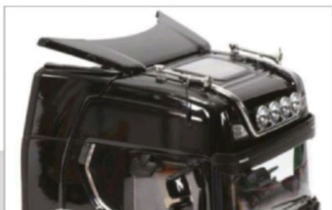
Above: The upper spoiler can be adjusted in height which is a nice touch.
