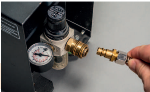
a) Connect the pressure hoses to the compressor using the male quick connector.
