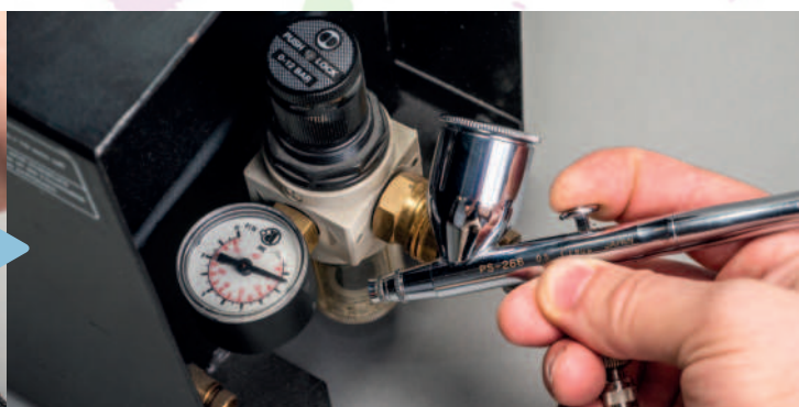
c) The air pressure is adjusted by means of the regulator. It should be noted that the actual working pressure can only be seen on the pressure gauge when the trigger of the air valve of the airbrush is pulled.
