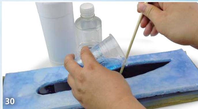
30 First the epoxy resin was gently poured into the submarine's position.
