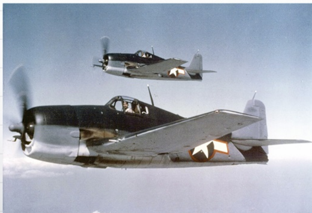
Two Grumman F6F-3 Hellcat fighters in a three-colour countershading camouflage: sea blue, intermediate blue, and insignia white. (US Navy National Museum of Naval Aviation)
