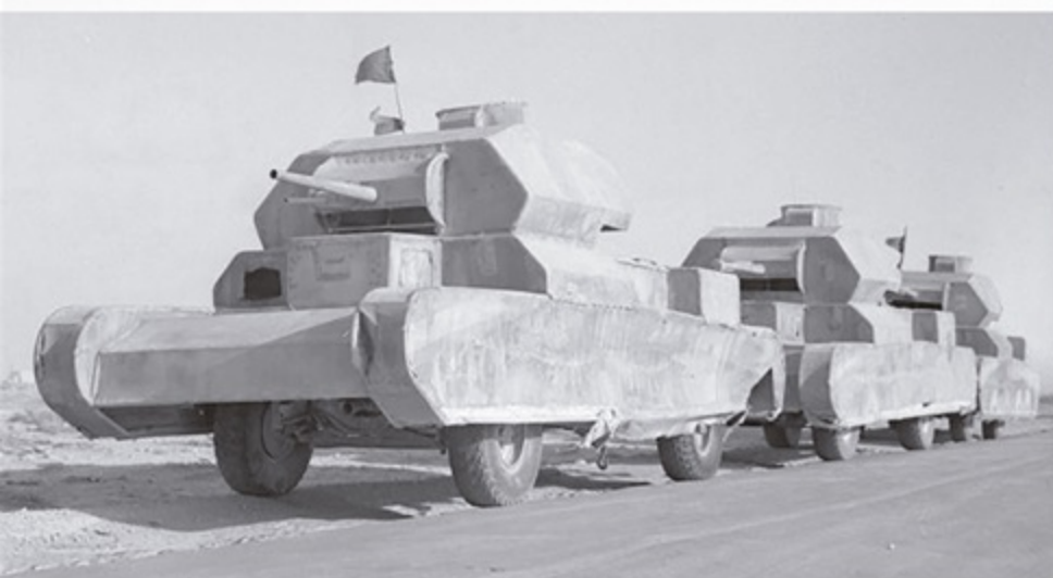
Dummy tanks made by a superstructure mounted on trucks. Western Desert, 13 February 1942. The disguise is not strictly part of the camouflage techniques. (IWM E8361)
