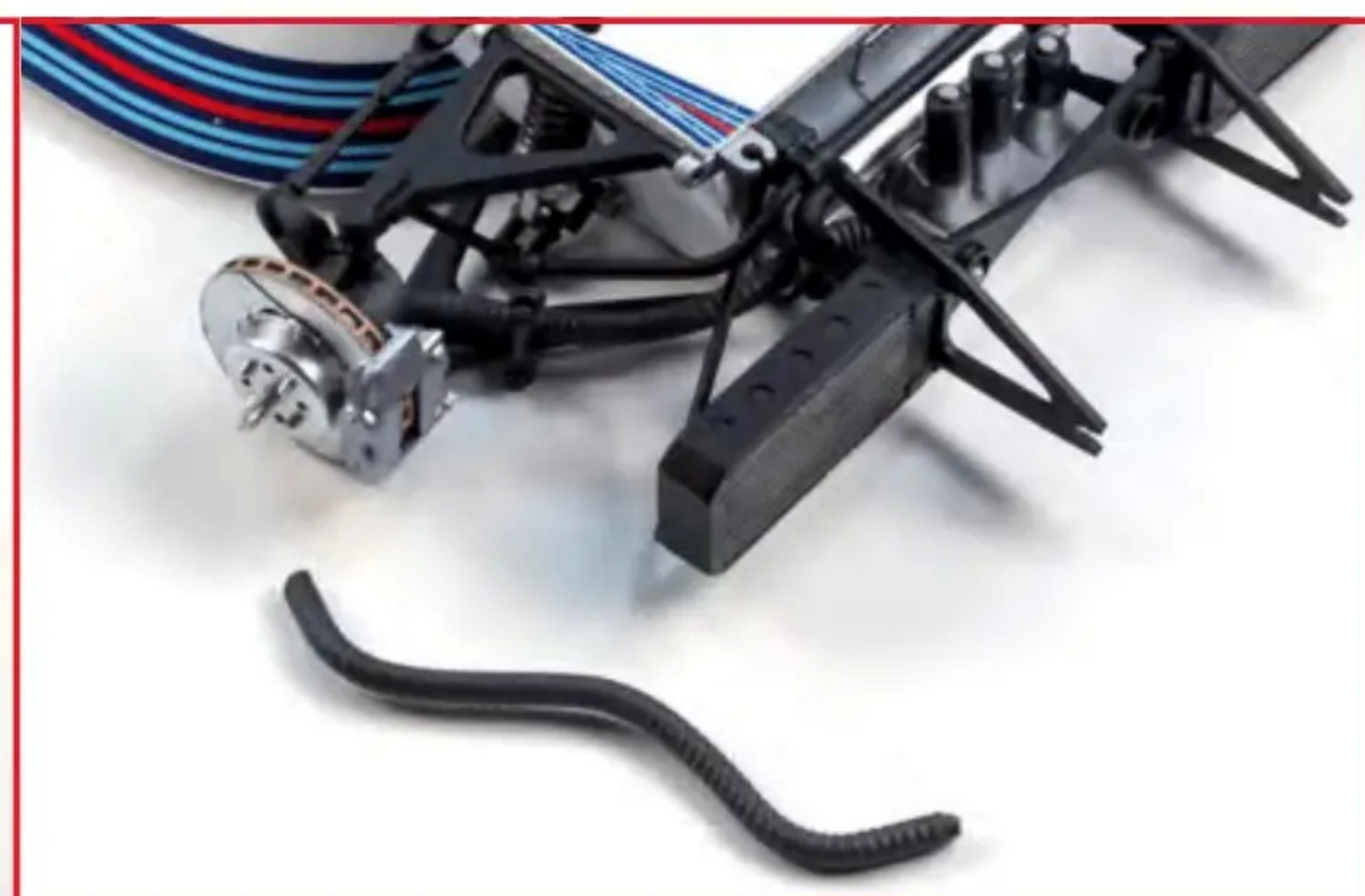
The kit does not provide brake ducts, which are a conspicuous part of the front end. I found this product with Model Factory Hiro, which uses pliable ribbed metal rods. Once the plastic sleeves are applied, gentle heat from a flame causes the plastic sleeve to shrink over the metal core. These were then bent and applied into position
