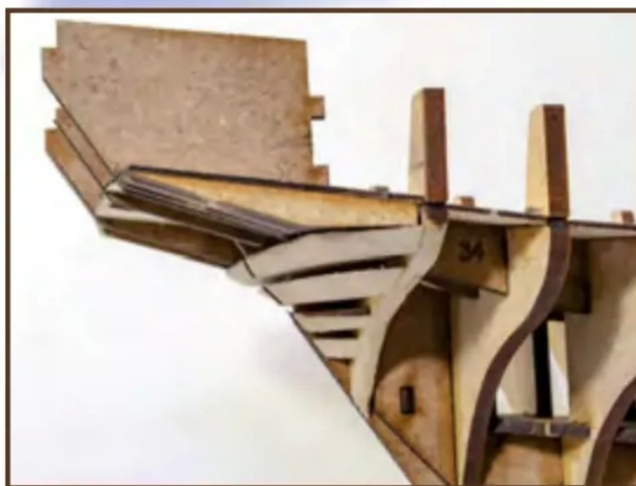
Some filler blocks are added to the stern, which will provide a base to plank to
