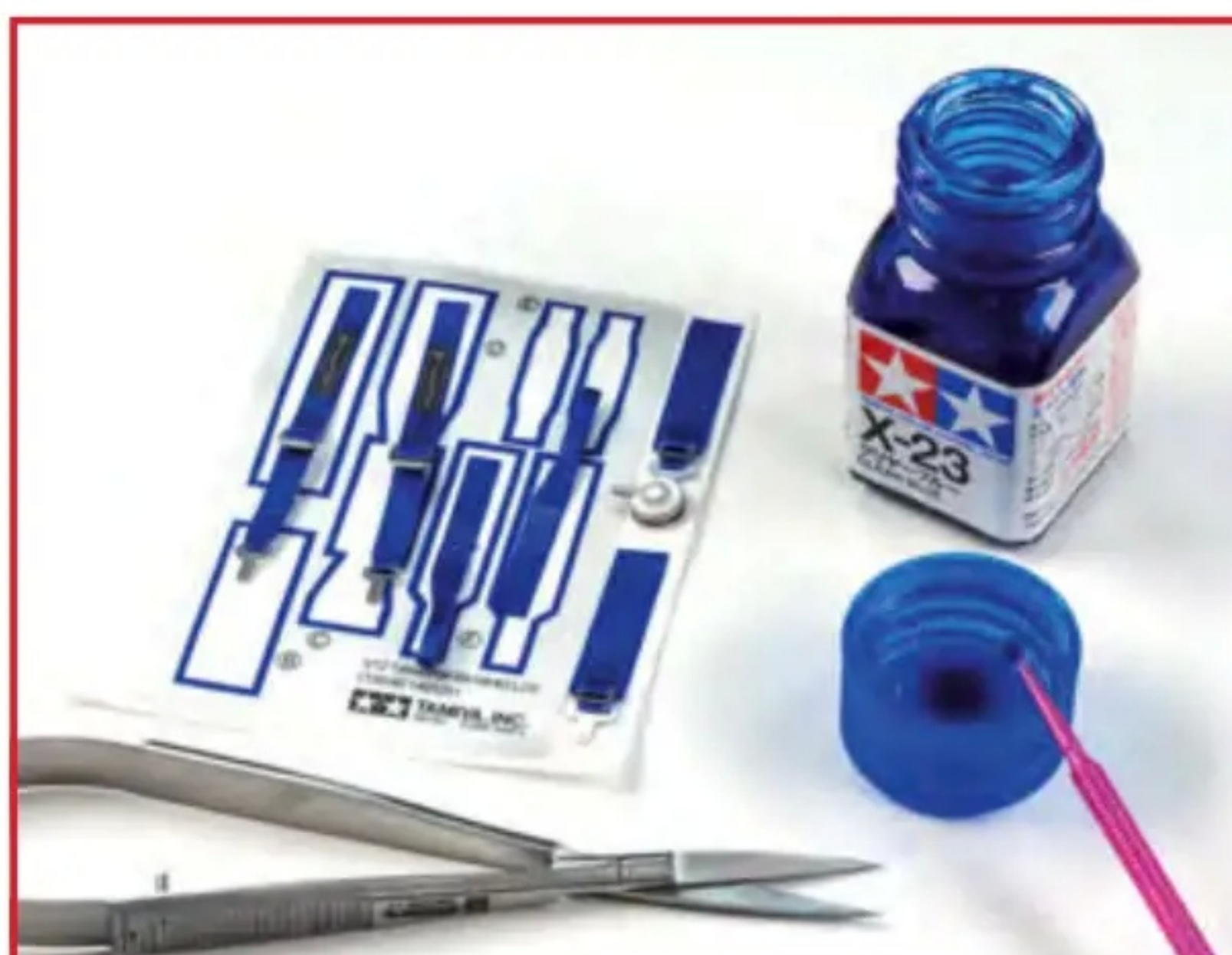
The kit provides lovely adhesive fabric seatbelts with PE hardware which requires some assembly. The edges of the fabric fray easily and have a white edge, so I solved both issues simultaneously by trimming the edges and sealing them with X-23 enamel paint
