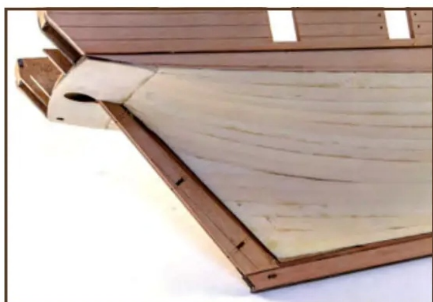
I can now fit the rudder post. You can also see how the planks run into the lower stern
