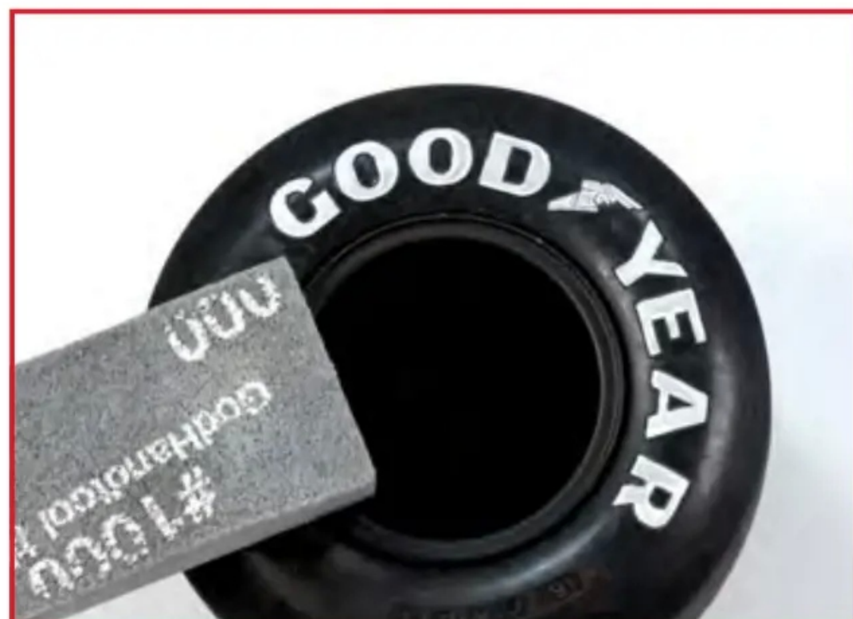
The Good Year logos required hand painting. I used Tamiya XF-2 and Tamiya acrylic paint retarder to help with flow and levelling. A 000 brush was required for the fine detail. After painting within the raised edges, I used a GodHand 1000 sanding block run gently over the raised edges to remove stray paint and increase definition
