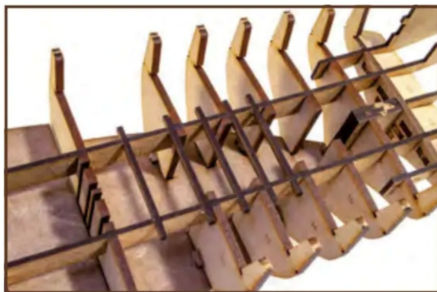
Two longitudinal beams now slot above the bulkheads, providing a base for the upper deck and these are supplemented by a number of cambered deck beams
