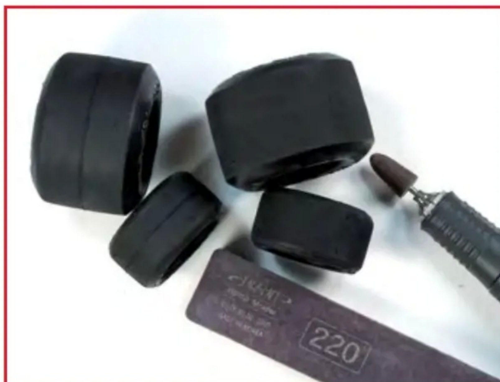
The rubber tyres contain a distinct mould seam, which needed to be removed. This was completed using a rotary abrasive rubber bullet followed by sanding under running water using an Infini soft sanding stick in 220 grit
