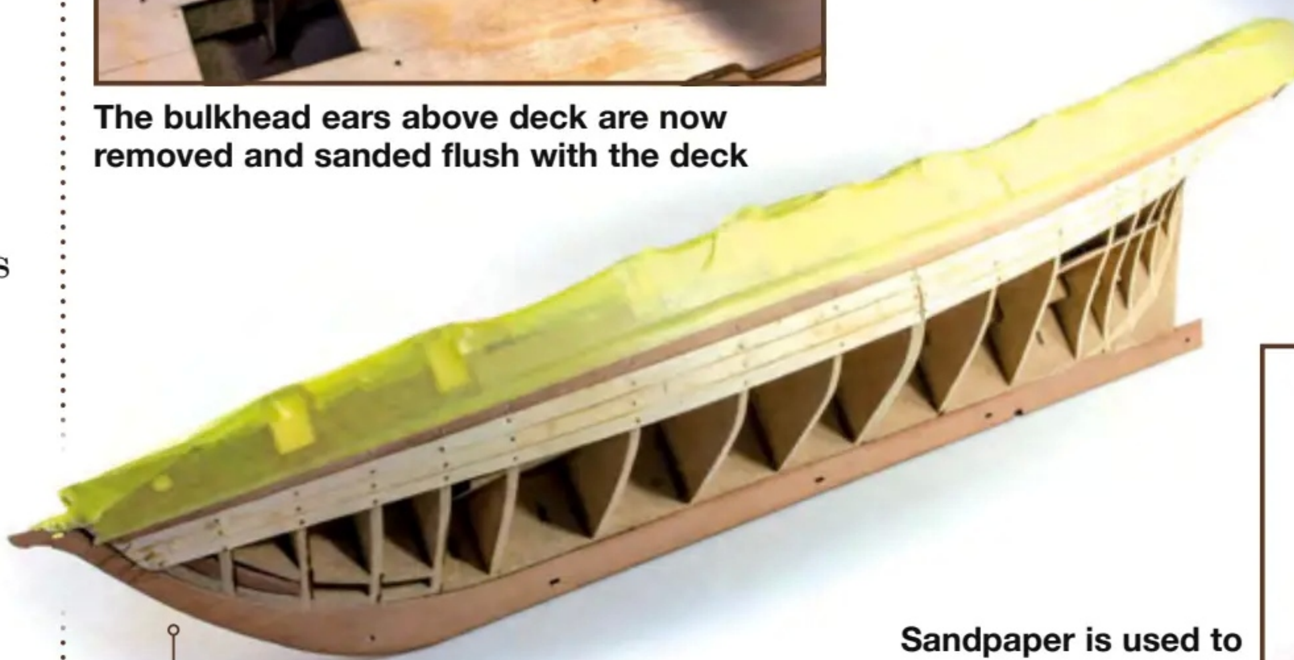
A laser-engraved limewood deck is now glued over the ply deck, hiding the remains of the MDF bulkheads
