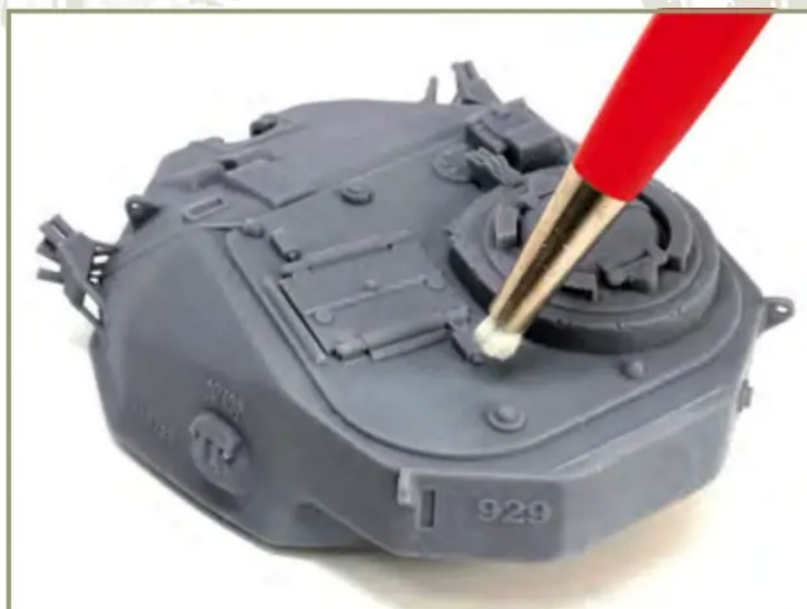
Any visible print lines on then upper turret were smoothed over using a fibreglass pen...
