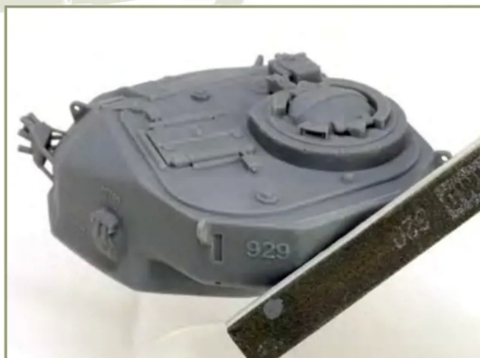
Unwanted remnants of the printing supports were cleaned away using a sanding stick
