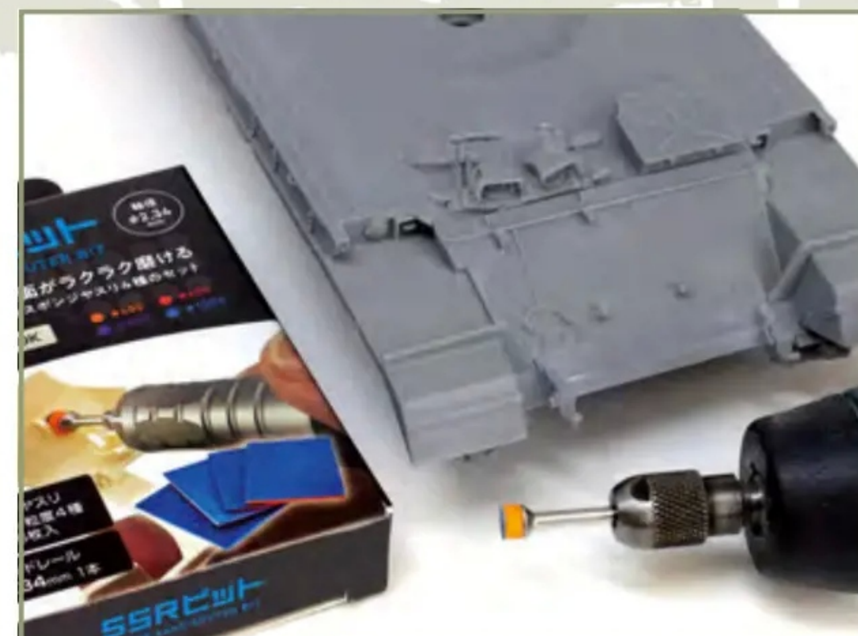
...and one of Argofile's 5mm sanding sponges mounted on their router bit
