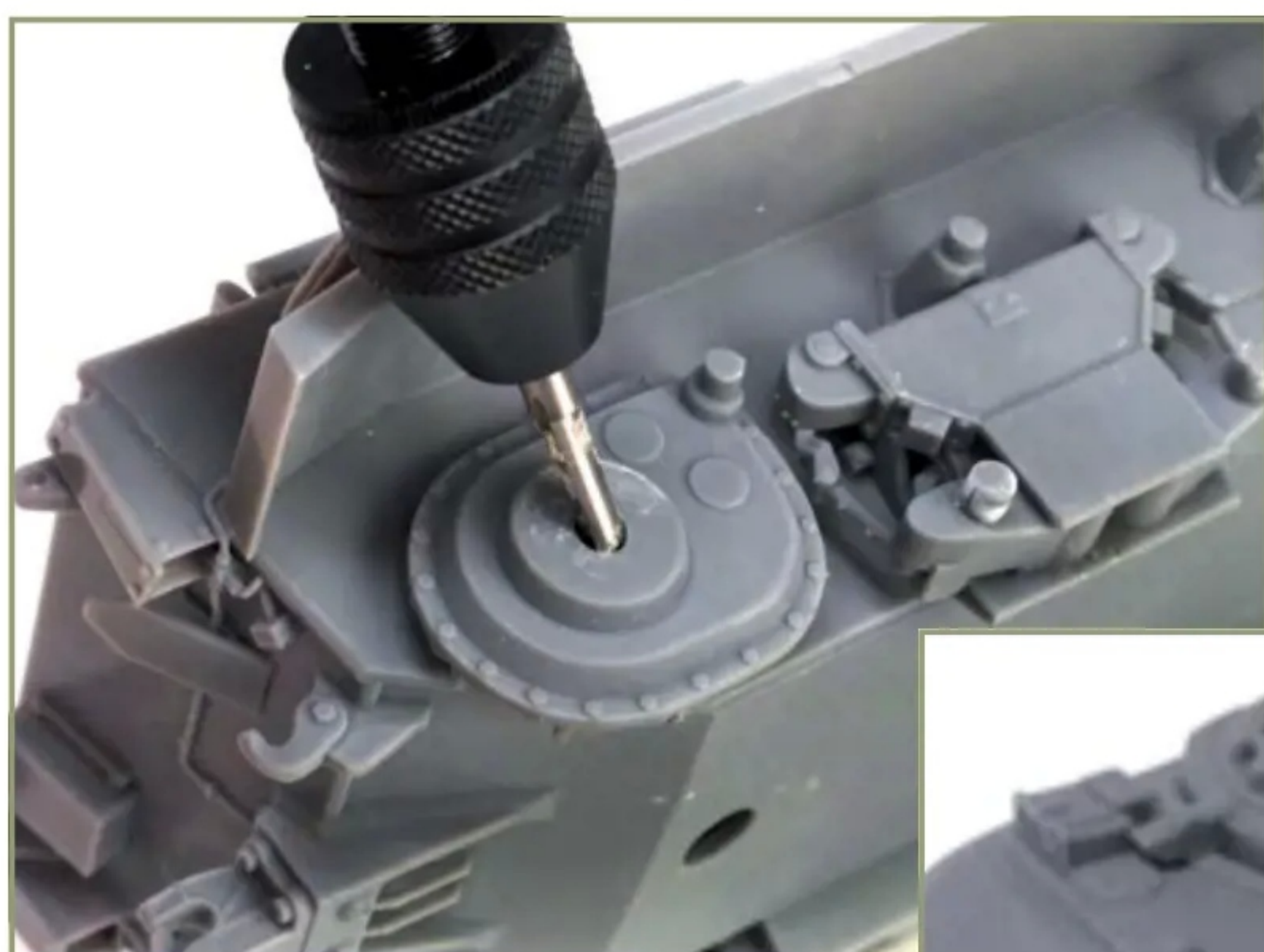
As with the tracks, the pin and socket joints for the wheels are virtually identical in size, so they don't slip together without using considerable force. A milling bit was used to ream out the holes for the sprockets and then each of the roadwheels, until they slipped together with ease
