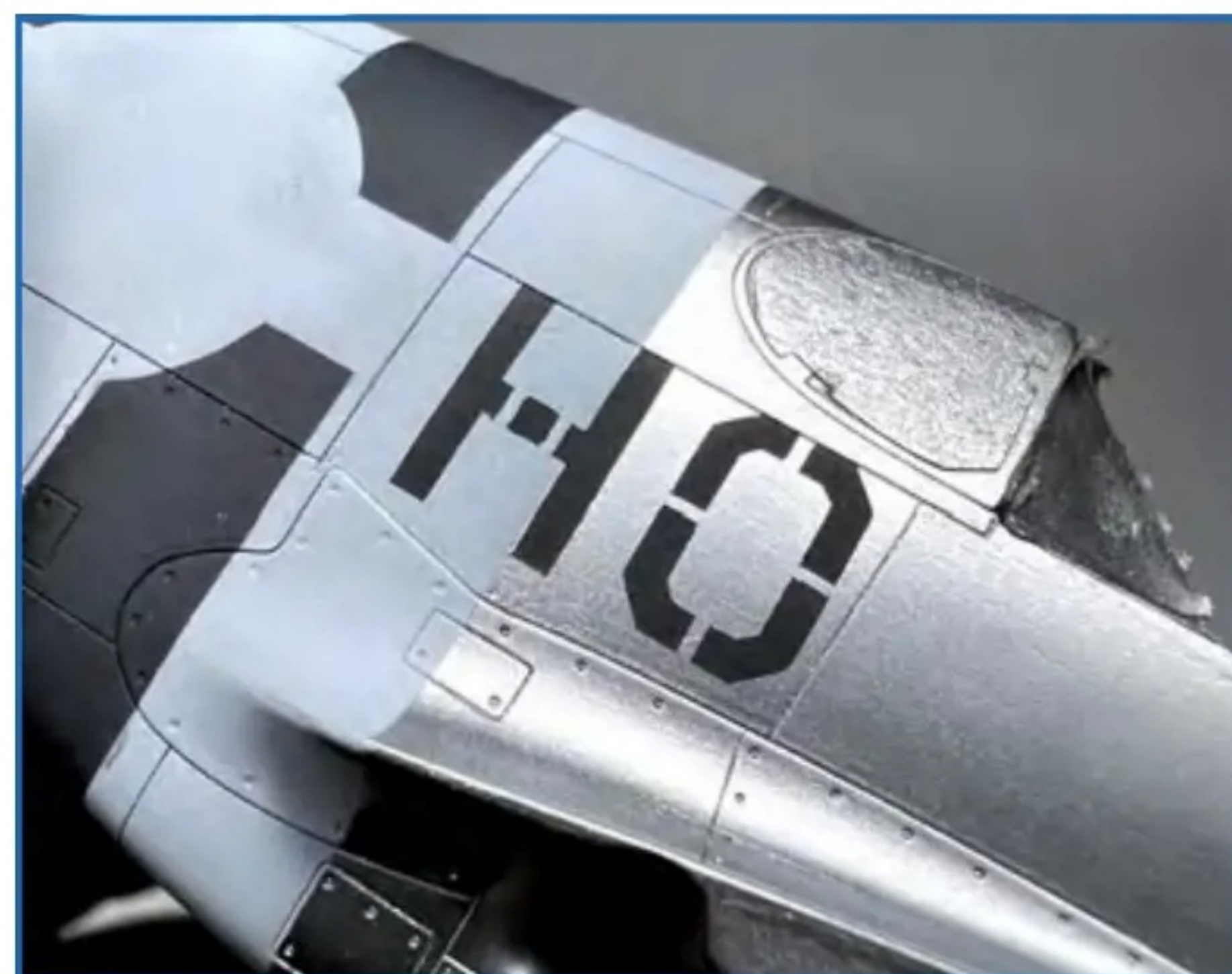
While the finished result is not perfect, there's no substitute for painted markings on a natural metal finish, where decal edges can stand out like a sore thumb
