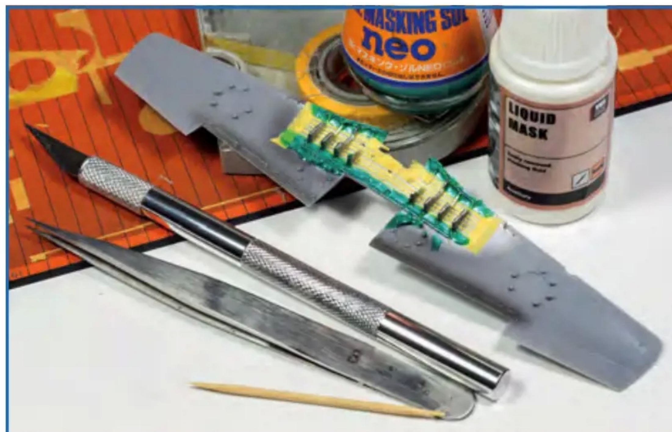
Effective masking takes a variety of materials — tape for sharp, straight lines, low viscosity masking fluid for sealing any gaps and high viscosity for wider coverage
