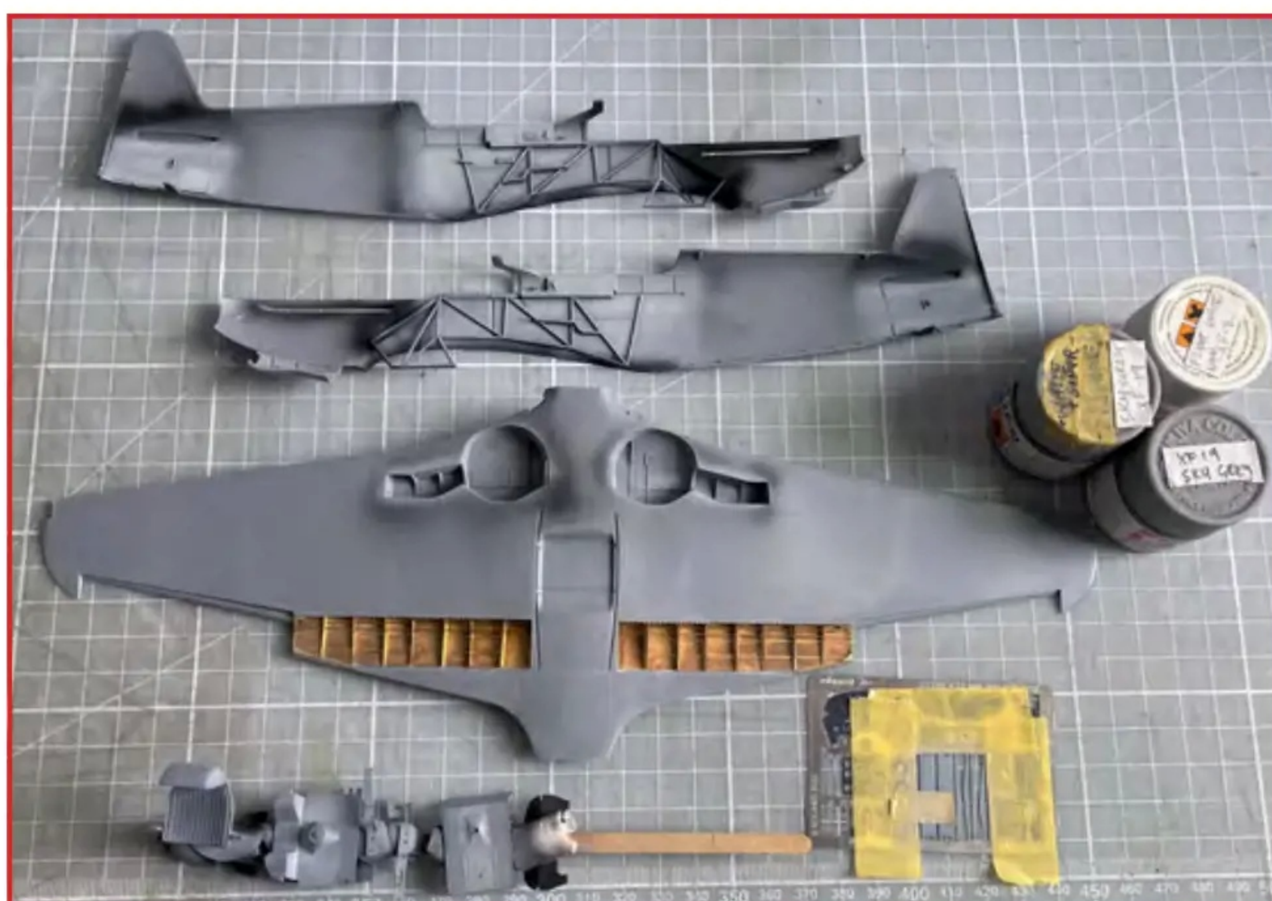
Paint time! The interior areas to be painted were first primed with Mr Surfacer 1500 Black. This will help create shadow areas in the next step. A lightened mix of XF-19 Sky Grey was then sprayed on the interior surfaces. This was done in light passes from above, letting the black undercoat create contrasting shadow areas
