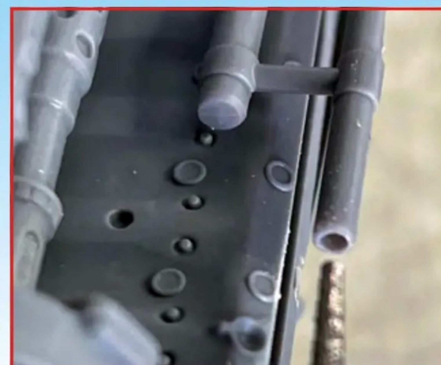
Before fitting the engine cowling, I bored out the tip of the machine gun tip. This low-powered USB rechargeable mini drill is ideal because it doesn't melt the plastic
