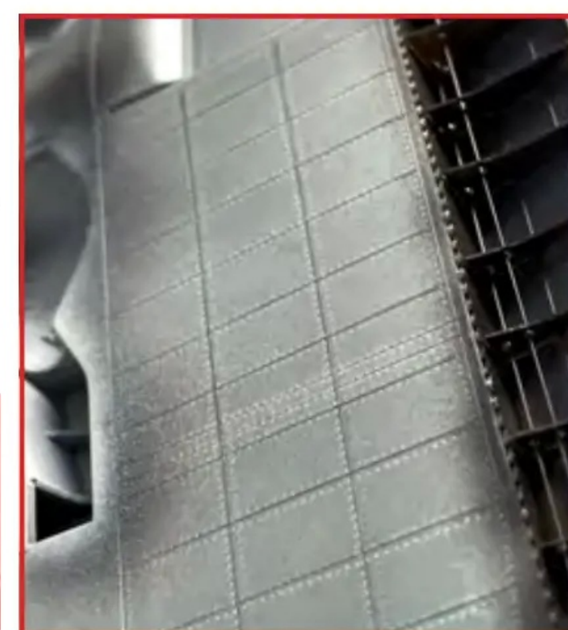
The surface of the kit has nicely engraved panel lines and subtle fabric textures, but no rivet detail. Using my RB riveter and a set of plans I found on the internet, I set about adding rows of rivets with the pounce wheel
