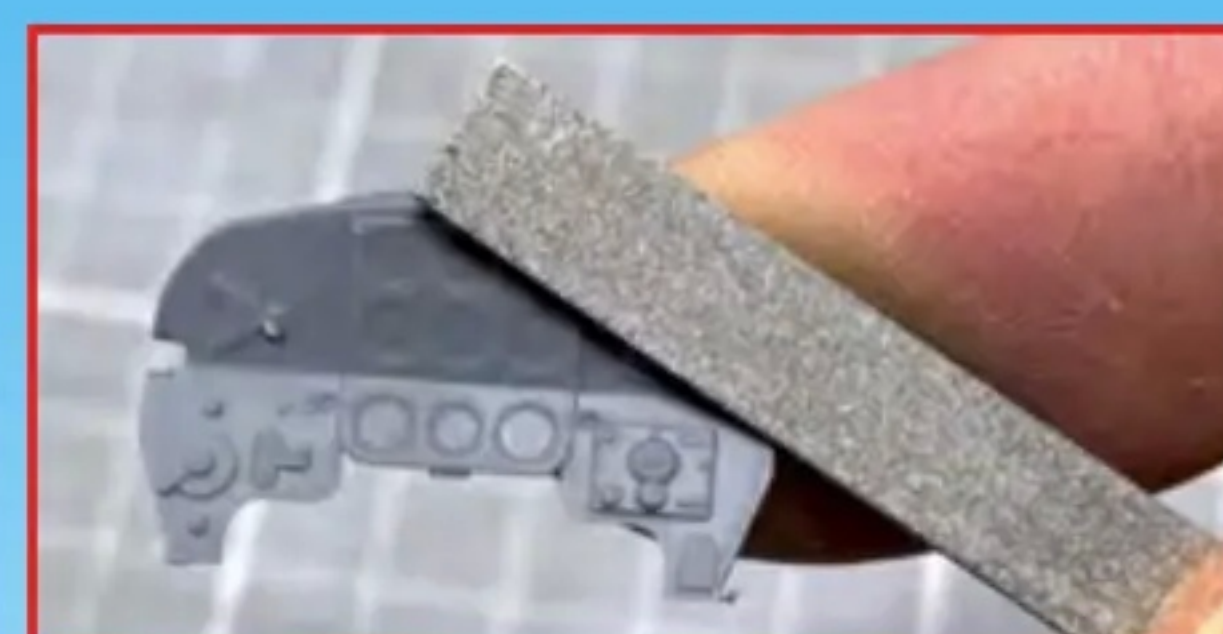
Before starting to paint, the cockpit dial details were sanded off in preparation for the printed PE detail to be glued on
