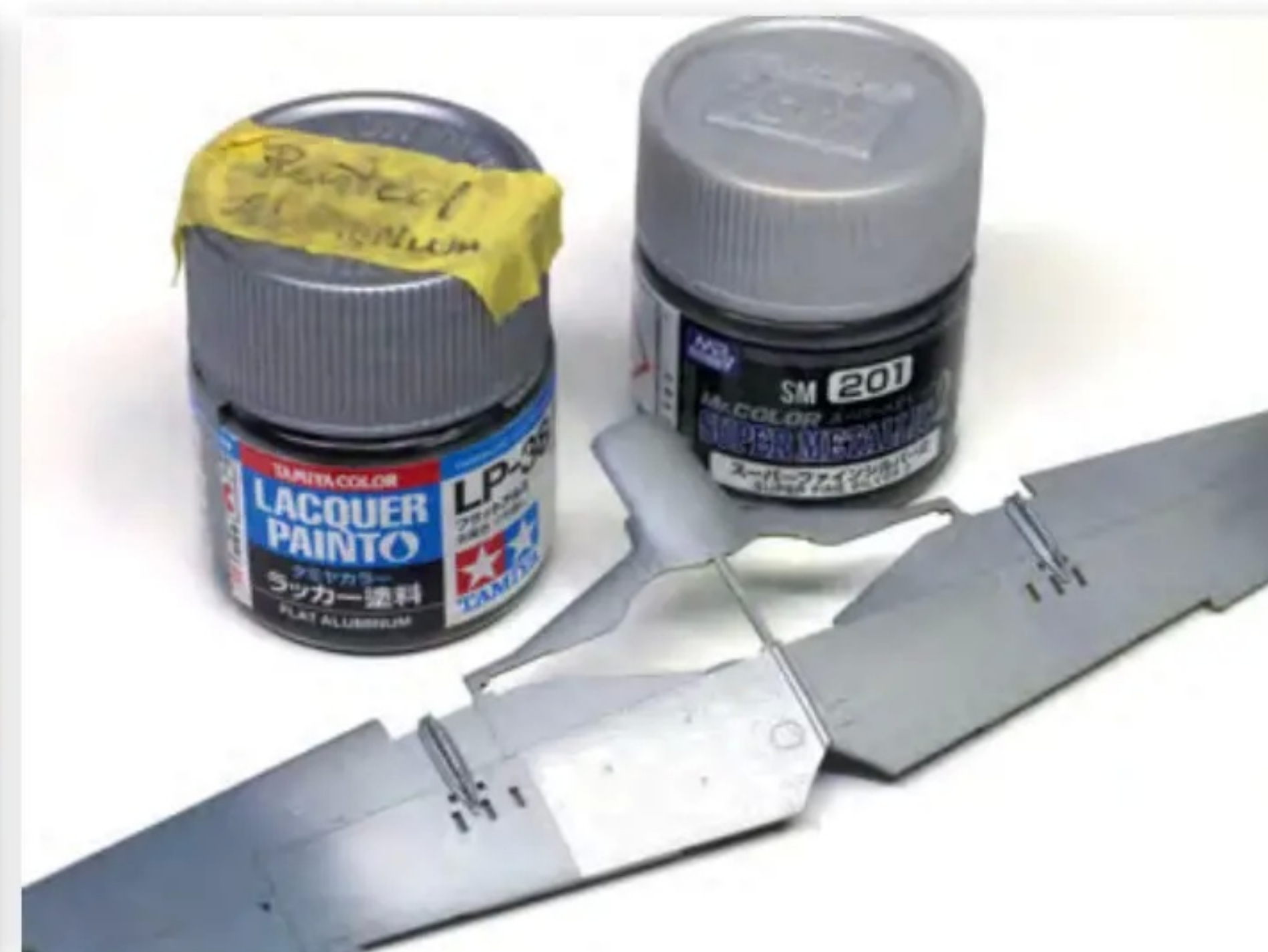
As usual, I pre-finished around openings with layers of paint that would cut down on my need to mask them off, later on. Here, the lower wing has been prepared using my mixed aluminium paint (Tamiya LP-38 Flat Aluminium, mixed with Mr Hobby Light Aircraft Grey), followed by panelling, airbrushed with a layer of Mr. Super Metallic Super Fine Silver 2
