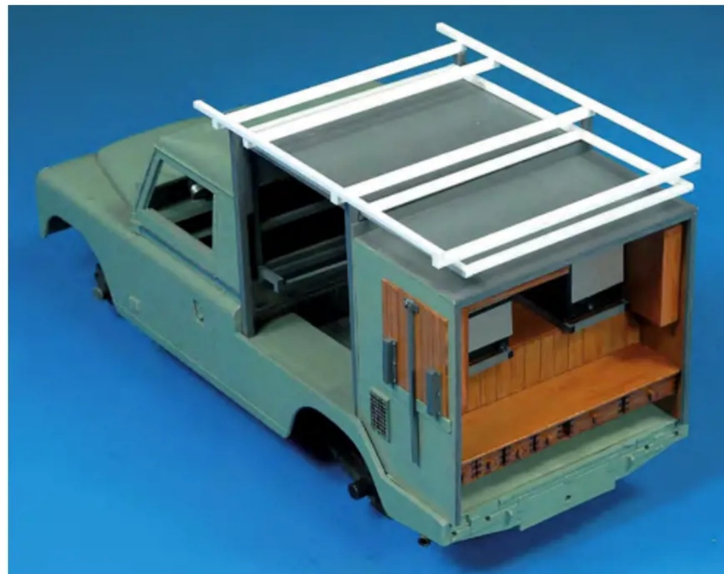
The upper stowage rack and lower rack for the weather protection tarp were built from 0.080" and 0.060" square rod respectively
