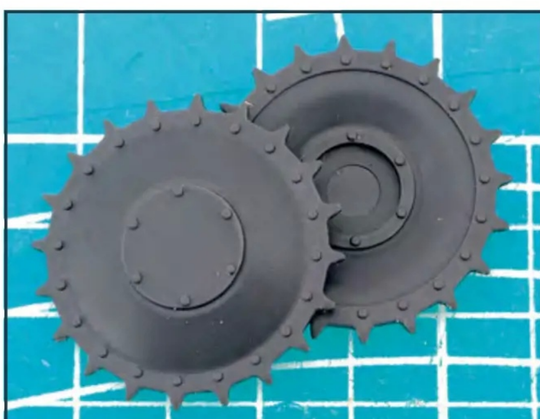
A simple stub-axle is cemented into the circular recess in the back of each sprocket. The axle then pushes into its conical housing, secured by a previously-installed polycap
