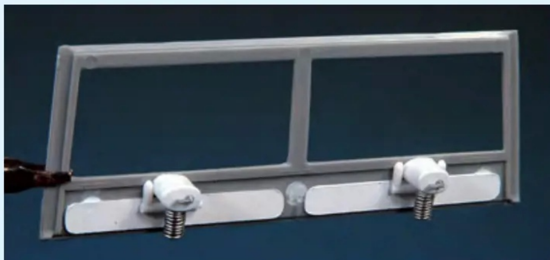
Wiper motors were added to the inside of the windscreen assembly
