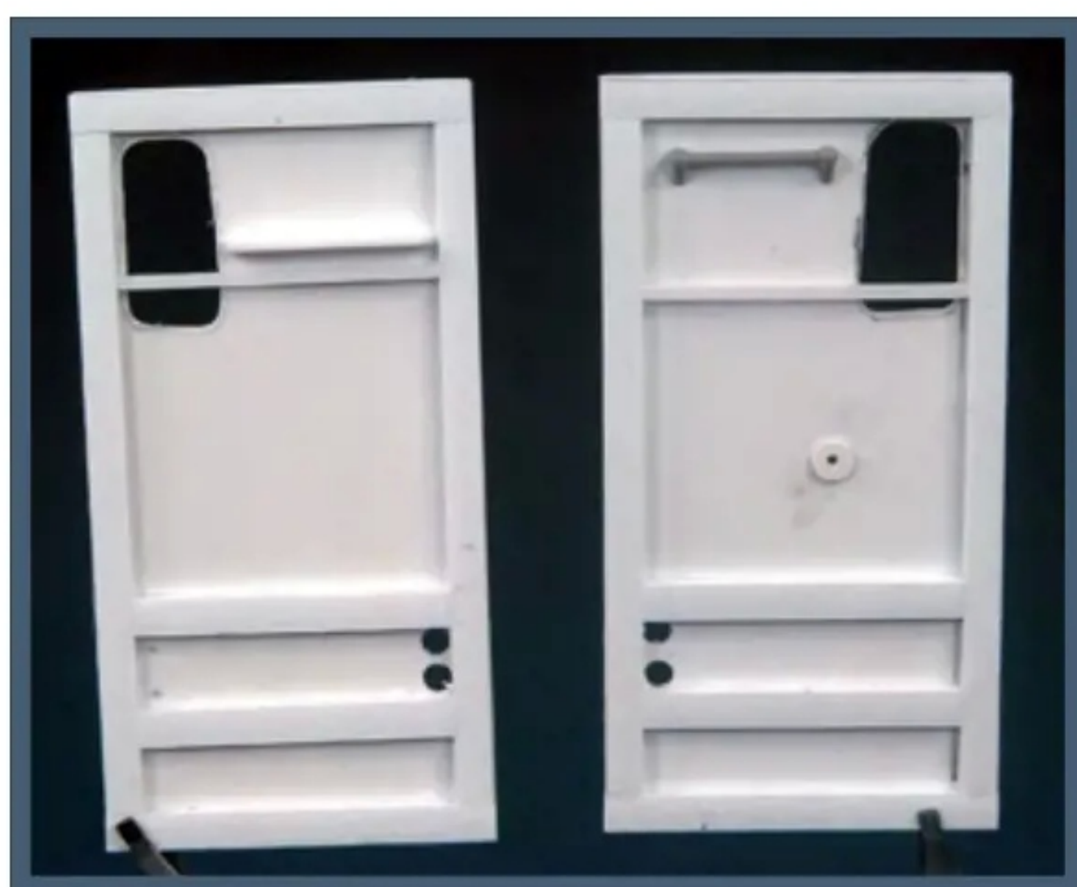
The two large rear doors were fabricated from strip and sheet, and holes cut out for the Land Rover shaped windows
