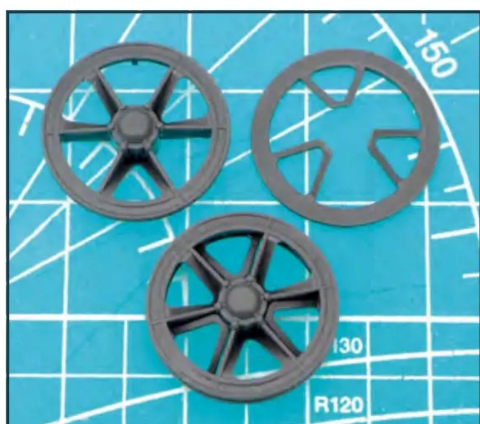
The track idler wheels assemble from two halves, perfectly recreating the complex design of the real idlers
