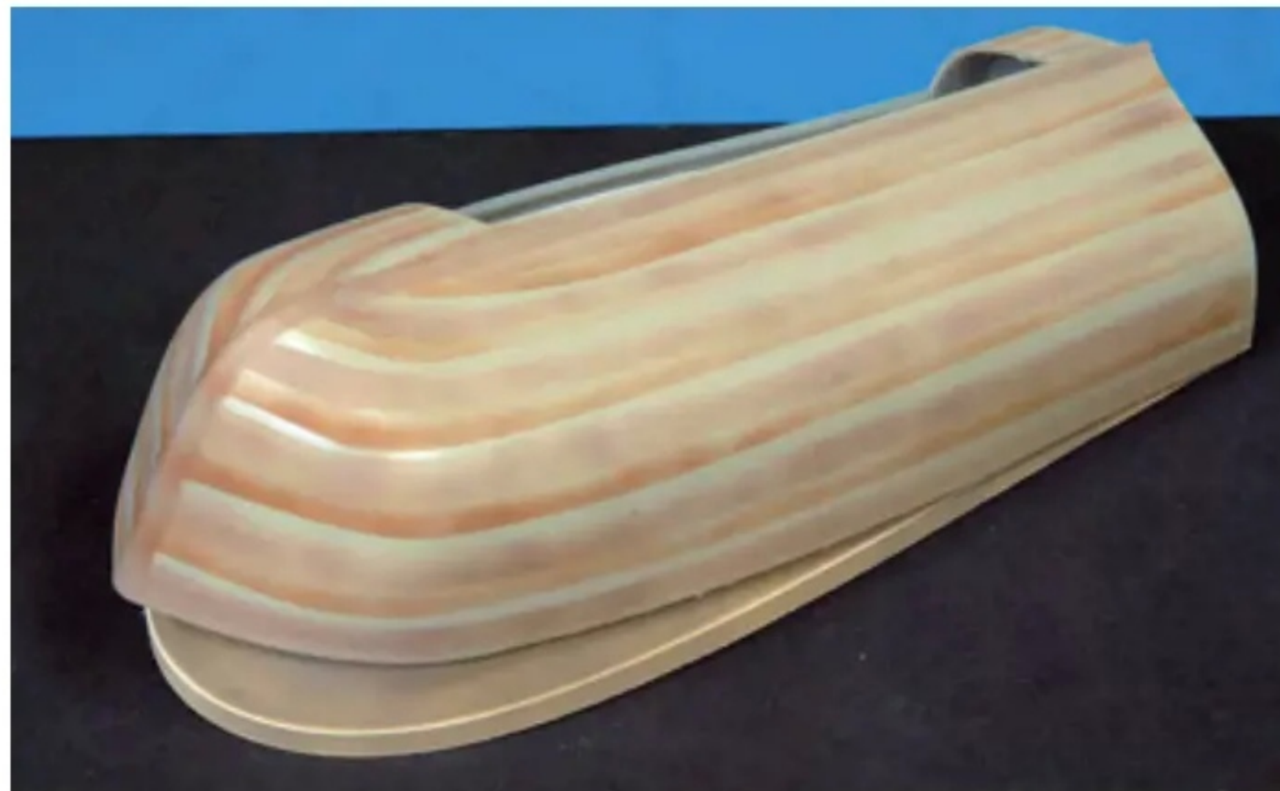
To make the smooth surface of the boat appear like planks, several lines of different tan and brown colours were airbrushed using strips of masking tape
