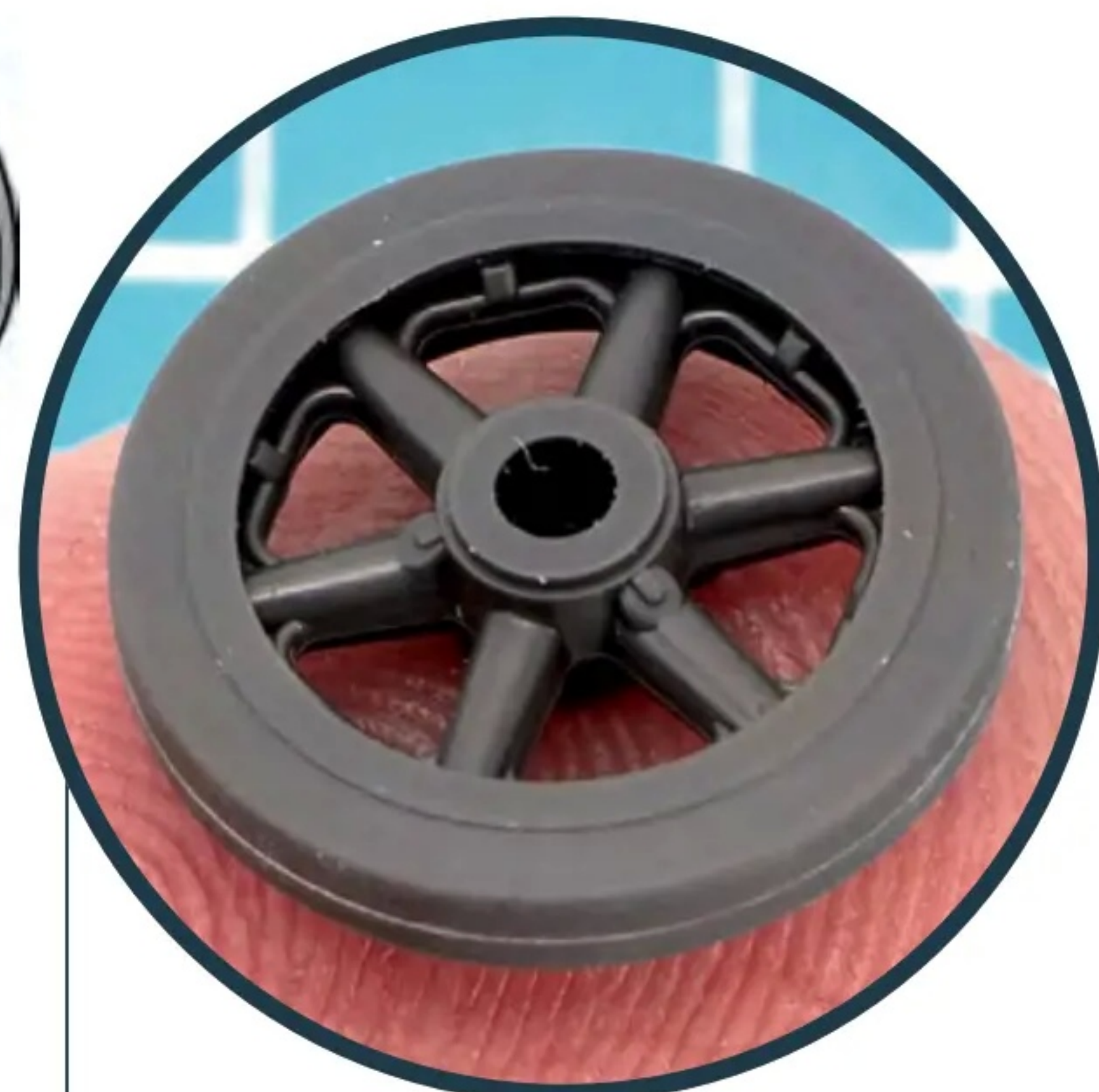
The result is a highly accurate depiction of the running wheels, complete with recesses behind the outer rims as per the real things
