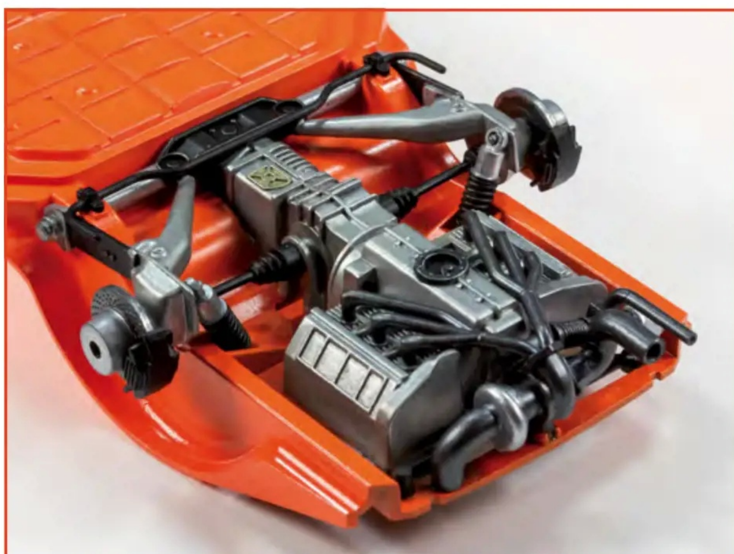
The rear axles and suspension parts installed
