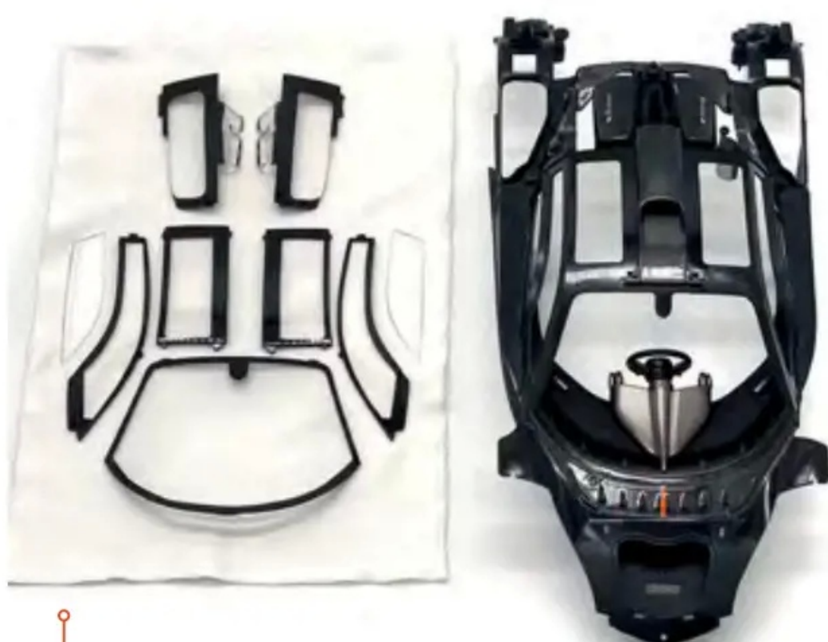
Templates were cut from masking tape so the edges of the clear parts could be painted
