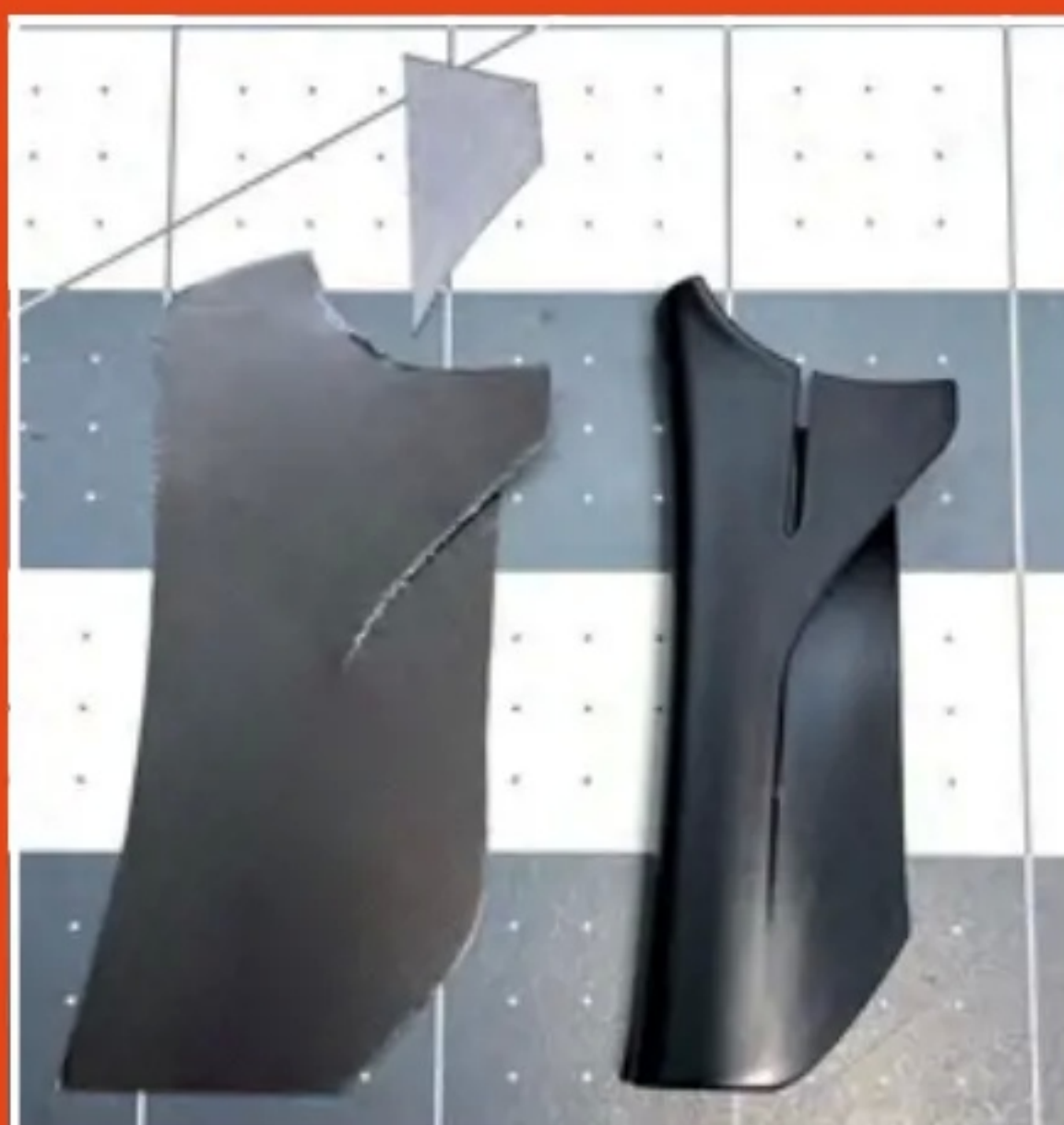
The doors also are seen having templates cut, the kit part primed, painted and carbon-fibre decals applied, finished off with a clear coat
