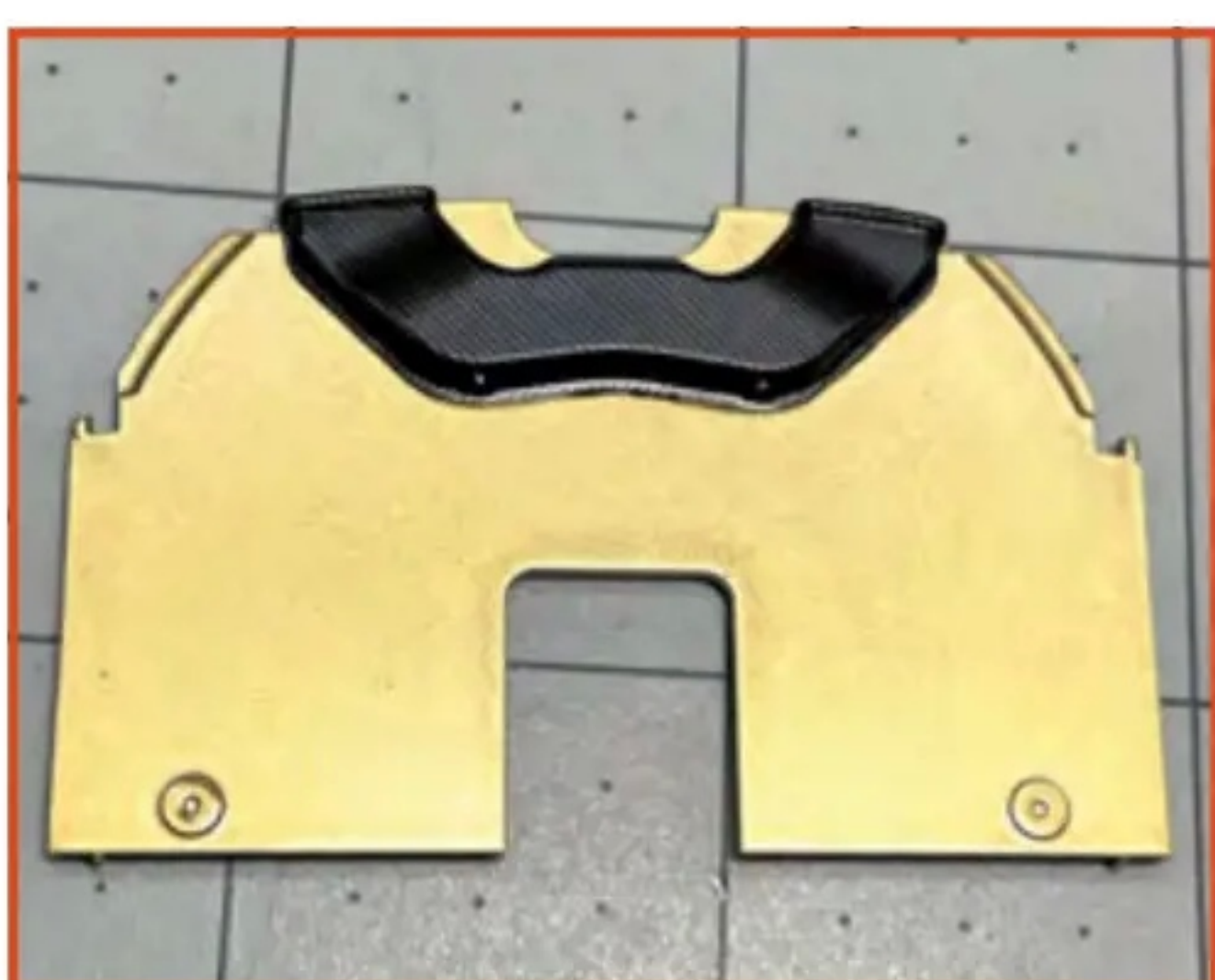
Here we see the attachment of the firewall and air duct to the central tub before gluing in the seats
