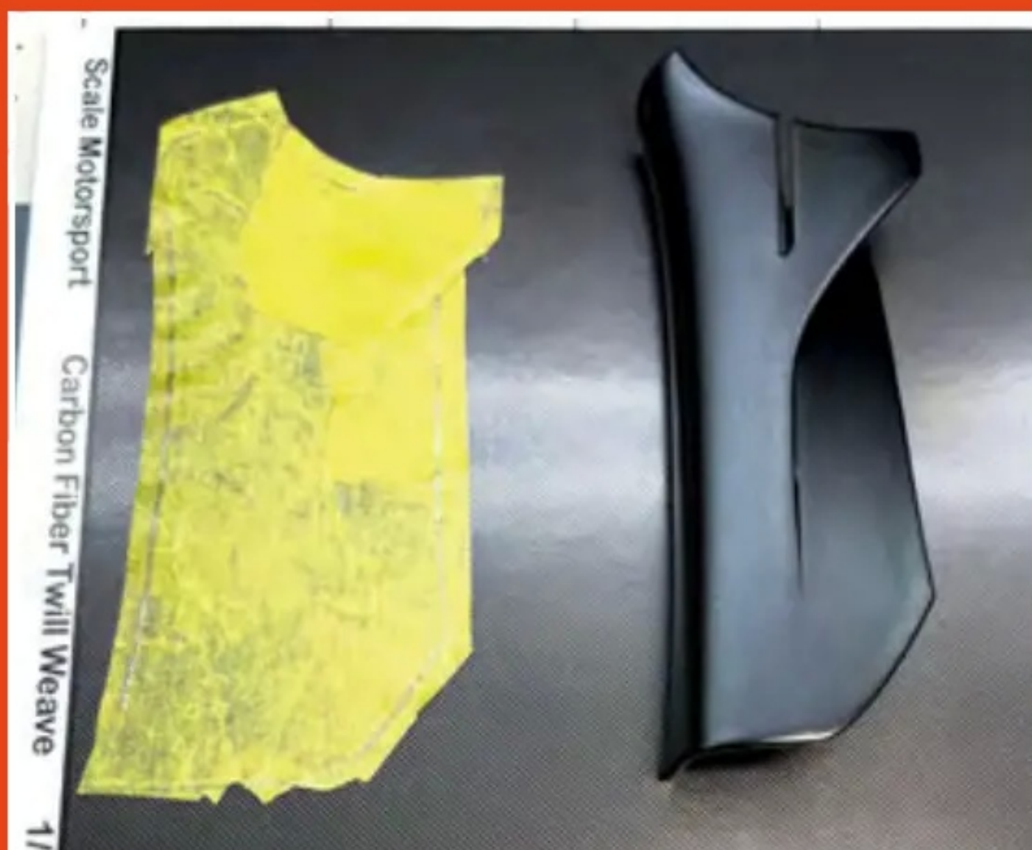
The doors also are seen having templates cut, the kit part primed, painted and carbon-fibre decals applied, finished off with a clear coat
