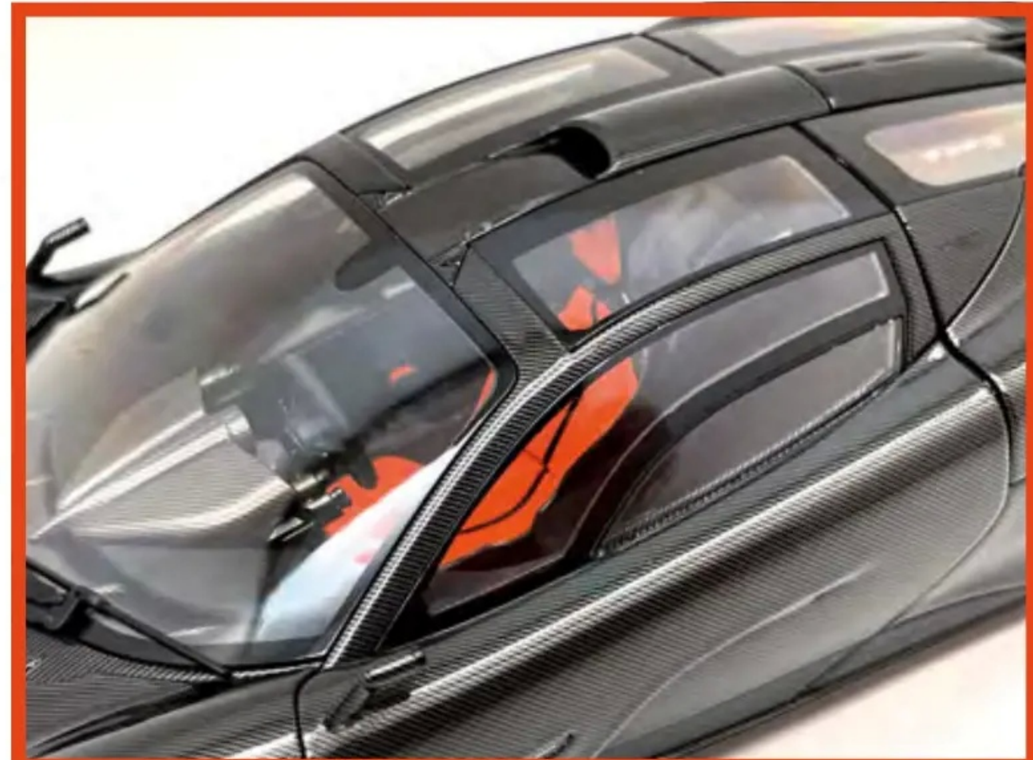
Templates were cut from masking tape so the edges of the clear parts could be painted
