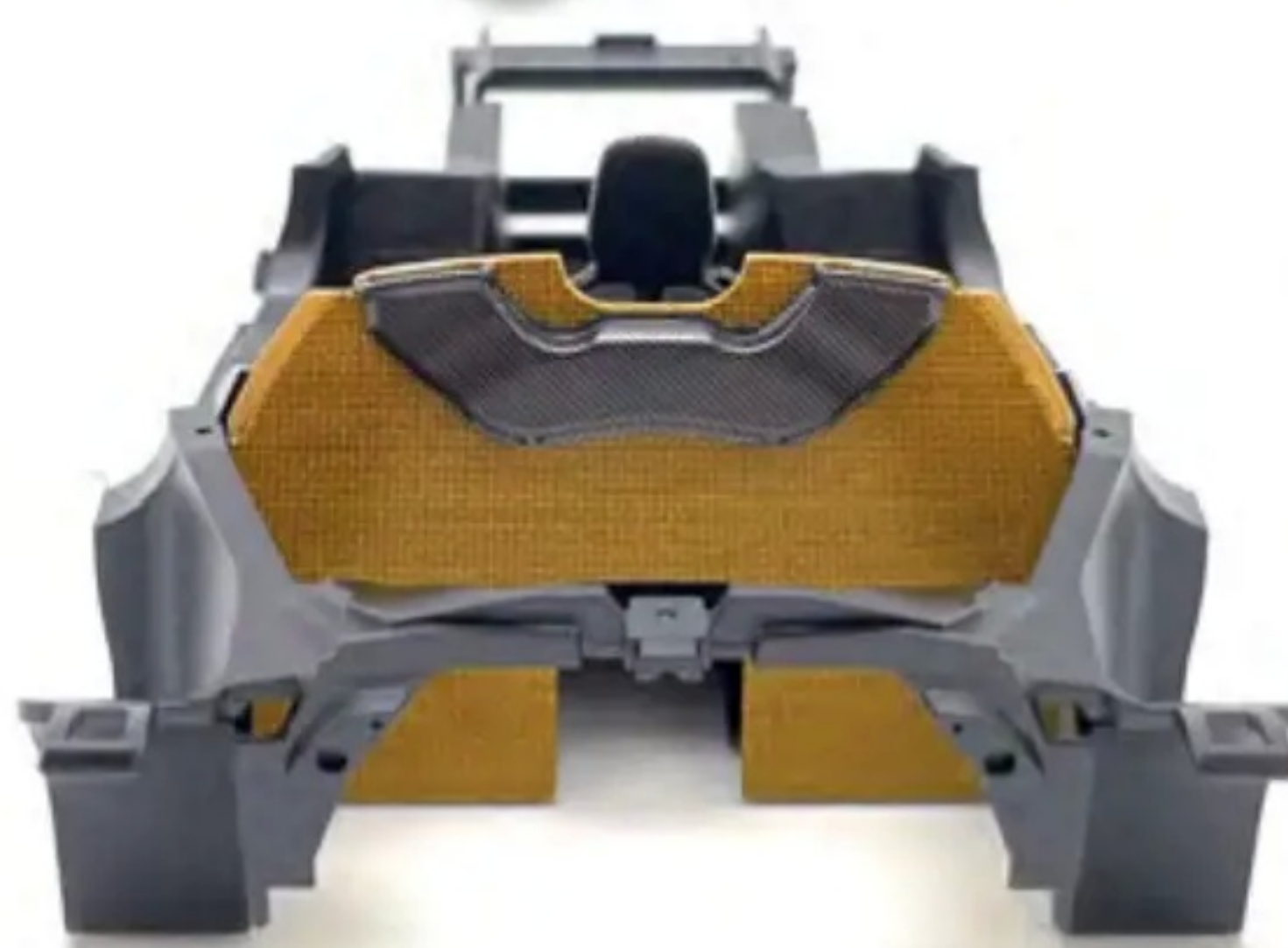
Here we see the attachment of the firewall and air duct to the central tub before gluing in the seats
