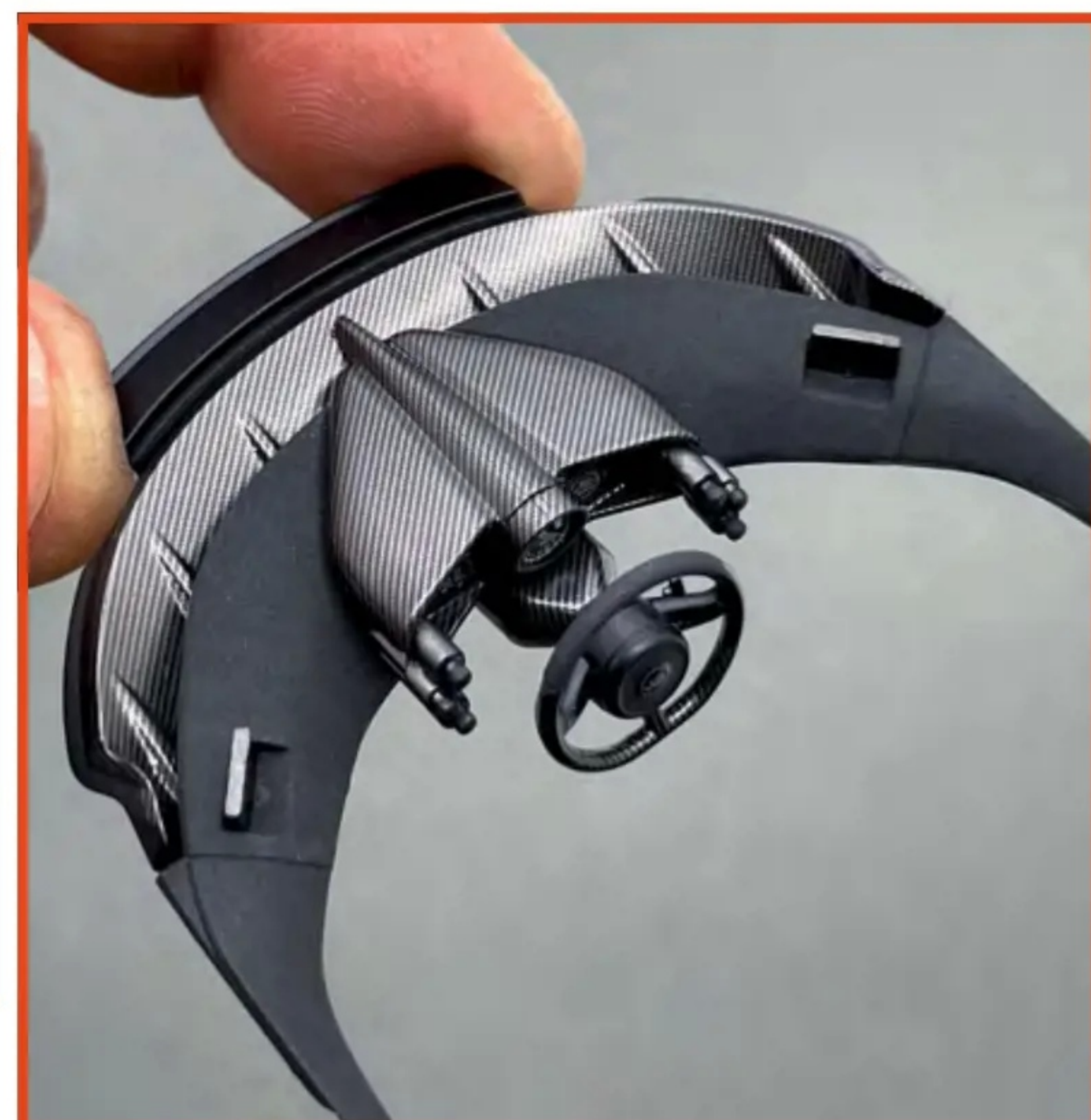
The dash panel complete after carbon-fibre decalling and textured paint. Clear gloss was applied over the dials
