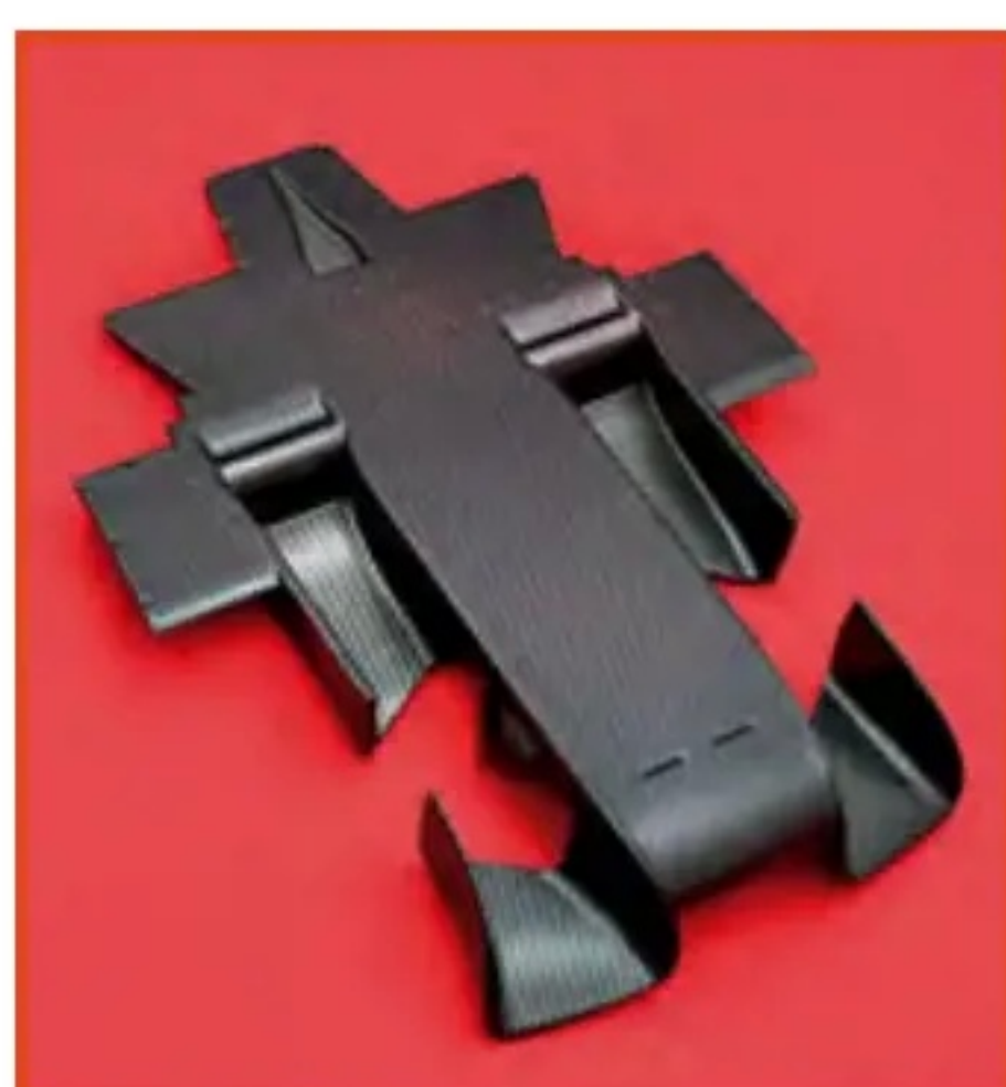
Here we see the attachment of the firewall and air duct to the central tub before gluing in the seats
