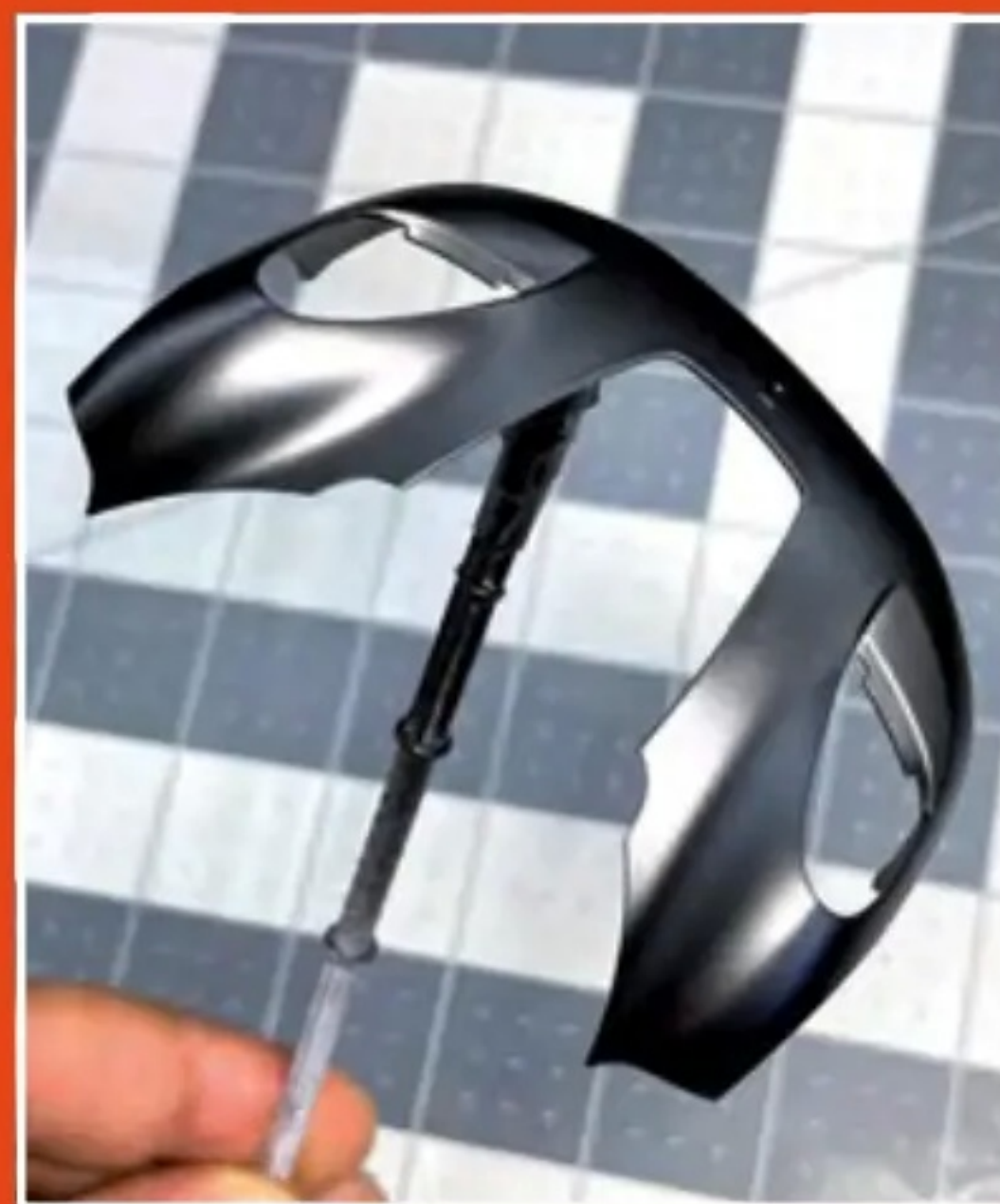
Here we see the nose of the car and the creation of the template, then a coat of Semi Gloss Black and the application of carbon-fibre decals
