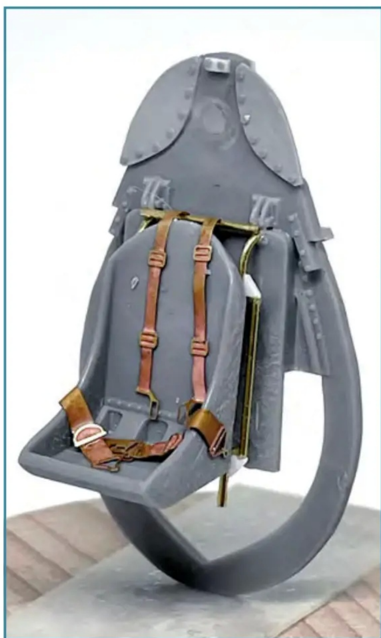
Photo-etched brass seat harnesses were fitted to the pilot's seat. The cockpit was initially paint Dull Dark Green, so Mr Color's Dark Green was used as the base colour
