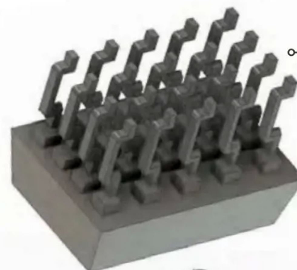
Having taught myself some basic CAD a couple of years back and buying a Phrozen Sonic Mini 8K printer not long after, I put both to use to make some smaller parts that I needed multiple copies of. These are tie down loops found on British vehicles such as the Centurion and Chieftain
