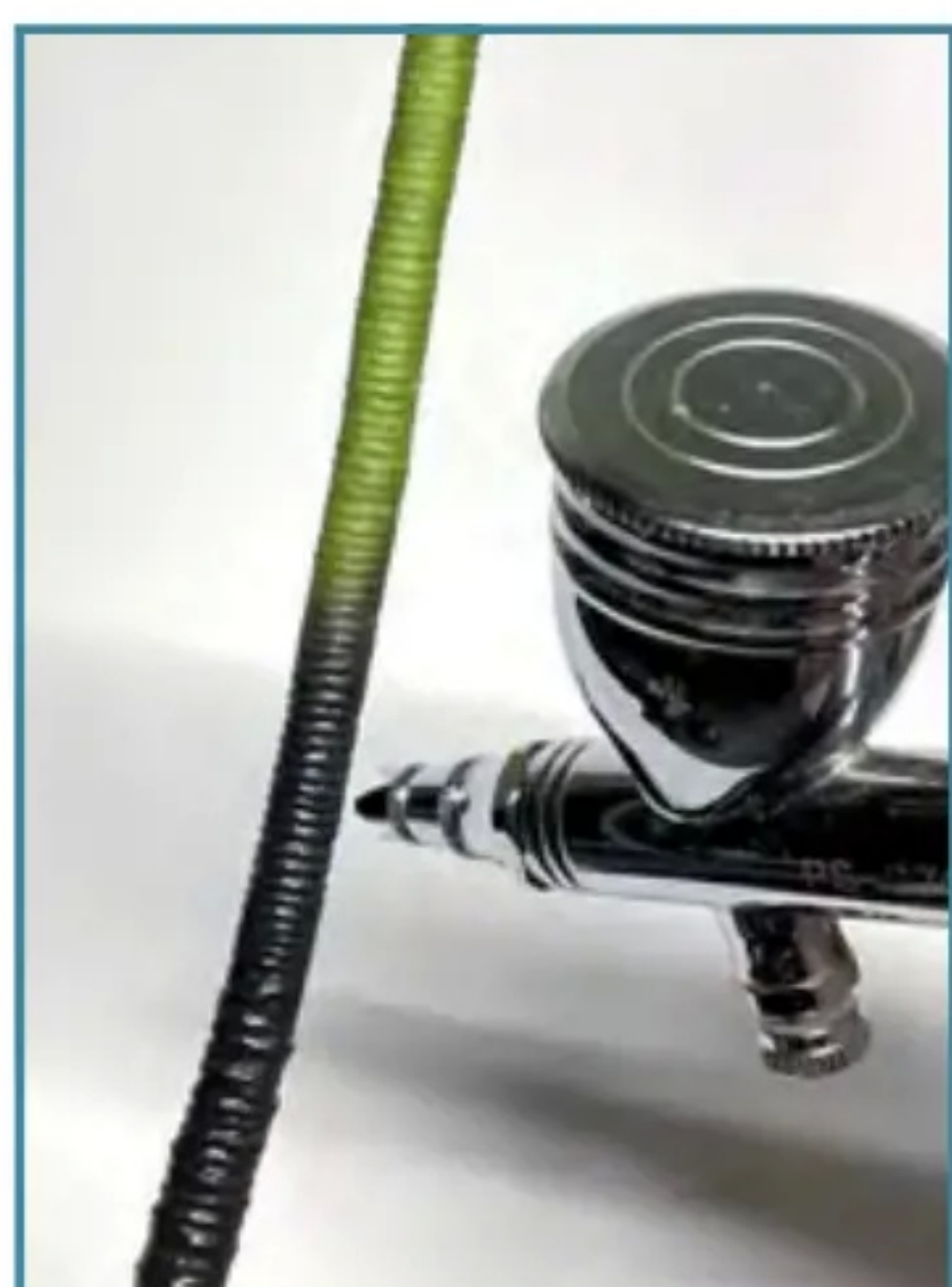
I sprayed black primer first, and then lightly airbrushed Tamiya XF-12 Light Grey at an angle
