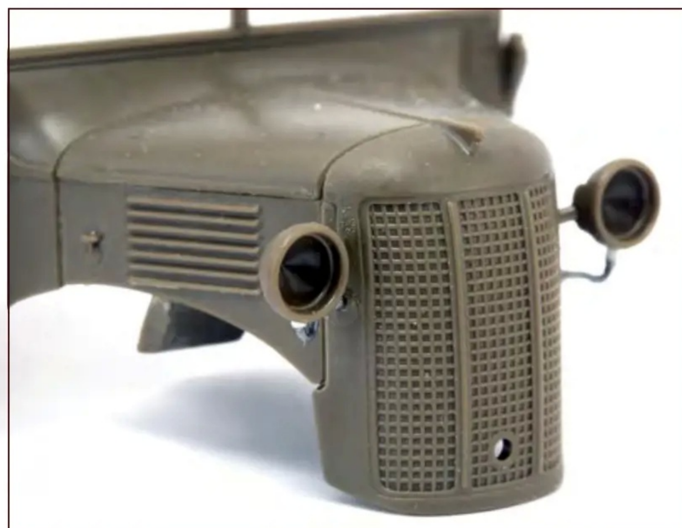
The headlights were given power cables and later, the lenses were replaced with foil-backed, clear resin items
