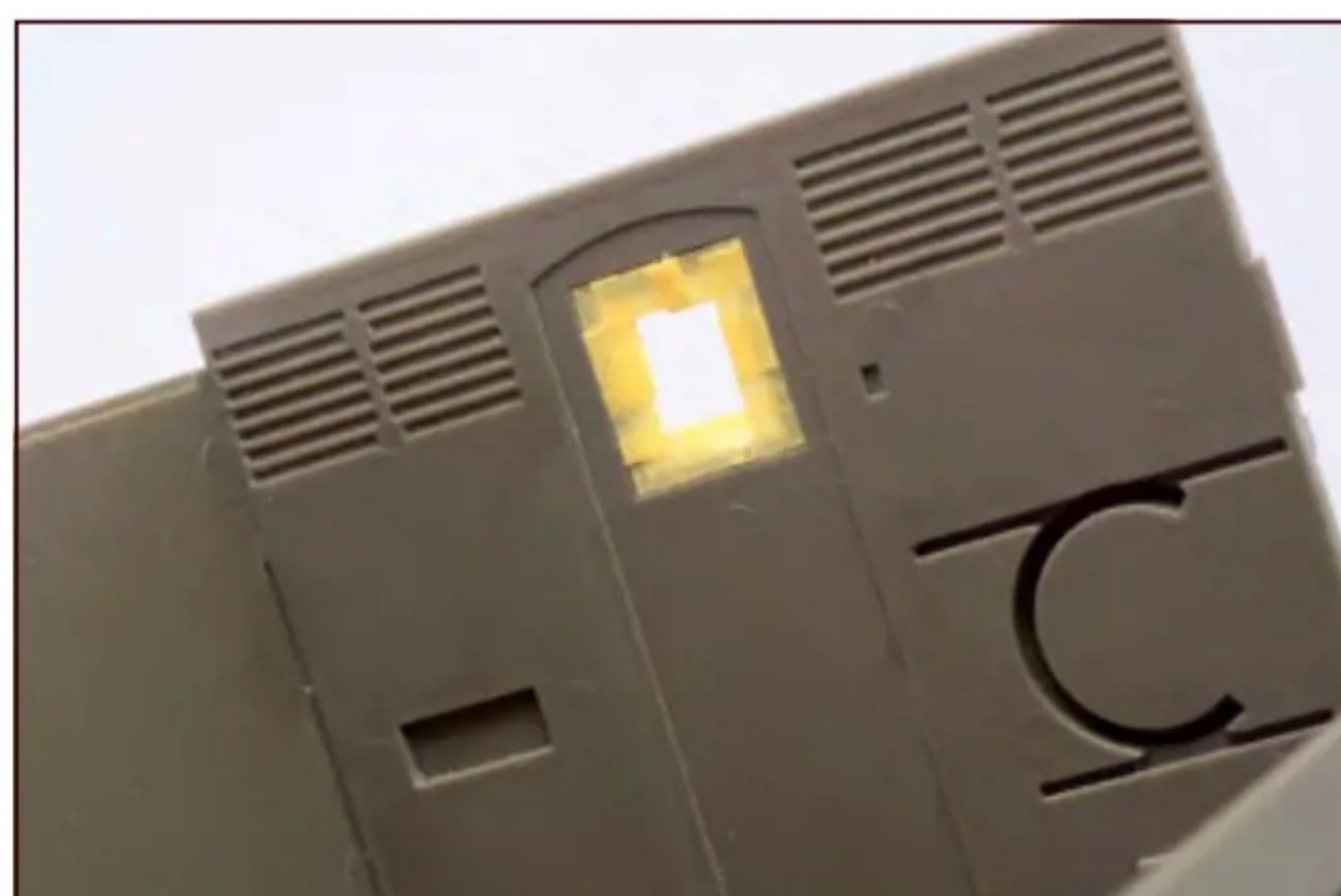
To allow the cabin's internal window to be easily cemented later on, the frame was masked off with tape to keep it clear of paint
