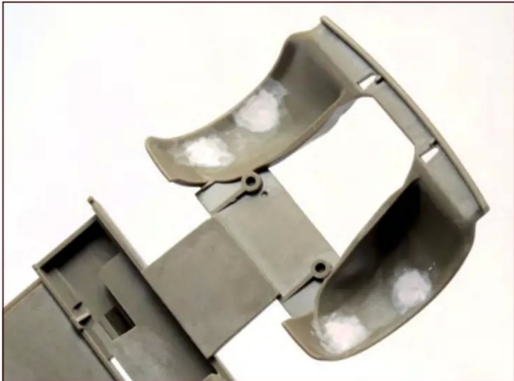
Although largely hidden when the body is mated to the chassis, the four big ejector-pin marks under the wings just had to be filled and sanded
