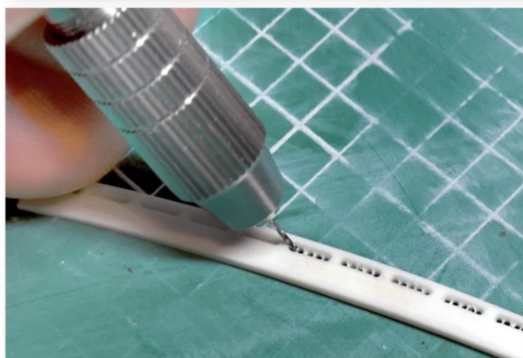
Opening up the rear vent panel that sits above the rear window. Mesh will be placed to the rear of the vent at a later point
