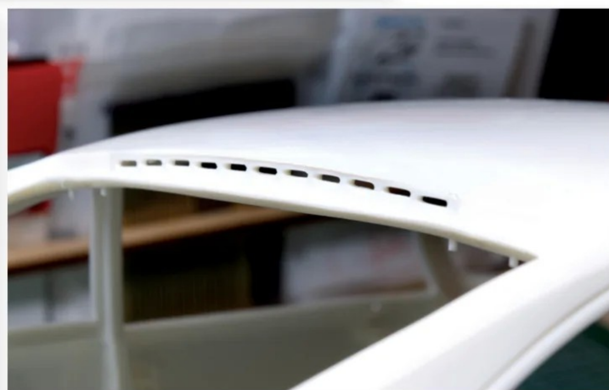
Now the vent panel is in place, the edges will be filled and sealed in giving a more uniform finish
