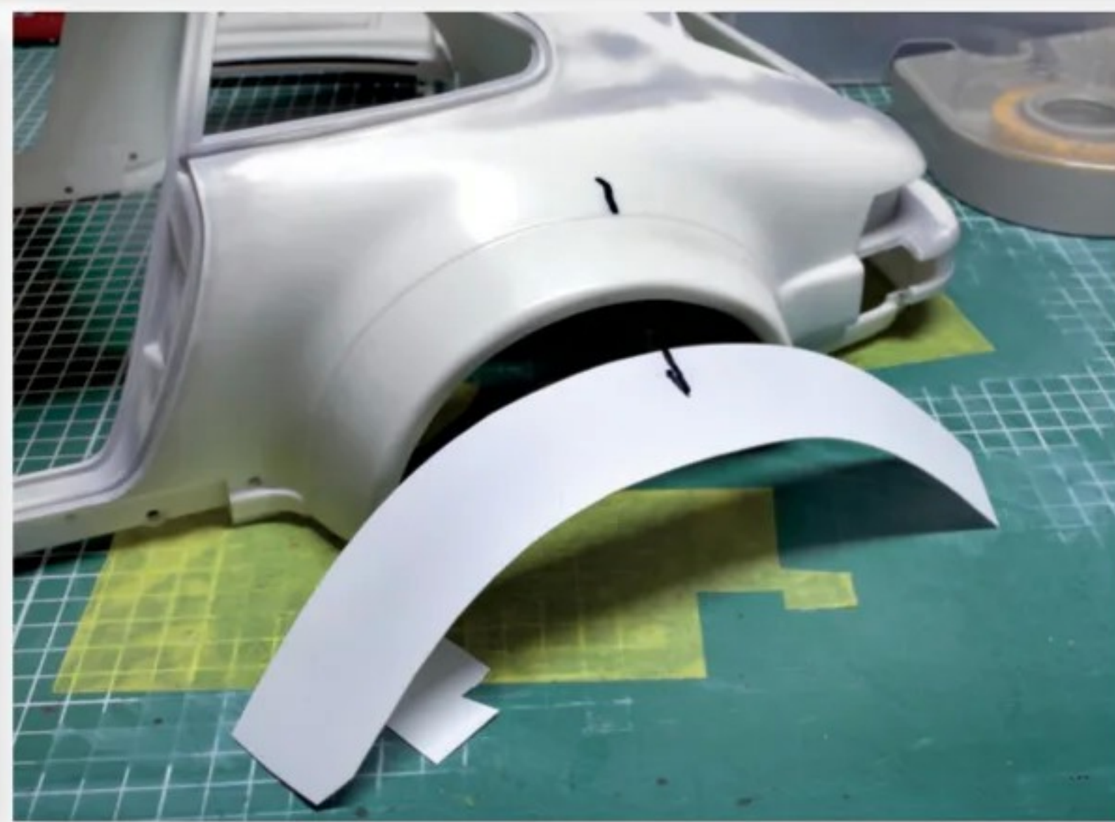
A new arch lift panel is made from thin styrene. Both rear arches are wider than the front. The front wheel arch lifts will take a little more work as they are tighter and thinner
