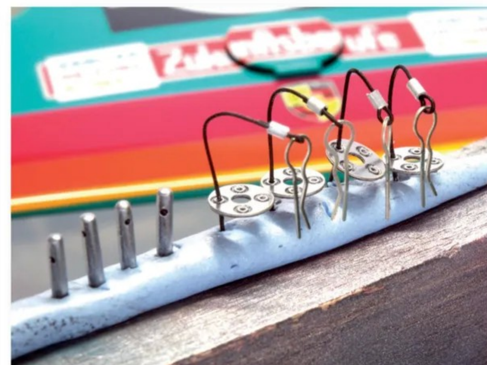
Quick release safety catch items made from different upgrade sets and added wire to simulate pin strap
