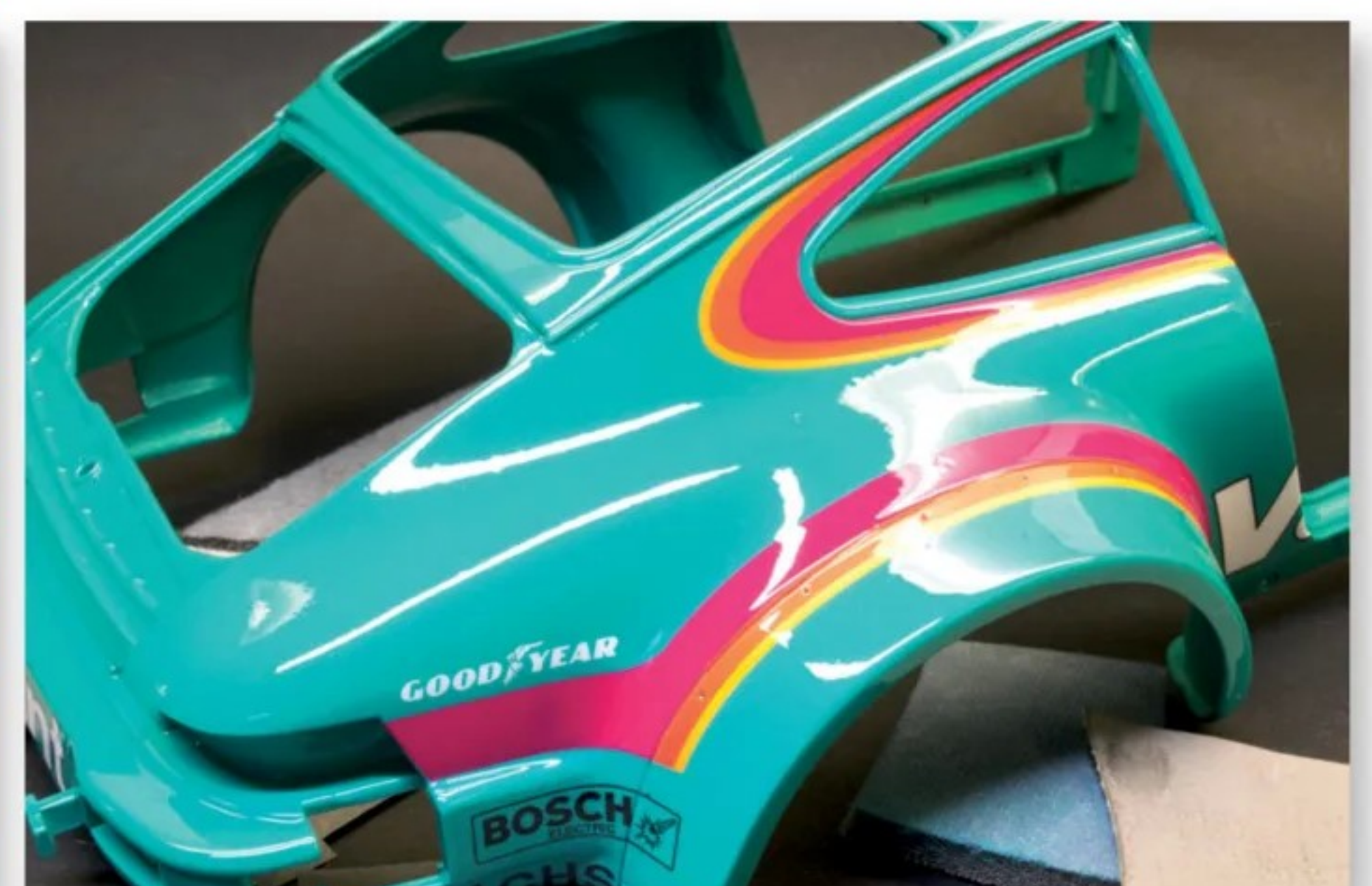
After decal application the main body was 2k gloss lacquered, followed by a full wet sand to smooth the surface prior to the compound work
