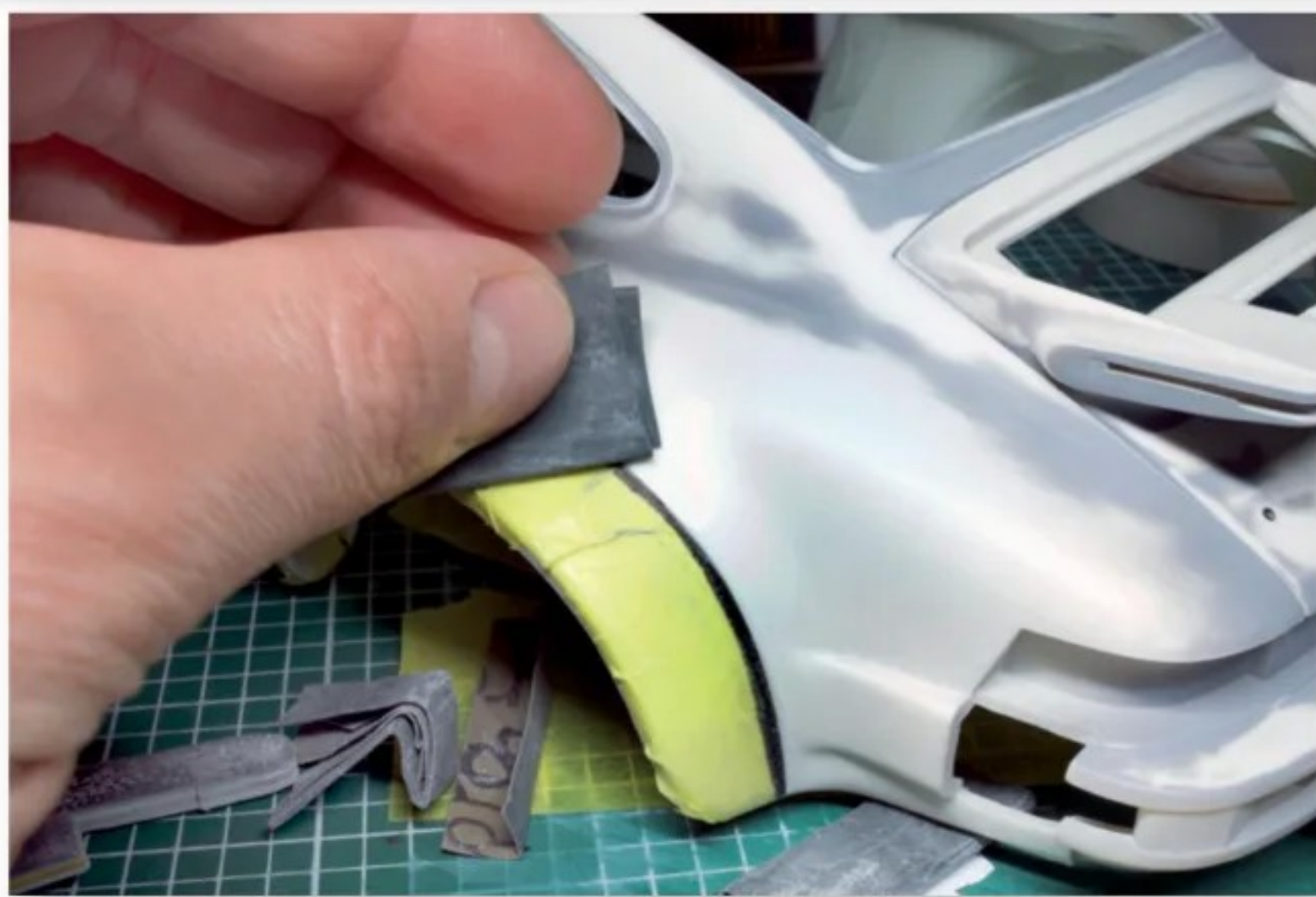
The arch re-work begins with masking stencils being made, then the moulded in wheel arch joining lip is sanded down and smoothed off on all four corners
