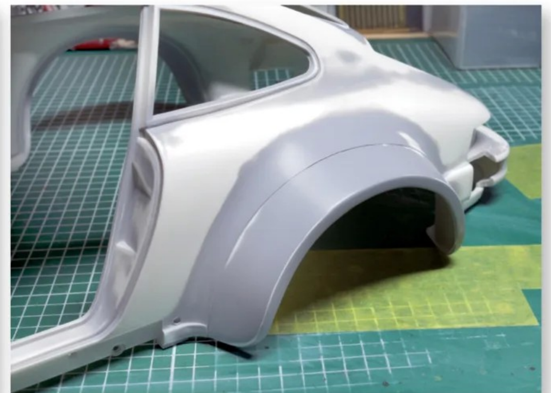
Once the filler was sanded smooth, primer was applied, mainly for a cleaner visual check. The filler/primer steps would be repeated many times until the job was complete
