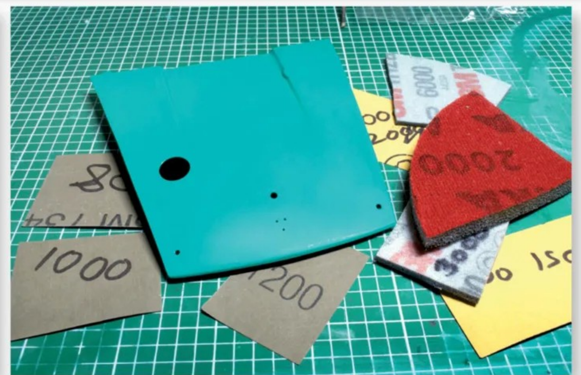
All panels were sanded smooth, to a certain point. Sanding perfection wasn't necessary here, as that's not required at this stage. Perfection can be chased at the end
