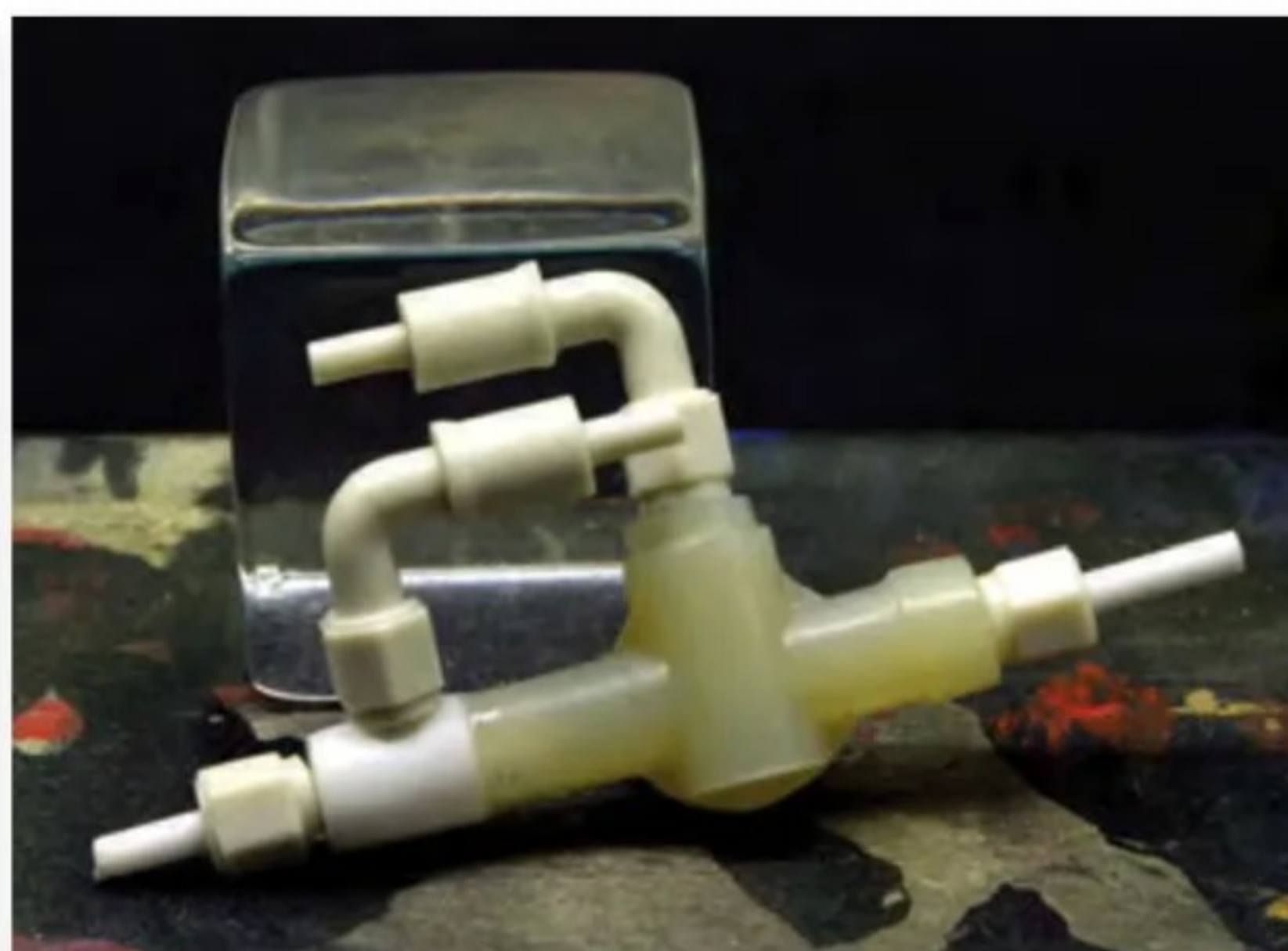
The completed high pressure hose junction. This will be mounted to the side of the tank
