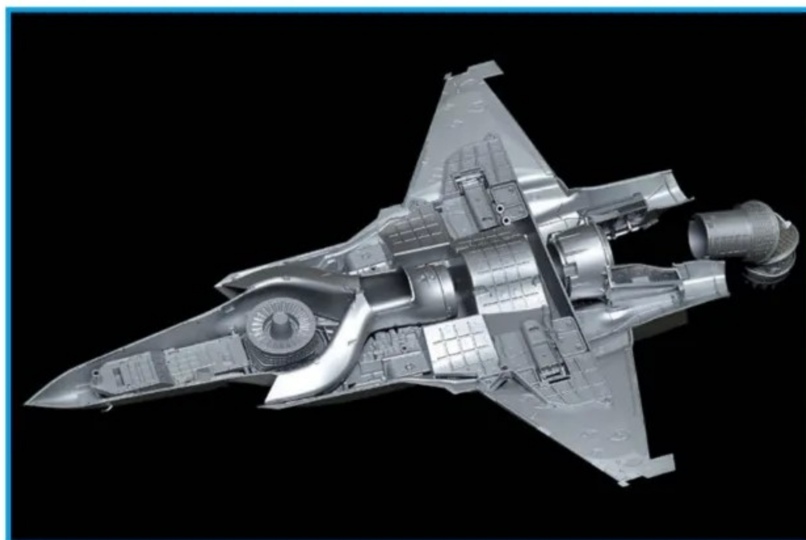
Overview of the fuselage interior showing the huge VSTOL fan behind the cockpit
