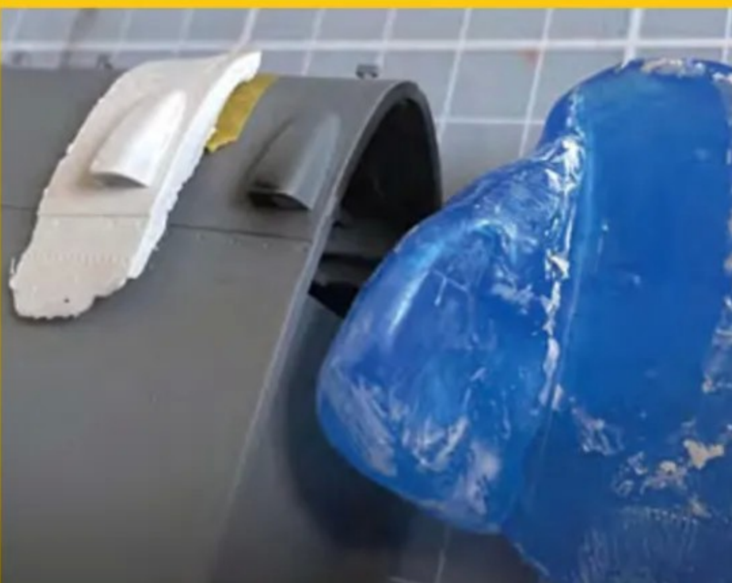
The matching port vent is sadly omitted from the Border Model kit. I moulded Blue Stuff around the starboard vent, then pressed Superfine White Milliput into the mould to make the replica which was trimmed and filed down and fixed in place using Deluxe Rocket Rapid cyanoacrylate adhesive (superglue)
