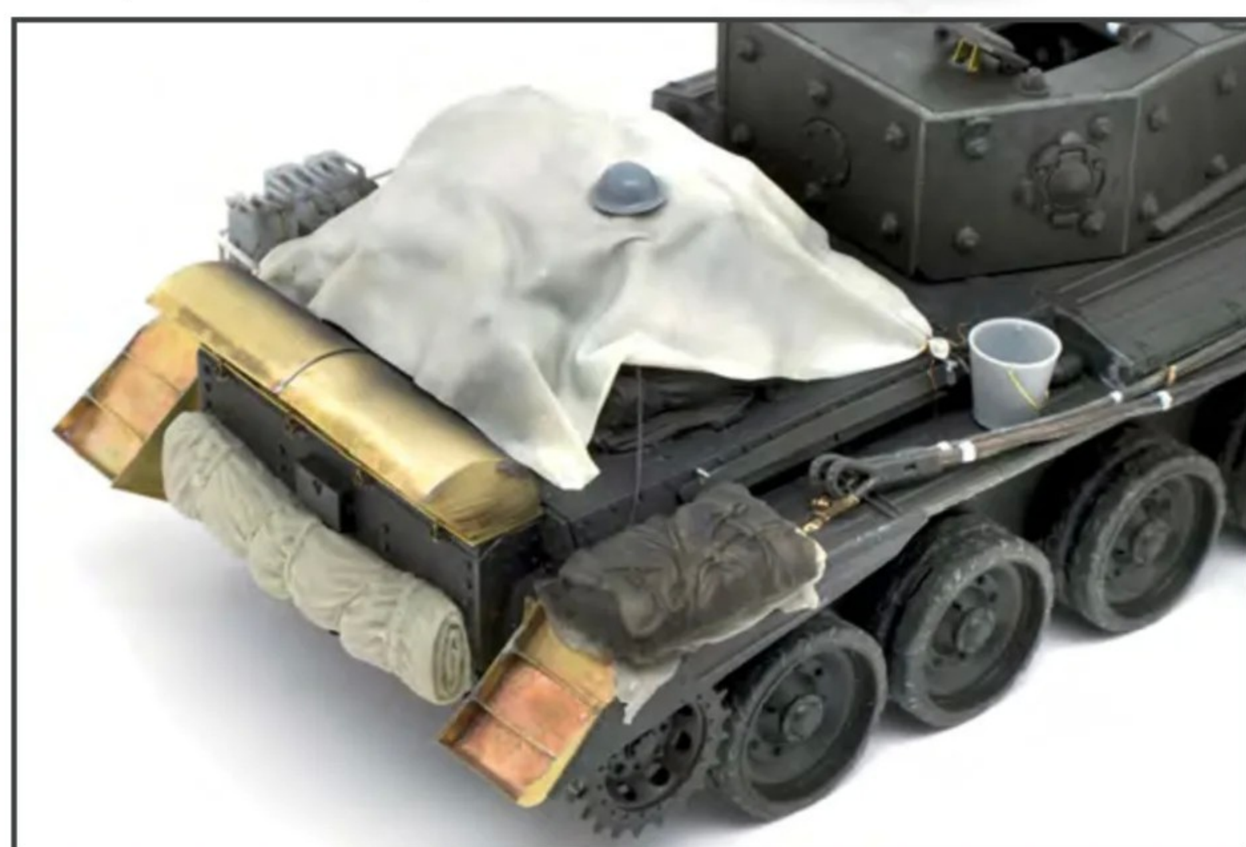
The Normandy Cowling was believed to be made of sheet metal probably cutting from oil barrels. Its purpose was to prevent smoke from being sucked into the crew compartment and making the crew sick. The tarp and worn cloth were made from two-part epoxy putty
