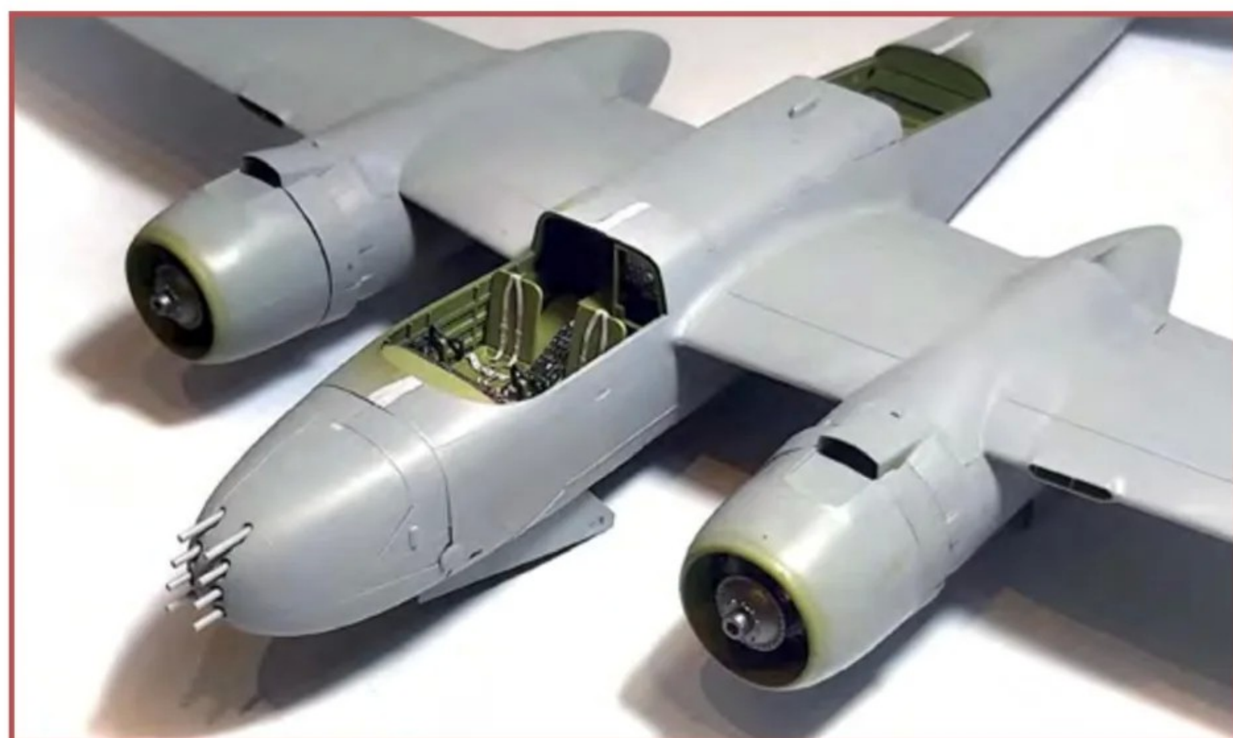
Problems with the fit of the nose; a lot of filling and sanding was needed to make the join flush with the fuselage
