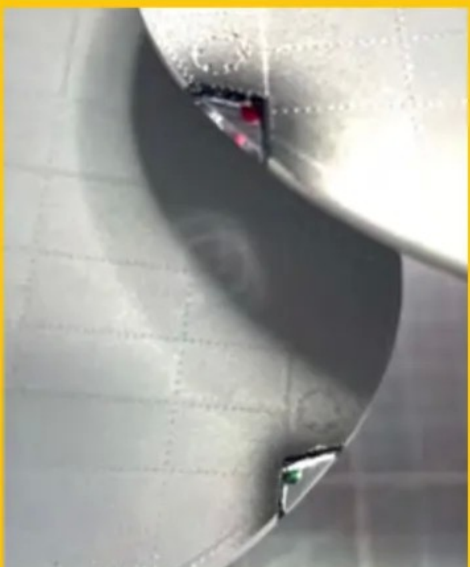
The clear wingtip lights fit poorly but are moulded with divots to paint the bulbs. The surrounds were sprayed black before fixing with CA. Delicate sanding blended them in, retaining the rows of delicately raised rivets
