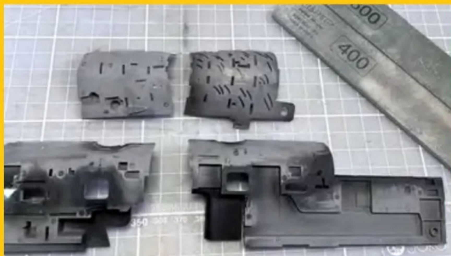
To enable the outer cockpit parts to fit, we need to sand down the raised ejector pin marks and mould seams on the inner nose, indicated by the hatching
