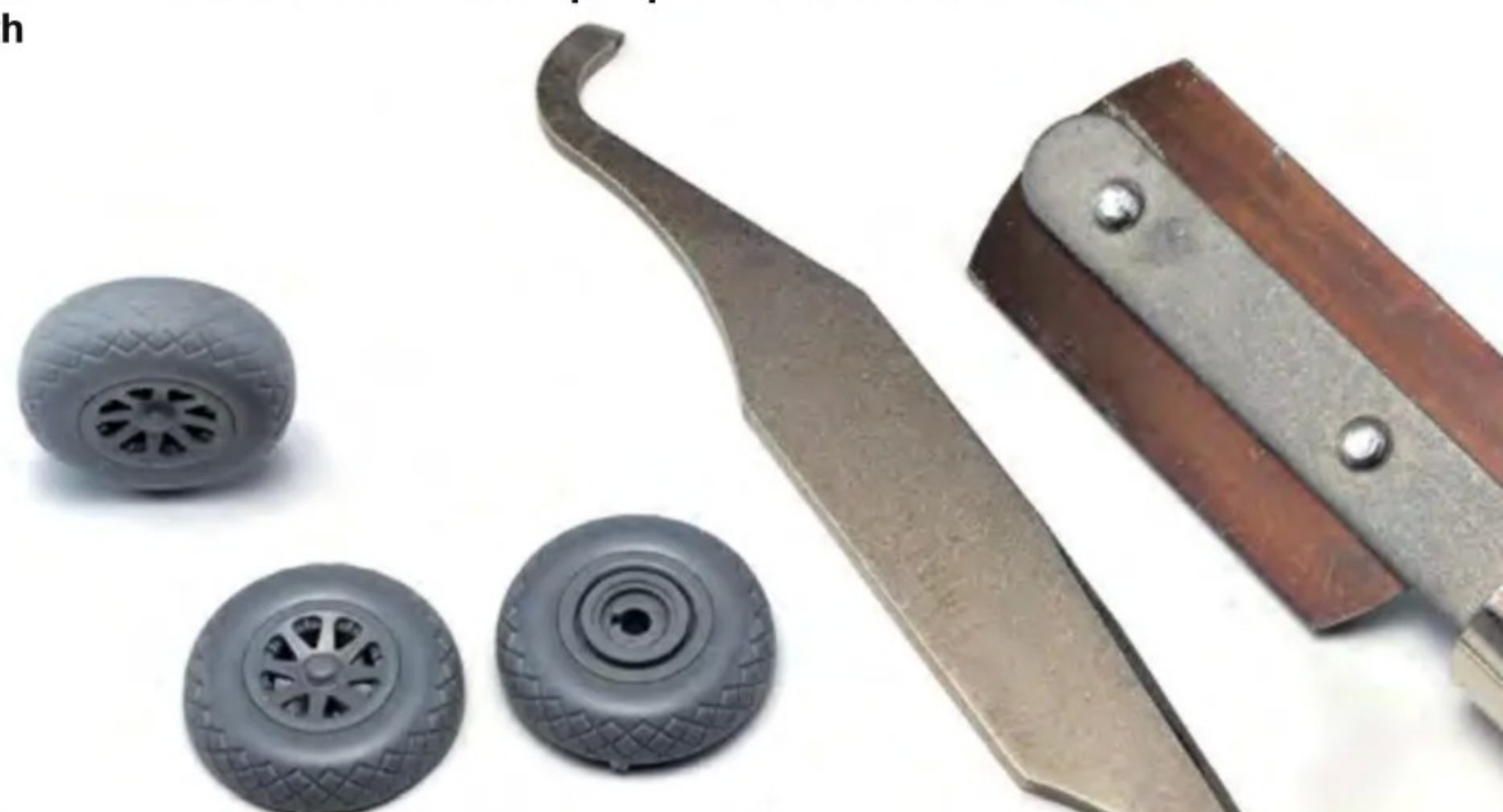
The filled area was spot primed to check for flaws
