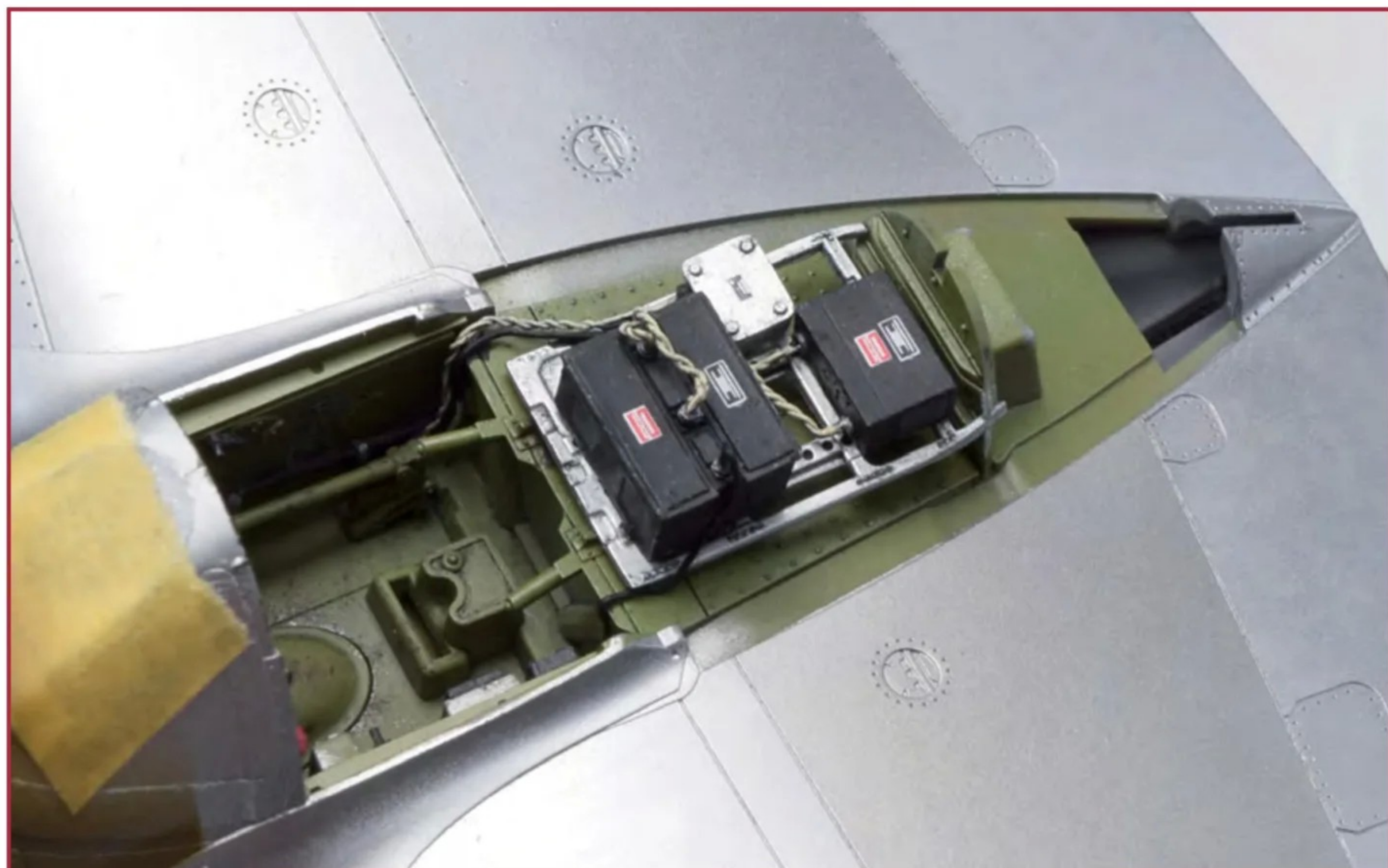
Radio gear painted and detailed with solder wire and placard decals
