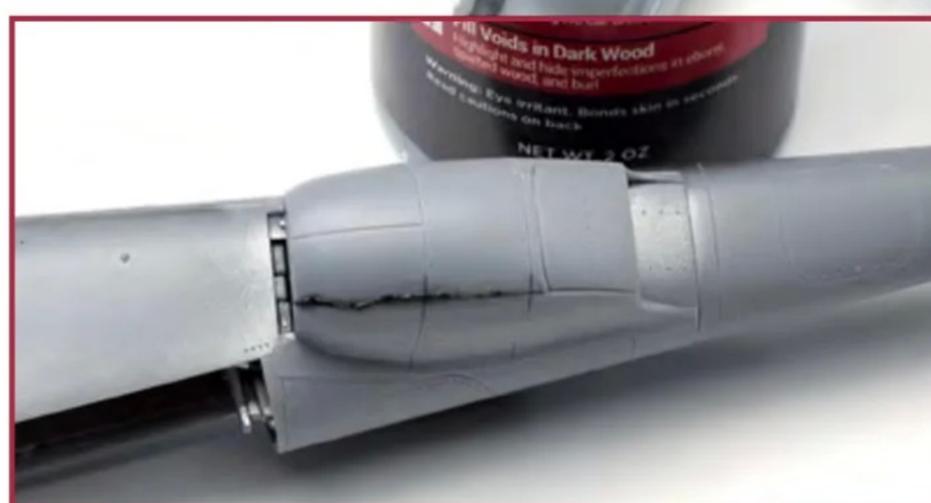
A gap was encountered in the radiator fairings, so it was filled with rubberized black CA, sanded smooth and panel lines restored
