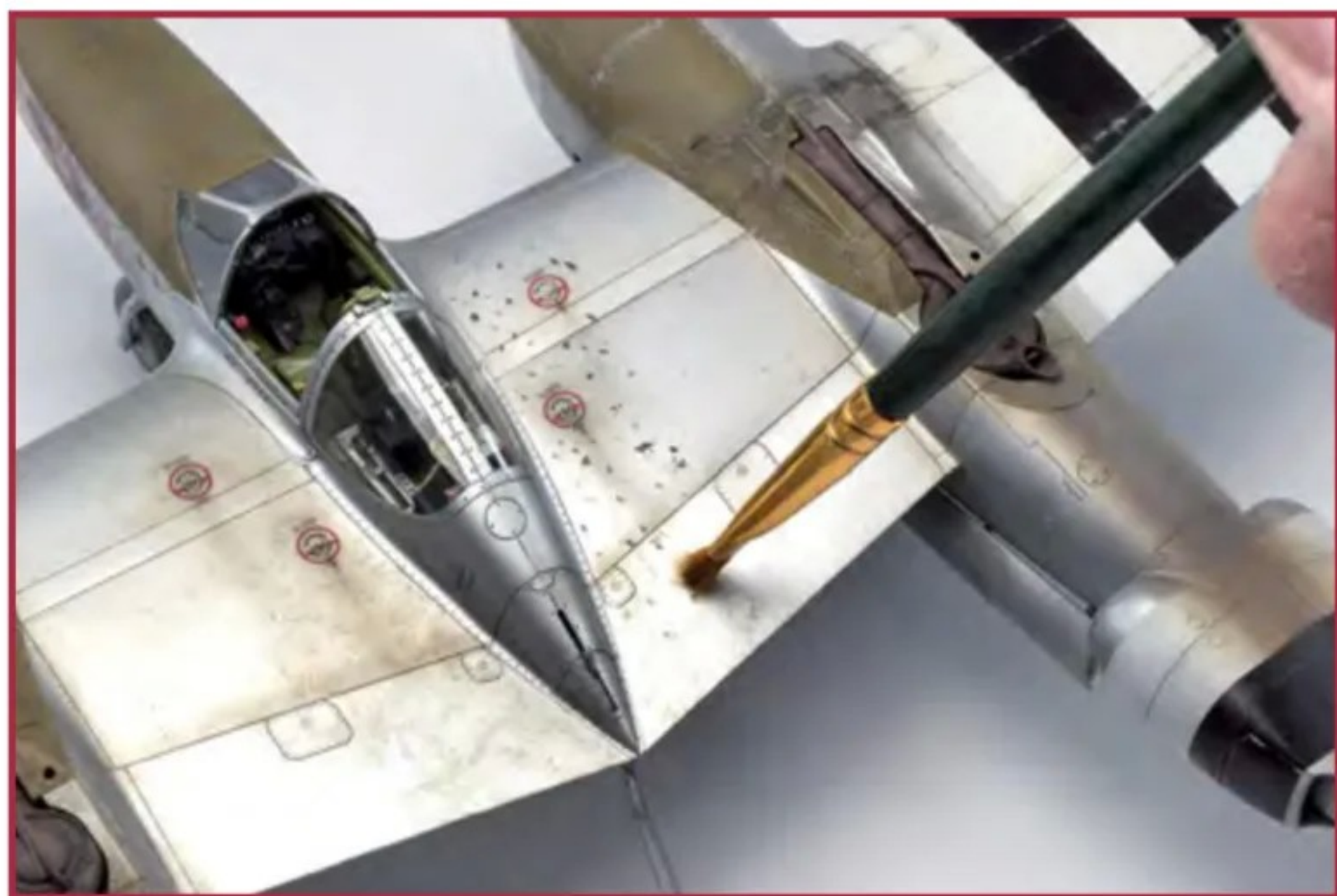
Small dots of oil paints applied to crew access areas and were then stippled with a stiff brush
