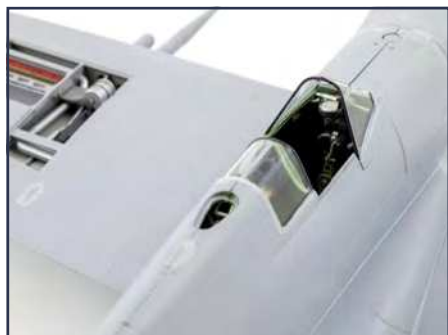
The rear clear canopy part wasn't the best of fits and a little fairing in was needed. In the end this was not noticeable when hidden under the slid back canopy
