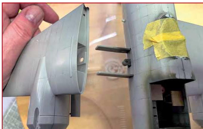
With the fuselage work done, the wings fit onto their spars without issue. Small lugs are designed into the wing root that helps lock the wings in place
