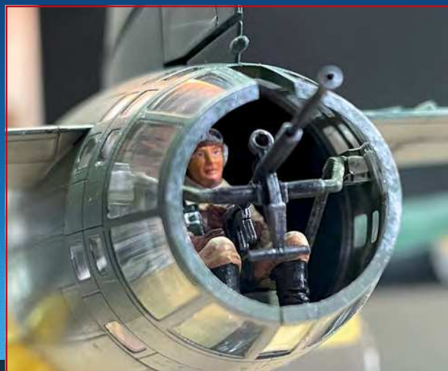
The rear gunner has been shielded by a tube of card stuffed with a piece of sponge throughout the painting process. At the end of the build, he's revealed to become one of the model's main features. The Betty had this intimidating and formidable cannon in the rear. Not formidable enough, though, to defend against the P-38s that shot Yamamoto down
