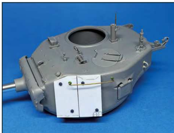
Care was taken to ensure the armour was fixed in precisely the right location in accordance with my reference shots. Some wiggling was needed until that was accomplished, left and right
