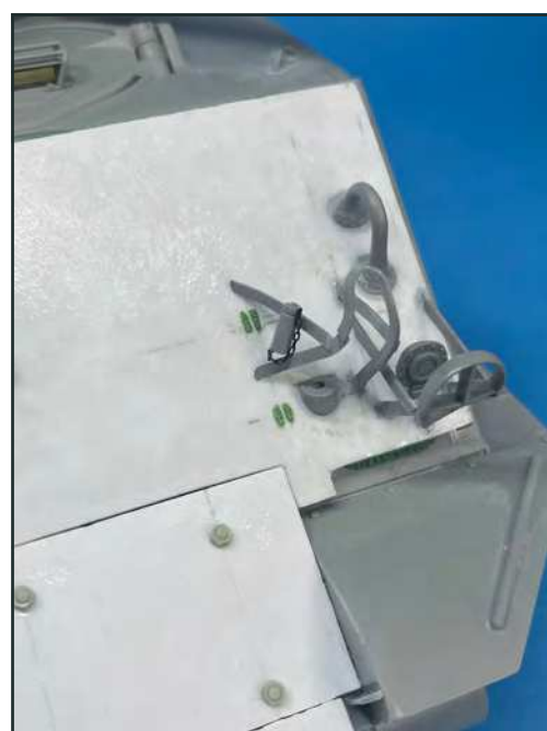
My reference images showed a broken light and deformed guard, so this was replicated on my model. Note how the nose armour is held in place with standard bolts, a detail that contrasts nicely with those locking nuts on the turret
