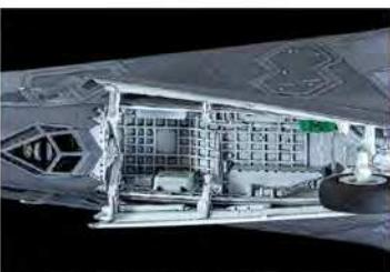
The nose landing gear bay has realistic inside details such as ribs and side boxes.
