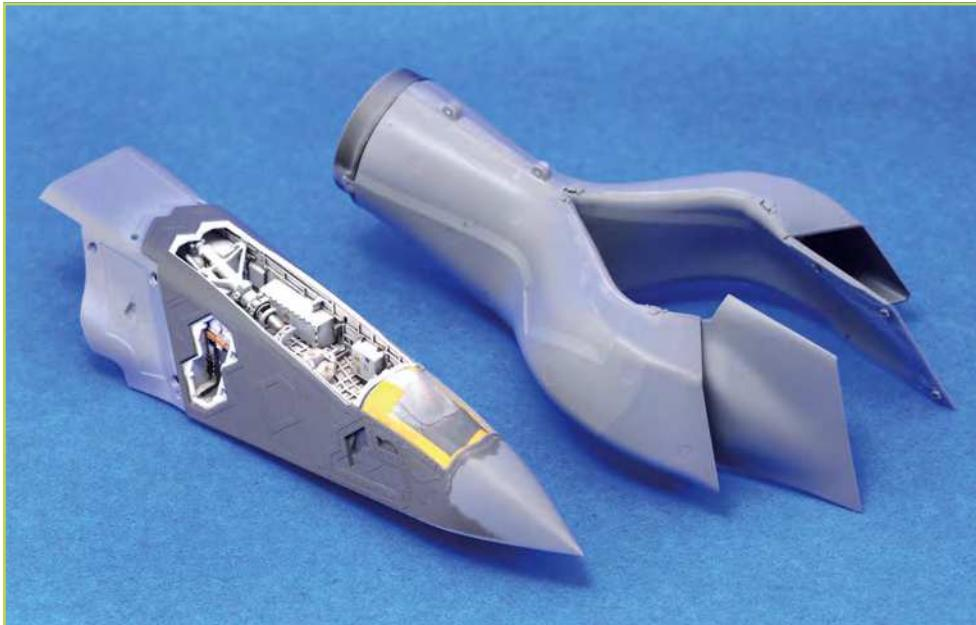
The intake sub-assembly awaits mating to the lower/front fuselage unit in which the front undercarriage bay has already been installed
