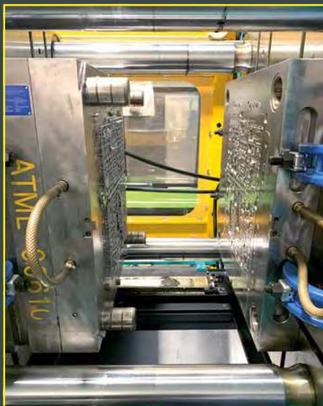
One of Plastech's injection-moulding machines with Spitfire moulds bolted firmly in place. The machine operates at 380-tons of pressure!
