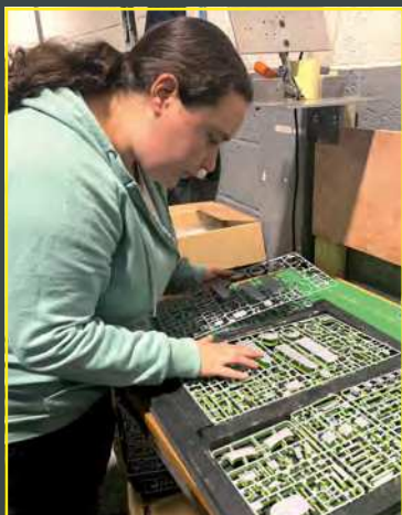
One of Plastech's technicians inspects the new frames for any imperfections, such as short-shots where the plastic didn't fully fill the mould. Airfix's quality control is extremely thorough
