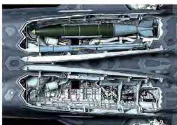
Fuselage weapons bay doors can be assembled open or closed; interior has various cables and lines.
