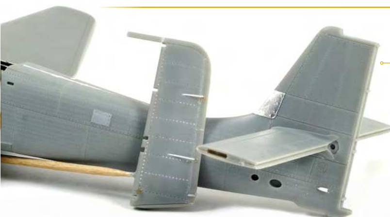
12 After completion of the airframe construction, the entire model was re-engraved. Although very tedious, it is worth taking a closer look at the pictures of the finished model
