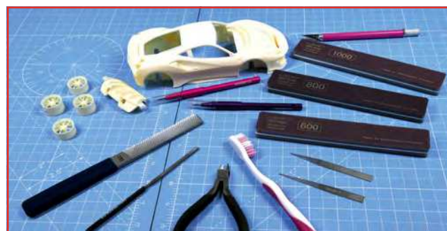
Some of the many modelling tools used to prepare the resin parts prior to paint. Not shown here, is however possibly the most important item is a good quality face mask as the particles flying about in the air when you are sanding, filing or scribing resin can be dangerous to your health
