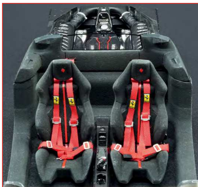
Carbon fibre Ferrari racing seats installed in the cabin, complete with full four point racing harnesses
