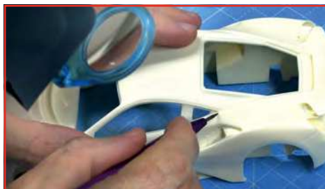
Scribing work around the windows was dual purpose. One scribe line was required to deepen the panel lines and door openings; another line was required to provide a neat masking tape cut guide line when painting the black 'rubber' areas before adding the windows. All this work needs to be done at prep stage
