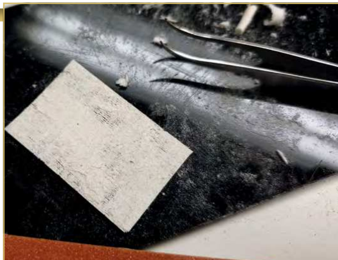
The scary and probably unnecessary part; thinning the back of the paper with a sharp knife, a sanding stick, and tweezers
