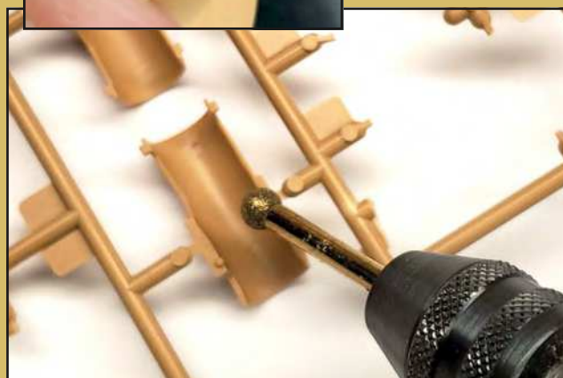
I used a Proxxon rotary tool to thin out the inside of the exhaust shields and the back side of the side skirts
