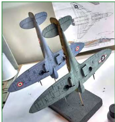
A block of Styrofoam and a couple of cocktail sticks makes a decent DIY drying stand
