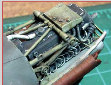
The gear in place. The upper diagonals are styrene stock and the light-coloured reinforcements are merely painted on. It's worthy to note that the gear was electrically driven via a long jack-screw and not hydraulics
