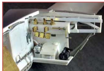
The rear panel was evidently open to the bomb bay; draughty! Empty cartridge case box and central rear panel, replete with doppletrommel holders, battery boxes, emergency landing gear manual crank and the auto pilot motor (an ancient model railroad brake part). Never throw anything away and use the best you've saved!
