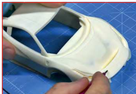
Preparation work on the resin included sanding out some slight imperfections on the body shell and using scribes to open out the panel lines (make them a bit deeper)
