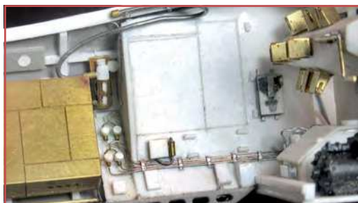
The port radioman's station was also largely rebuilt. The cockpit was incredibly cramped and crowded. I built up the contents in layers; new fuse panel, document pouch and such. Brass was soldered when possible for strength
