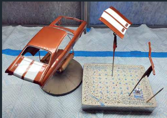
With the decals all done and the Bare Metal Foil complete the panel lines received a wash with some dark grey Tamiya Panel Line Accent colour. It was then time for the clear coat to seal everything in and give the body that lovely gloss shine. I used my now go to 2k clear from Gravity Colors. This is after the third and final wet coat, where we are left with a lovely smooth glass like finish
