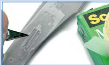
The panels of the outputs of the four machine guns and the two barrels of the fuselage are excessively staggered so I set out to correct them. I masked with 3M Magic Tape and cut along the line of the panels, exposing them
