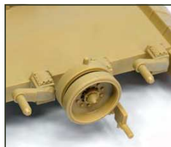
In order to perfectly align the tracks, one of the roadwheels, right and left, feature a different locating mount and then this pin that slots through the lower run of track
