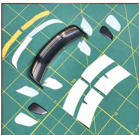
Here we can see the rear wing and its mounts being templated up, before 2k clear coat (above) and after (right)
