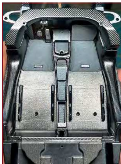
The tub was considered done after applying carbon-fibre decals and painting the carpets with grey texture-paint
