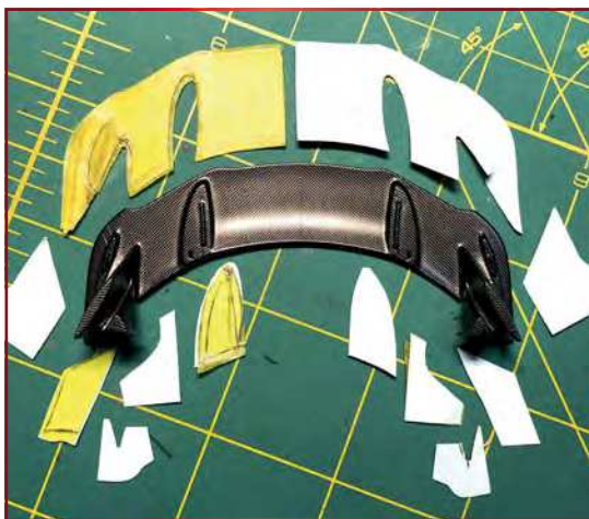
Applying 1:12 scale carbon-fibre decals to the front splitter except the lip, where 1:20 was used
