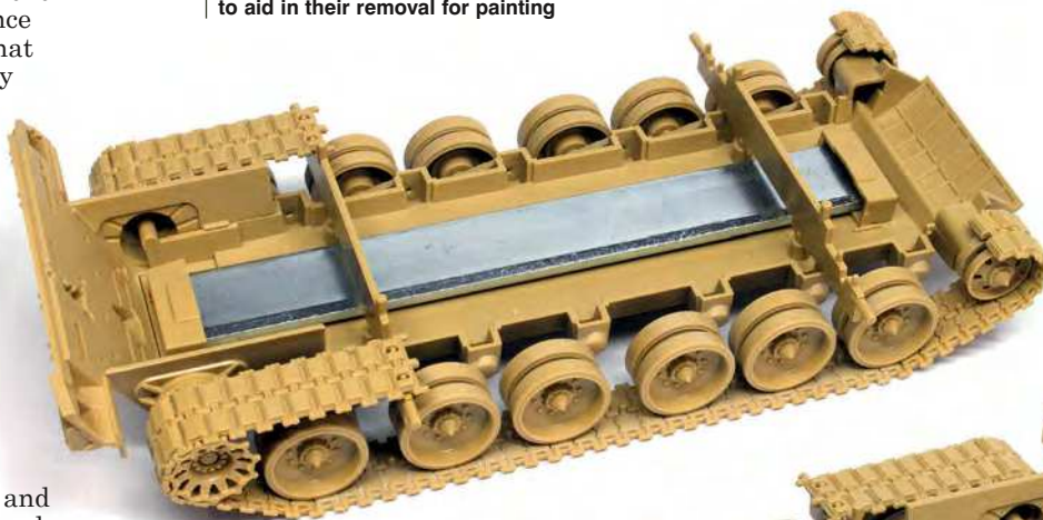
In order to perfectly align the tracks, one of the roadwheels, right and left, feature a different locating mount and then this pin that slots through the lower run of track
