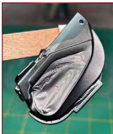
Applying carbon-fibre decal to the door panel was very complicated. It had to be cut with a knife where the central aperture is, but the results looked amazing
