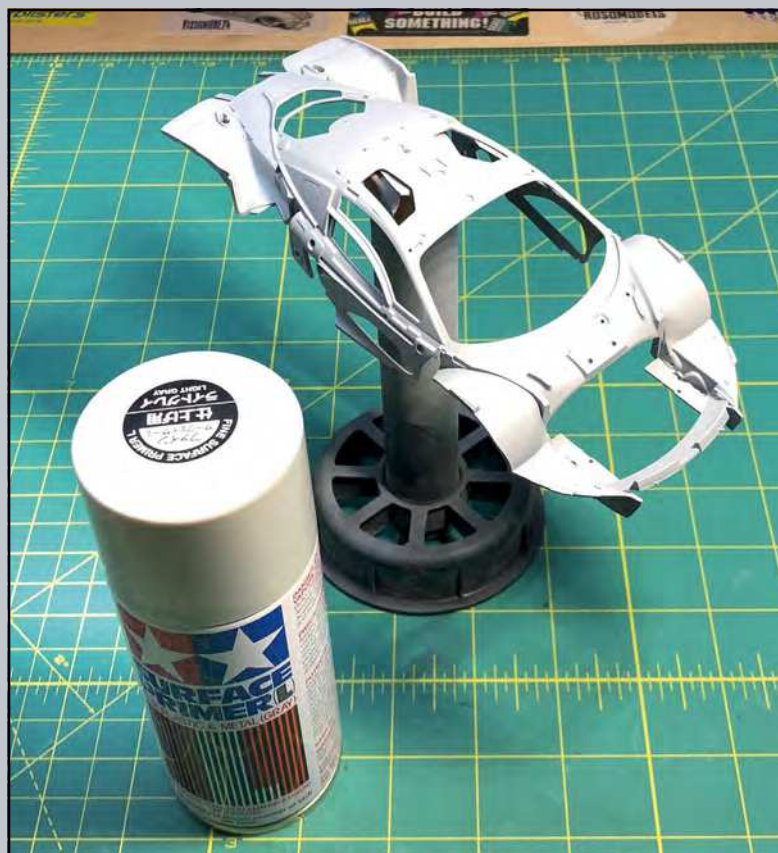
After cleaning the under-panels the author used Tamiya Grey Primer as an undercoat
