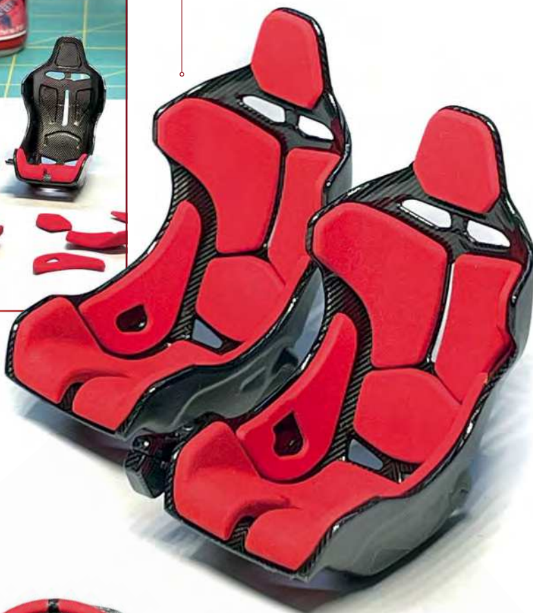
After using automotive 2k clear coat on the seat shells, the pads were then glued to the seats. The pads being separate made things much easier
