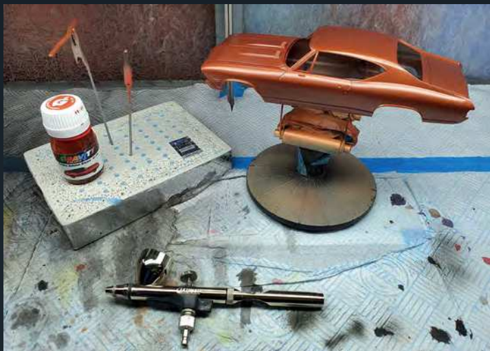
After eight coats of the Pontiac Autumn Bronze I was happy with the depth and coverage of the colour. The paint being a metallic was sprayed with a UMP Apex using the 0.2mm needle conversion. Now that the base-coat was complete the body was left for 24 hours before moving on with the decals and Bare Metal Foil on the various trim pieces
