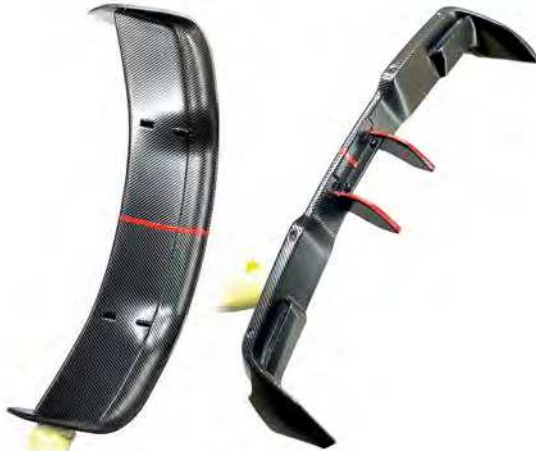
Here we can see the rear wing and its mounts being templated up, before 2k clear coat (above) and after (right)
