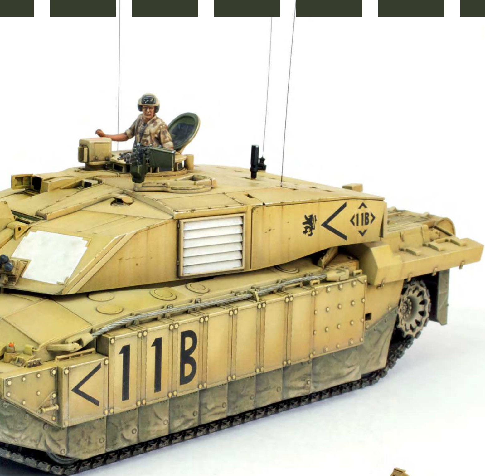
Here's the completed lower hull. The bulkheads that you see are a clever way to hold the side-skirts and upper run of tracks in place
