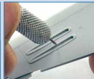
Finally, I deepened the rivets with an awl
