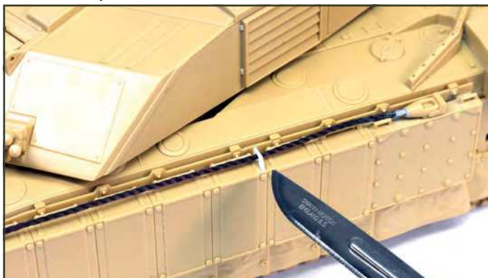
And finally! I added a small bracket for the tow cable, a simple chip of plastic card replicating this feature in 1:48
