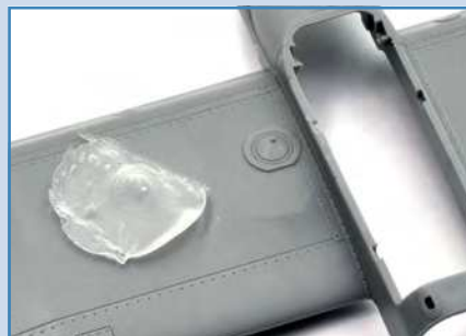
With a little silicone, the existing panel mould was made
