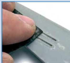
With a fine-grit sandpaper, I roughened the plastic until it was levelled with the 3M tape
