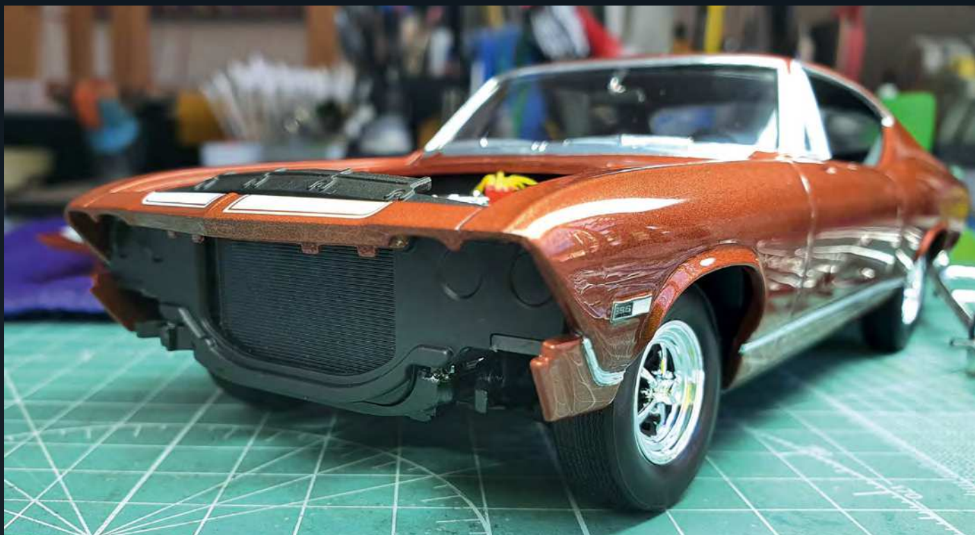
Body on and wheels fitted. The body and chassis fit on this model is tight, very tight. It does take some persuasion (and a strong will to flex the body far enough to let it slide over the interior) but once in place it sits nicely and there are no interference issues
