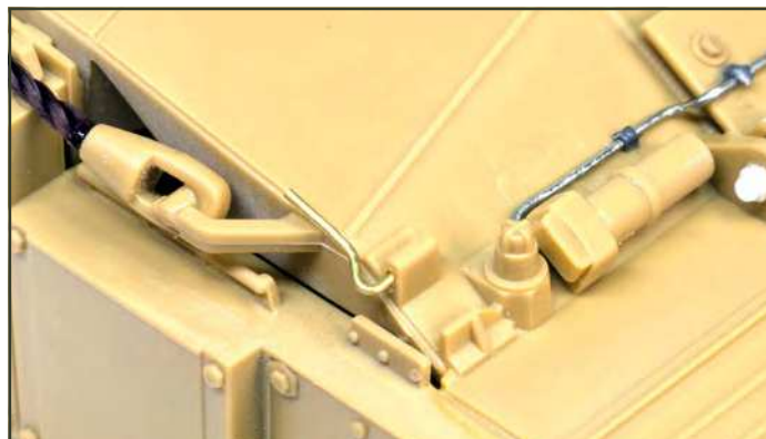
Another small addition was this mirror bracket, made here from copper wire, bent to shape
