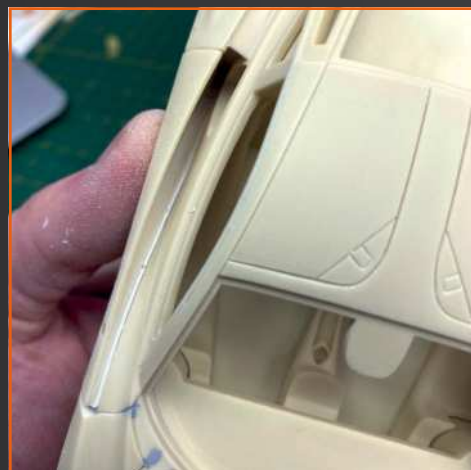
Checking the gaps between the door and fender
