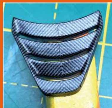
Carbon-fibre decals applied and ready for 2K clear from Streetblisters
