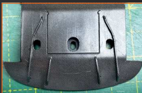
Rear diffuser in carbon-fibre, ready for coat of Semi-Gloss Clear from Zero Paints
