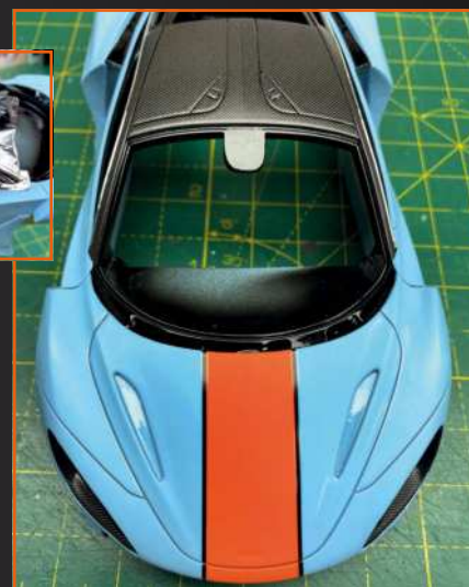
Applying 1mm black stripes decals from Microscale
