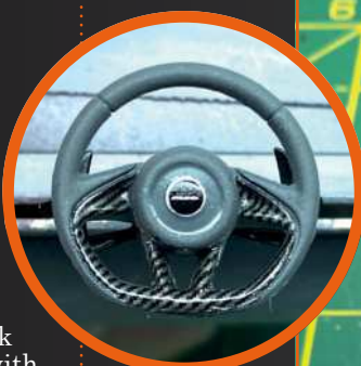
Finished steering wheel with carbon-fibre decal
