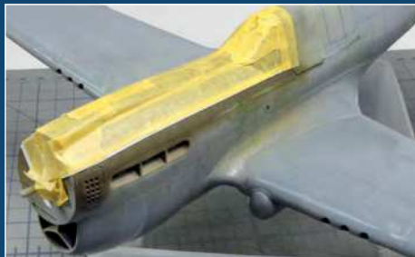
After a primer coat of Mr. Surfacer 1500, the aircraft was painted using Testors Model Master Buffable Aluminum Plate. After a 24 hour "setting" period, the paint was thoroughly buffed using a Dremel polishing disc
