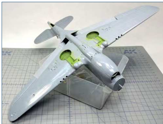
Attaching the wing to the fuselage leaves behind many seams the require filling, particularly around the forward wing root section
