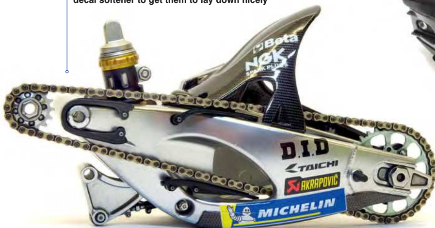
The completed swing arm. Be careful applying those large 'Michelin' decals as they seem very thick. Use gentle heat along with a decent strength decal softener to get them to lay down nicely
