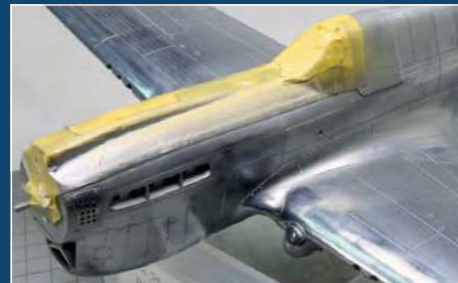
After a primer coat of Mr. Surfacer 1500, the aircraft was painted using Testors Model Master Buffable Aluminum Plate. After a 24 hour "setting" period, the paint was thoroughly buffed using a Dremel polishing disc
