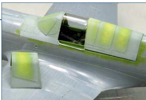
Pros and cons. The forward windscreen design is brilliant and trouble free. The rear canopy is problematic, as blending the hard clear plastic and the soft grey plastic requires some extra attention
