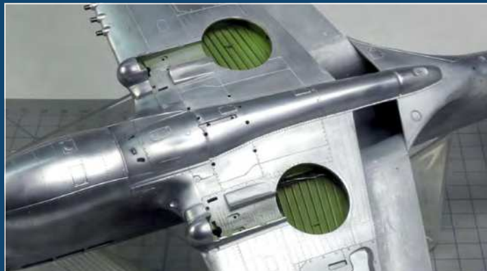
Decals were applied using MicroSet and MicroSol. If there is a clear protective coat, the Metallizer is not damaged by this process
