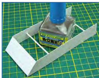
The rooftop frame was assembled from sheets of plastic card
