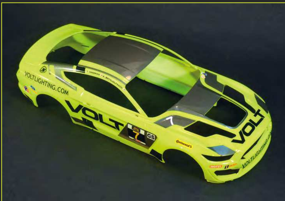
The bodywork finished after application of Zero Paints two-component polyurethane varnish
