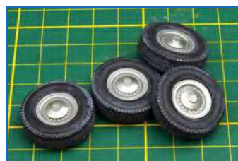
The wheels were painted with black primer and then with Mr Hobby silver for the hubs, weathered with a grey oil paint colour-wash
