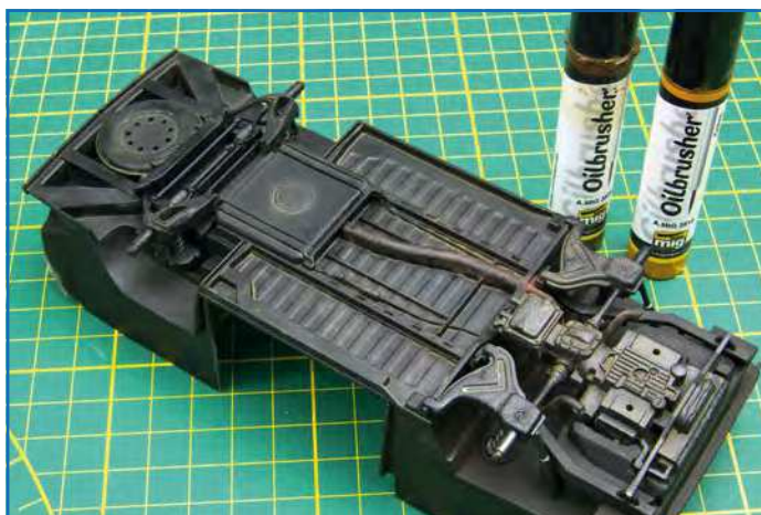
After assembling all the elements of the undercarriage, I applied black primer from Mr Hobby with an airbrush and at the same time I gave it a little weathering.
