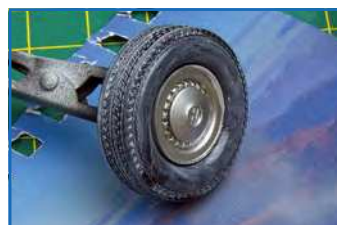
The small parts needed a solid clean-up of flash and other imperfections before being glued together
