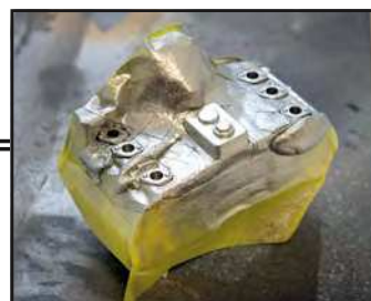
Further paint masking to finish up the final detail. Once all masking is taken away the colour shading and tidy up can be begin
