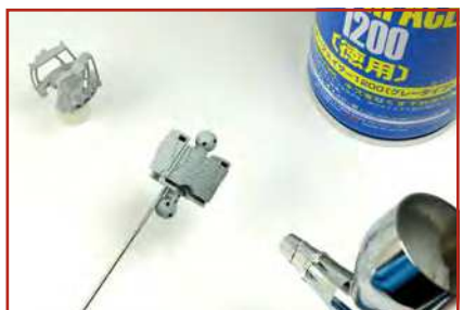
The lower torso was primed with Mr. Surfacer 1200
