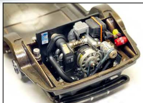
Once fitted there are other smaller items to add to finish up the engine bay. Thankfully this will all be visible due to the ability to open the rear bonnet
