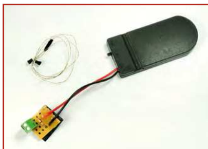
A LED circuit by Tiryidium Models will need to be installed inside the C-3PO's body
