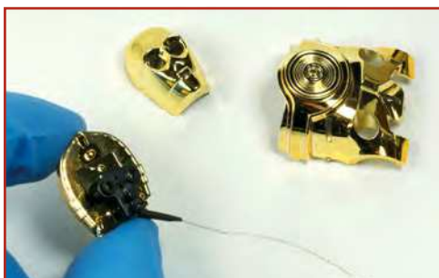
The first step is to place the diodes inside the eye sockets. Then you have to start threading the wires through different parts of the droid's body
