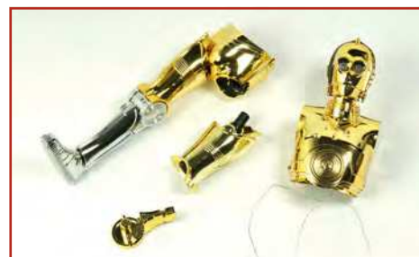
I put together the next parts of droid's body leaving them movable whenever possible. I had to plan ahead how the wire would go through and on some occasions I drilled a wider passage
