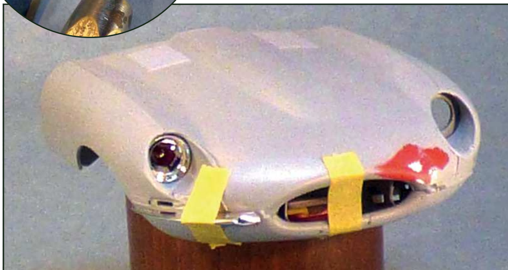
An assembly test of the chrome parts shows that the paint layer must be thin, otherwise it will no longer be possible to fix these parts correctly
