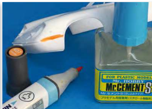
There is a joint around the lower nose, here being highlighted ready for filling and sanding
