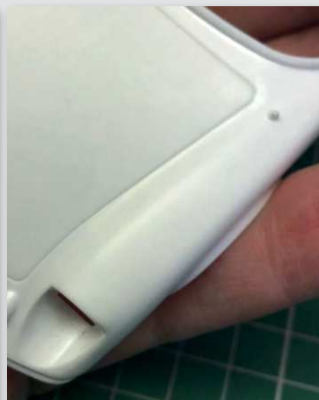
Care is needed to ensure that the surface of the body shell is as smooth as possible, wet 'n' dry paper, followed by a polish with Scotchbrite, being needed to remove the mould lines that flow over the wings and edges of the roof and rear quarter panels
