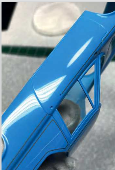
This is the result of several dust coats, overlaid with one heavy 'wet' coat, the latter thinned with around 70% Mr. Color Leveling Thinner
