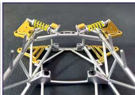
The upper part of the rear chassis attached to the lower. You are instructed to fit the engine and gearbox to the lower chassis before doing this, but I decided that I would add the engine and gearbox later
