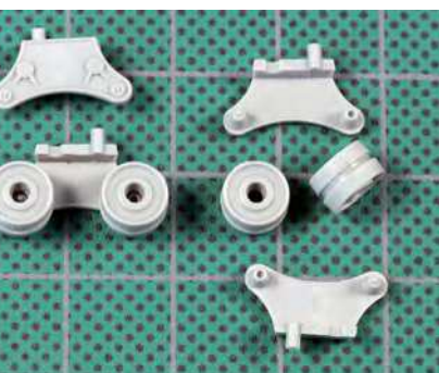
The road wheels are grouped in pairs on the bogies. If only the upper part of the supports is glued, their mobility is preserved, which is always helps at the painting stage. The bolts securing the axles have not been changed at this stage
