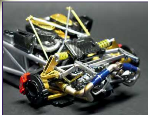
The finished rear chassis and engine area, a big milestone as it was the first completed area
