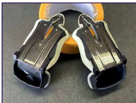
The seat backs were again clear coated using 2K from Firescale Modeler, I also added some Top Studio rivet heads
