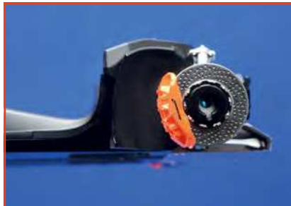
Here we see the very compact front suspension, with brakes and shock absorbers in place. The front wheels are steerable but only to a limited degree on the finished model
