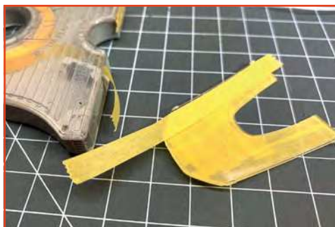
The front and rear windcreens, plus upper side windows must have their edges painted gloss black, which calls for some extensive masking. One side was covered with tape, allowing for a margin, which was then trimmed off, using the edge of the moulding as a guide
