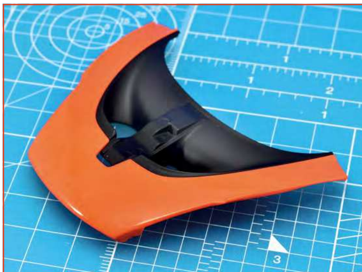
The upper part of the radiator duct (in black) fits to the painted bonnet/nose panel via four tabs that locate very positively to the underside of the orange-painted panel
