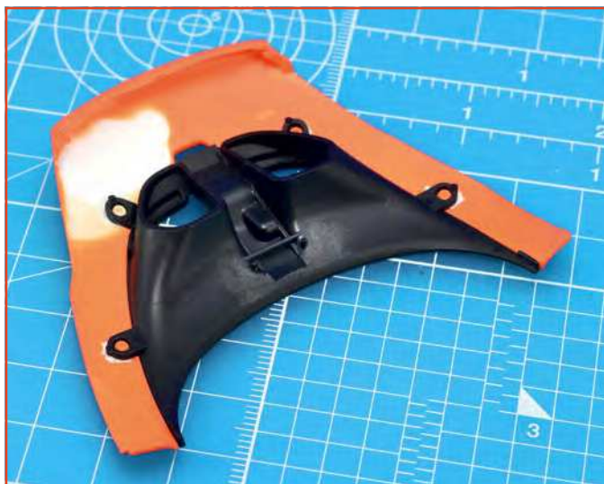
The four tabs can be seen here. The orange paint's over-spray (as well as the black paint on the tabs) has been scraped off to create a plastic-to-plastic contact so the liquid cement can bond properly
