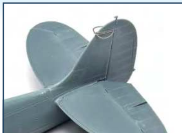
Tail components including the parachute guard designed to prevent the lines from becoming entangled in the fin/rudder
