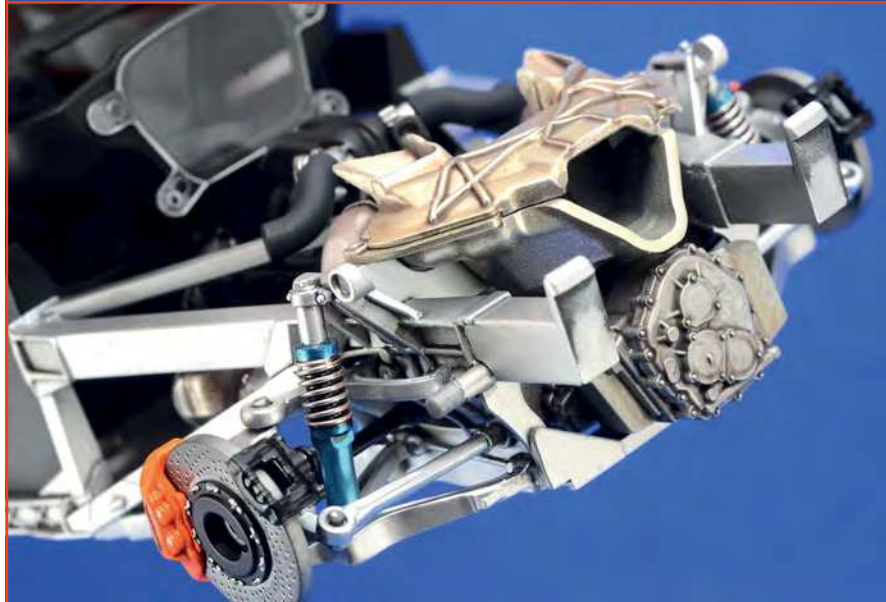
Jumping through quite a few stages here, we see the rear chassis elements in place, with the engine, exhaust, suspension and brakes installed. Almost all of this will be nearly totally hidden on the finished model!
