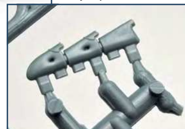
Some unfortunate sink marks in the exhausts
