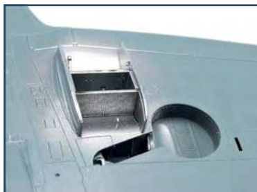
Lower wing radiator with a detail wash prior to closing up
