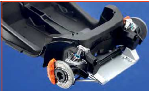
Here we see the very compact front suspension, with brakes and shock absorbers in place. The front wheels are steerable but only to a limited degree on the finished model
