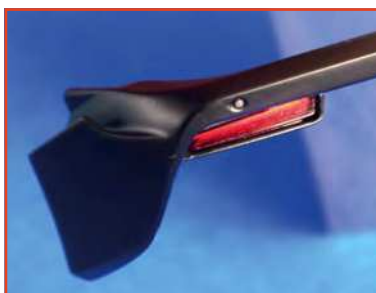
The rear lights are far simpler; just one clear part each. While still on the sprue, each lens was airbrushed with Tamiya LP-52 Clear Red and allowed to cure for a few days. The rear face was then airbrushed with Alclad 2 Chrome and the part then trimmed from the sprue and fixed into place with 'Future' floor polish
