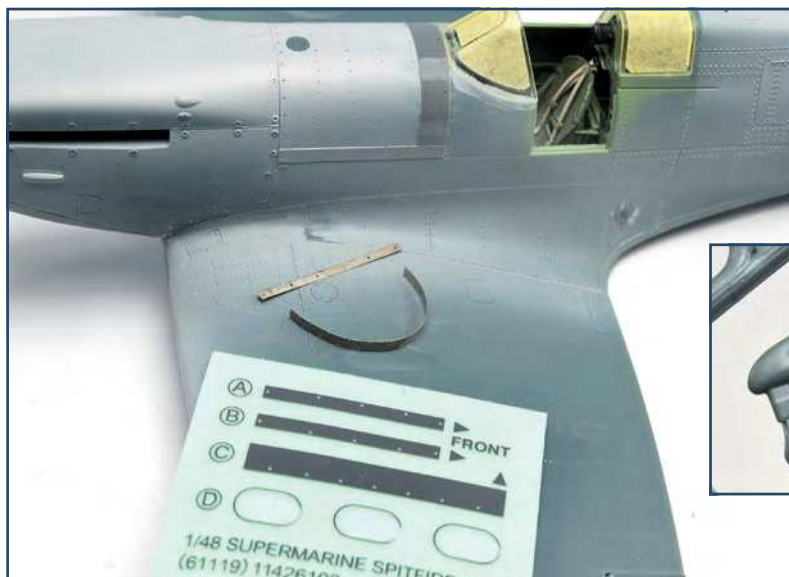
Kit supplied PE parts for the unarmoured fuel tank cover and the author's alternative parts sourced from a Tamiya Spitfire
