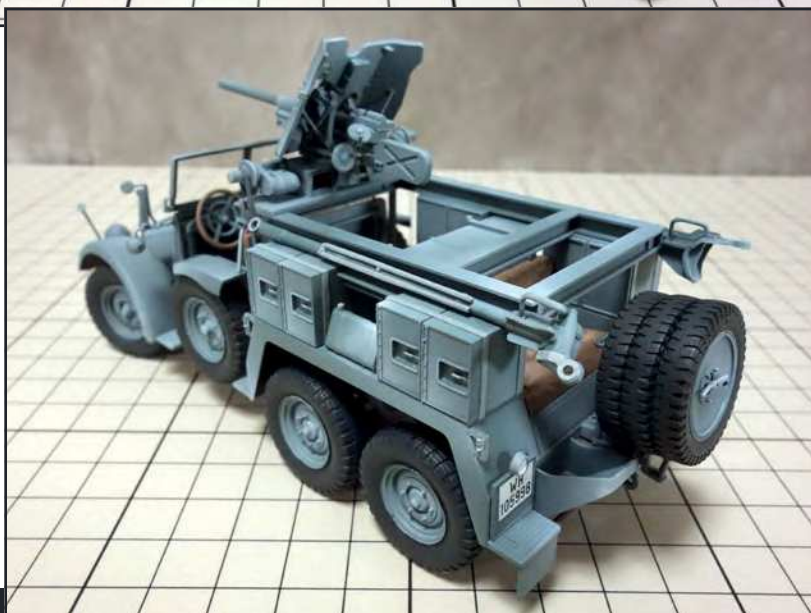
The completed vehicle was airbrushed with Tamiya XF-22 RLM Grey and highlights sprayed from above, with some white added, well thinned. For shading, more RLM Grey plus a little black was airbrushed from below
