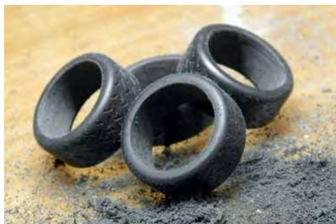
Adaptation of the internal diameter of the tyres in order to insert the rim correctly
