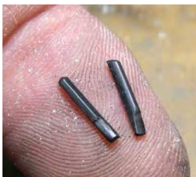
The door handles were remade from two pieces of sprue, cut, filed and sanded to shape
