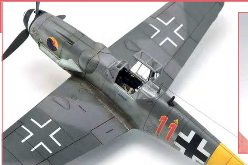
Some chipping was sparingly applied using a sharpened Prismacolor silver pencil
