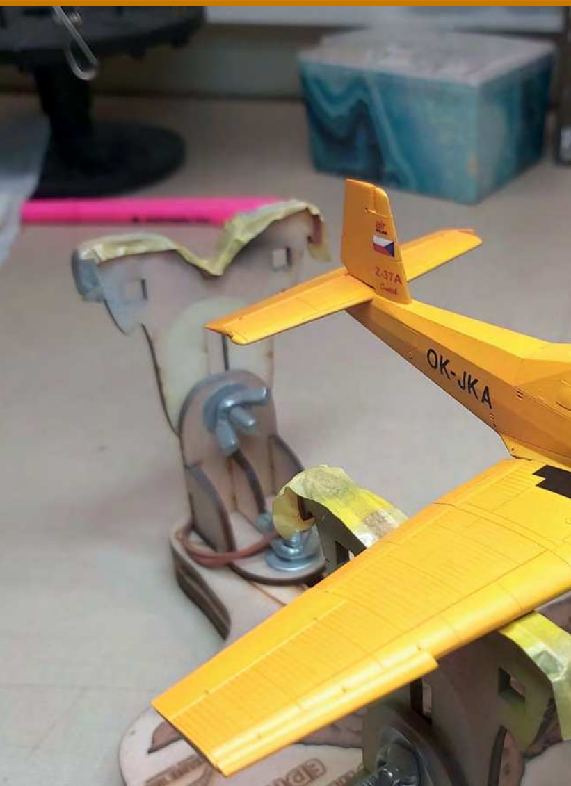
Three coats of Mr Color C113 RLM04 Yellow, diluted with Mr Color lacquer thinner, were then sprayed. Once this was done, the individual panels were lightly shaded
