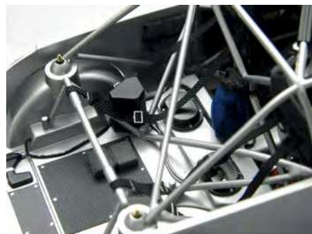
Completed rear area of the passenger compartment showing carbon-fiber structures and seat harnesses
