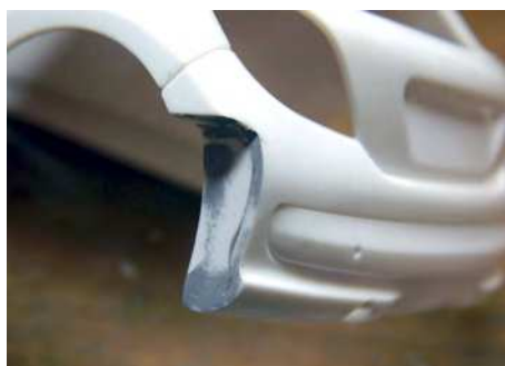
The 'EVO' rear bumper redone, filled and ready for painting
