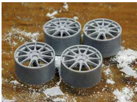
The 'Reji' wheels during the cleaning and filling work. Many defects were found
