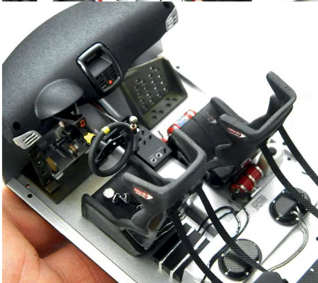
Images of the complete passenger compartment before the fitting of the roll-cage
