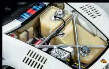
Front hood is removable, allowing inspection of fuel tank, oil tank, battery and washer tank.
