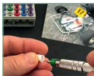
Micro drills were used to open up the wheels for new bolts
