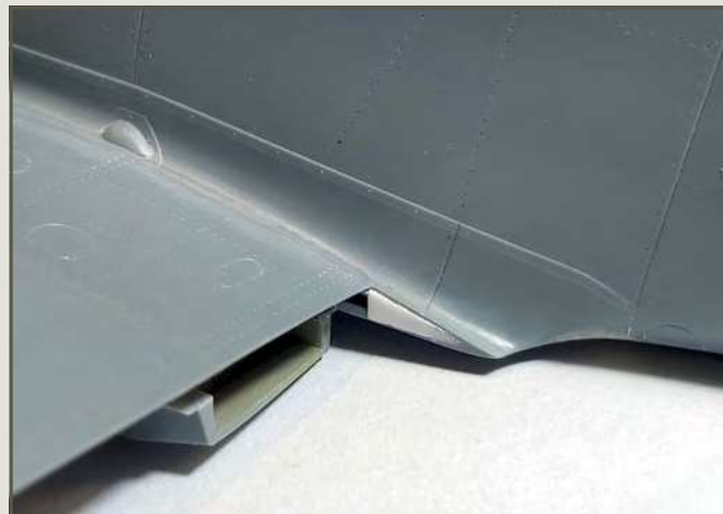
Plastic card fillets were used to fill the apertures formed when the flaps are 'dropped'
