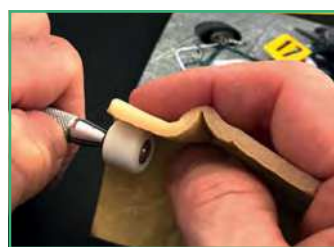
A tyre is being spun on a minidrill to create a smooth tread
