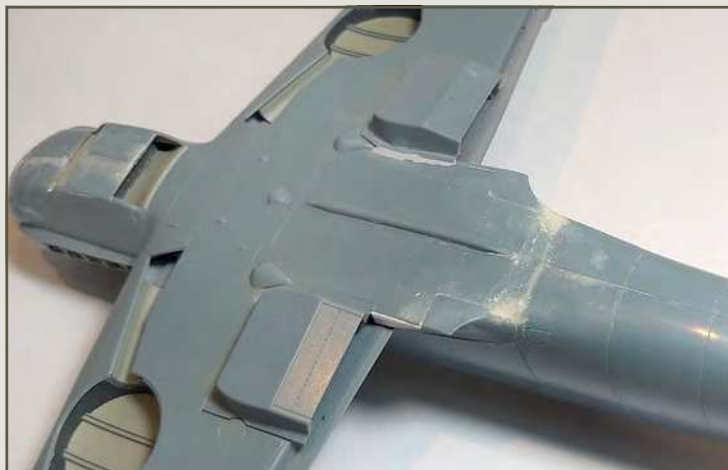
Some filling/sanding was needed where the rear wing root meets the fuselage
