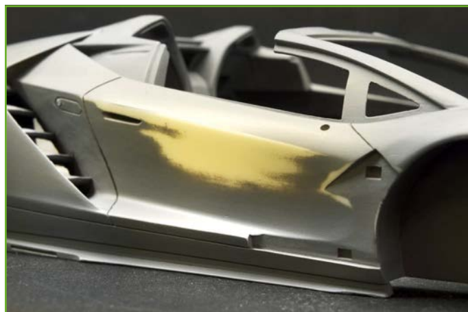
Body prepping process: sanding, filler, sanding, primer, sanding, primer, sanding and so on...
