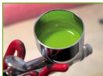
Once the paint was mixed thoroughly it was poured into the paint cup. With its fine pearl pigment, this colour looks amazing under bright light
