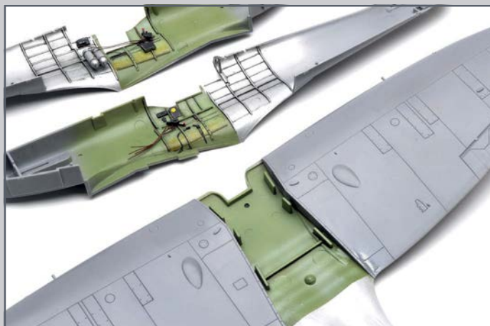
Lead wire was used to up-detail to the cockpit
