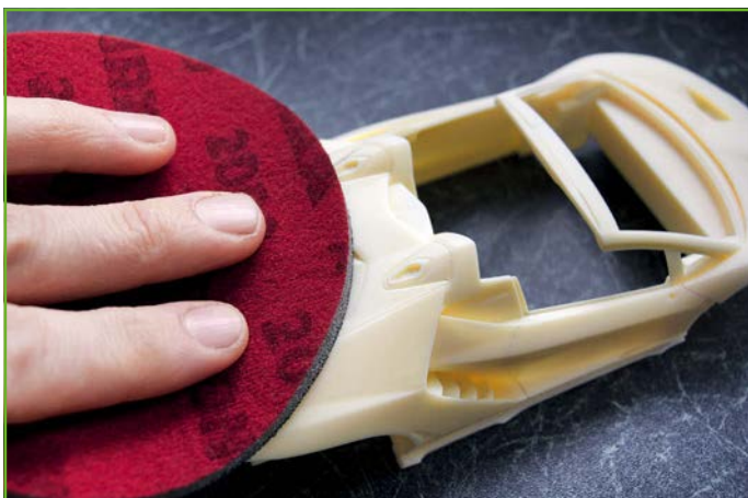
Body prep using a 2000-grit Abralon disc pad. These are superb sanding tools to use as they are soft which enables the user to follow panel contours safely whilst minimising the risk of pressure marks
