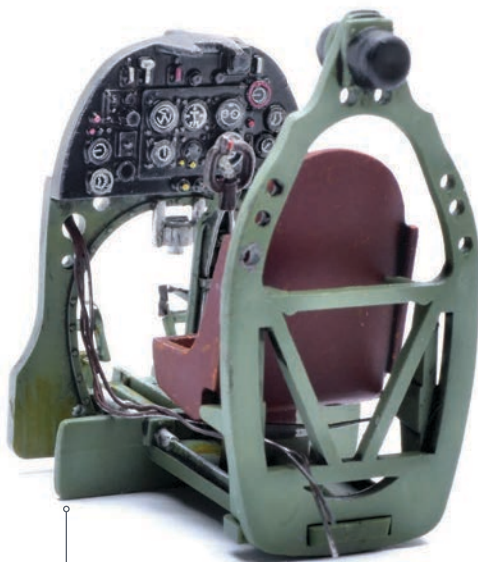
Holes were drilled out in the bulkhead and the author used dial decals from MDC on the instrument panel
